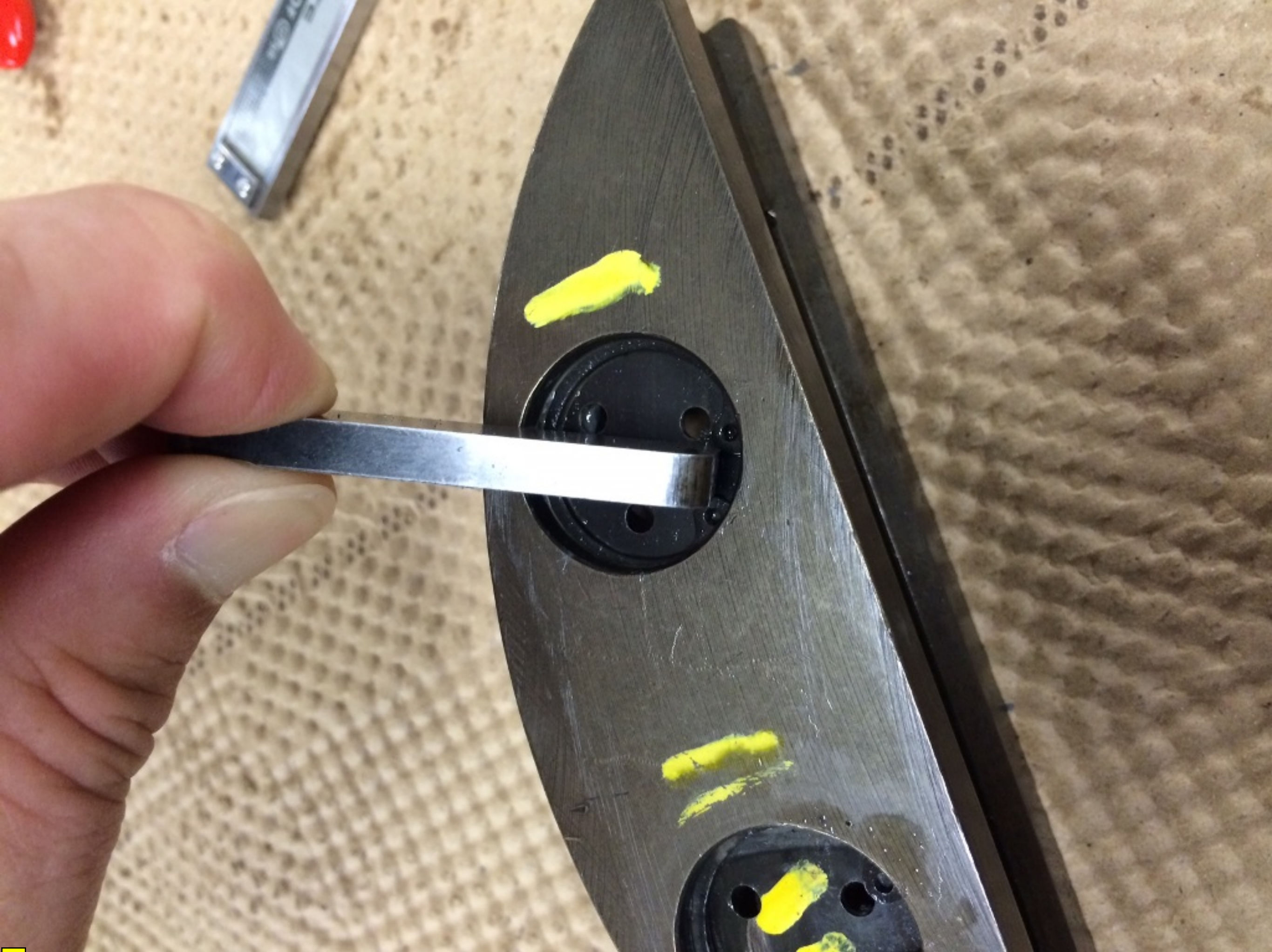
Photo 6 – Snap Rings on Rear Upper Counterweight When Gauge Did Not Fit
