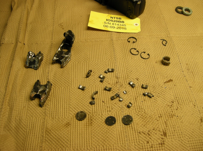
Photo 4 – Rear Lower Crankshaft Counterweight Snap Rings And Retaining
