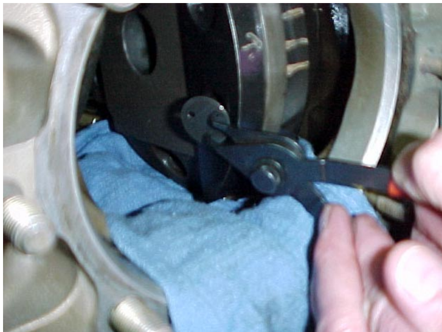
FIGURE 2. REMOVING COUNTERWEIGHT RETAINING PLATES
