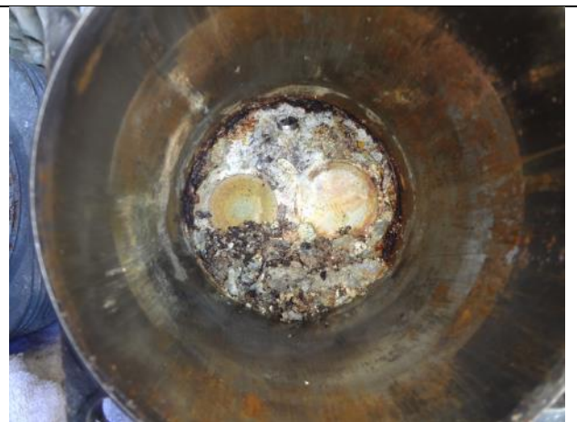
Photo 32: Cylinder No. 2 Barrel after Removal
