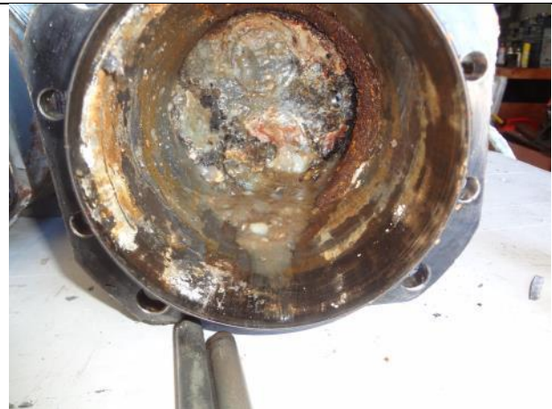
Photo 36: Cylinder No. 4 Barrel after Removal
