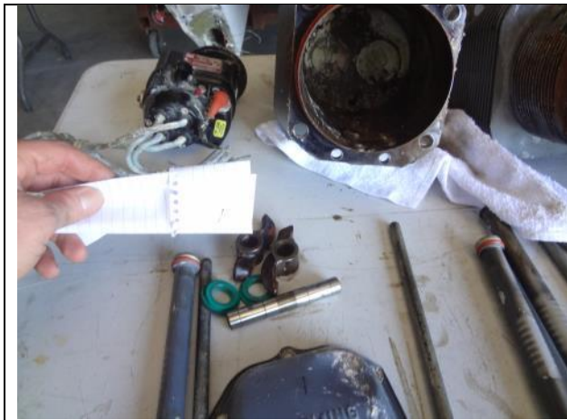
Photo 29: Cylinder No. 1 Components after Removal
