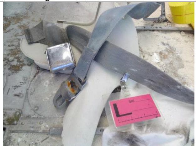
Photo 18: Left (Pilot) Seatbelt as Found - Post Recovery
