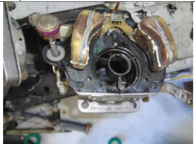
Photo 40: Carburetor Floats as Found after Removal
