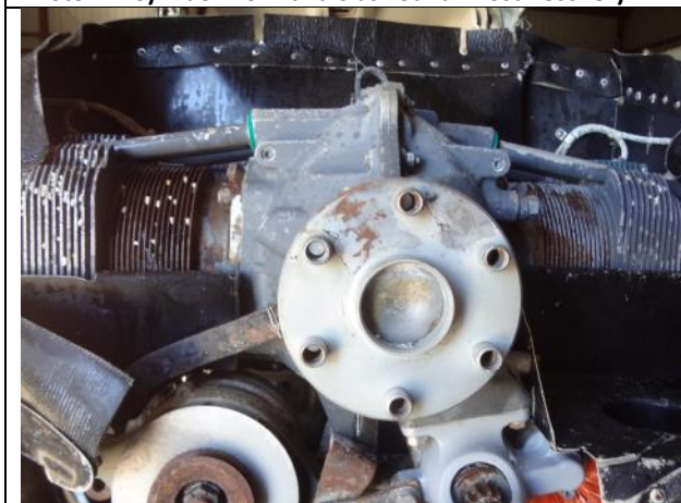
Photo 23: Propeller Flange as Found - Post Recovery
