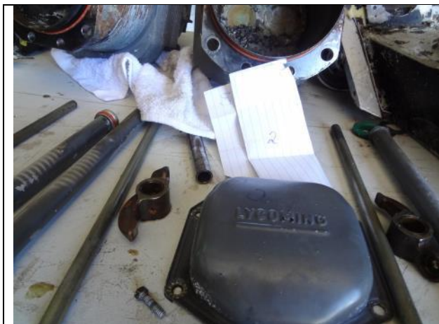
Photo 31: Cylinder No. 2 Components after Removal
