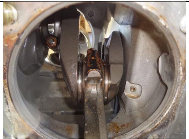
Photo 26: Crankshaft as Viewed Through Cylinder No. 4
