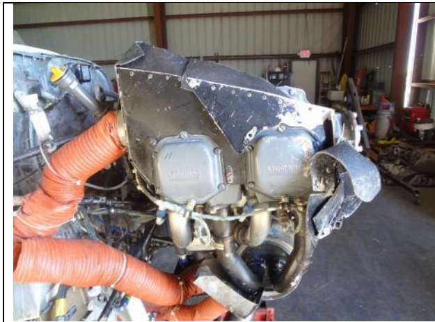
Photo 21: Cylinder No. 1 and 3 as Found - Post Recovery
