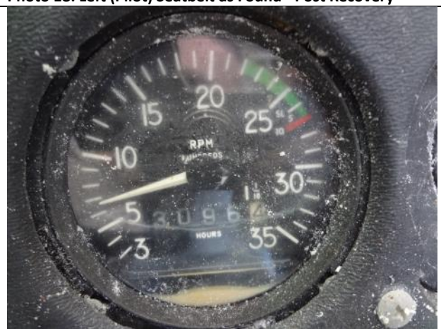
Photo 20: Tachometer as Found - 3096.4
