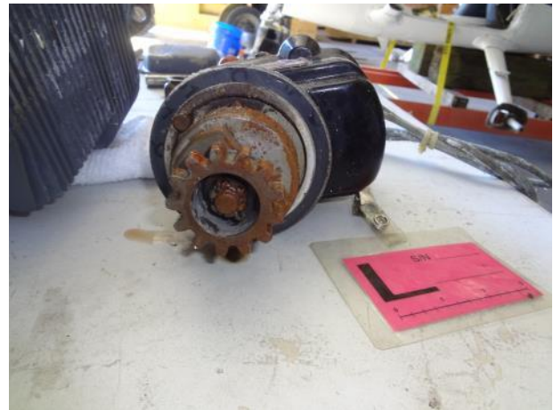
Photo 45: Left Magneto Gear with Corrosion
