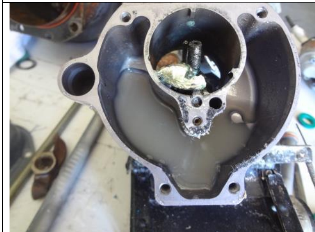
Photo 39: Fluid Found in Carburetor
