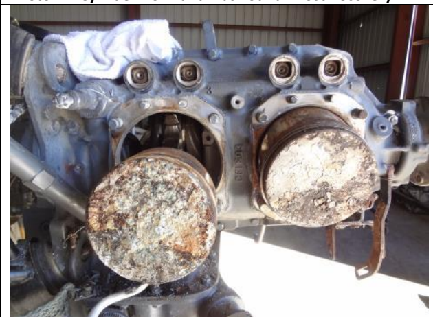
Photo 24: Cylinder No. 1 and 3 after Removal of Cylinder Barrel
