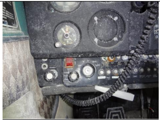
Photo 16: Magneto Switch in "OFF" Position
