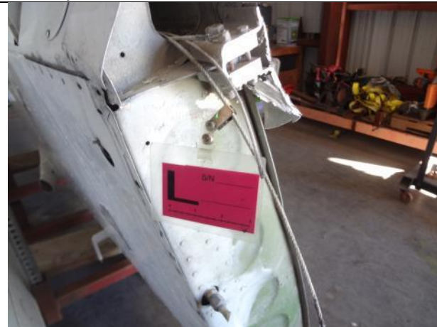
Photo 13: Left Wing Flight Control Cables with Recovery Cut Marks
