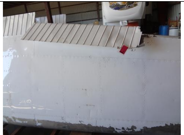
Photo 8: Remaining Portion of Left Aileron - Post Recovery
