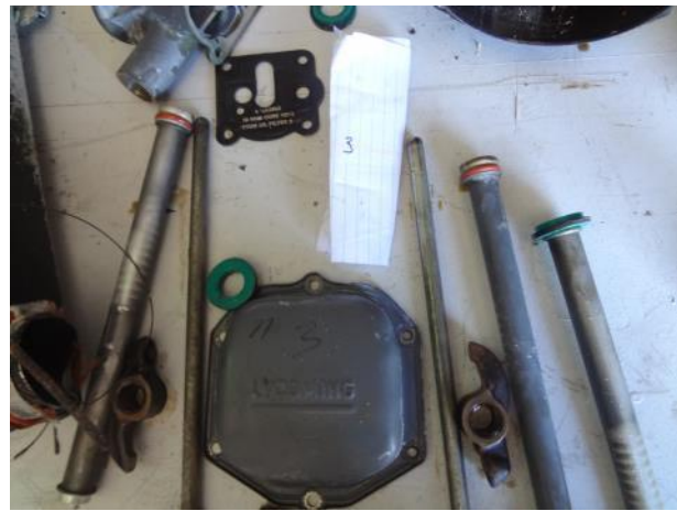
Photo 33: Cylinder No. 3 Components after Removal
