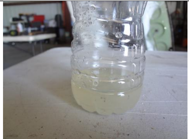
Photo 14: Fluid Extracted from Fuel Strainer
