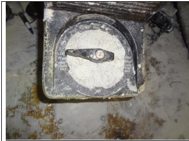
Photo 15: Fuel Selector Valve - Left Tank Selected
