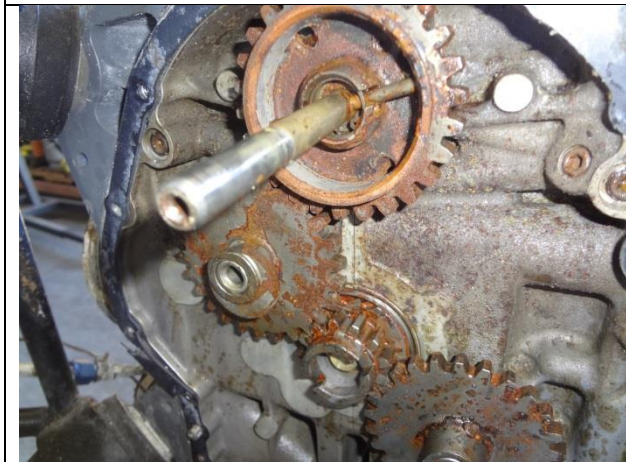
Photo 27: Gear in Accessory Gear Pad on Rear of Engine as Found
