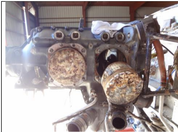
Photo 25: Cylinder Nos. 2 and 4 after Removal of Cylinder Barrel
