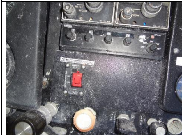
Photo 17: ELT Switch in "ON" Position as Found
