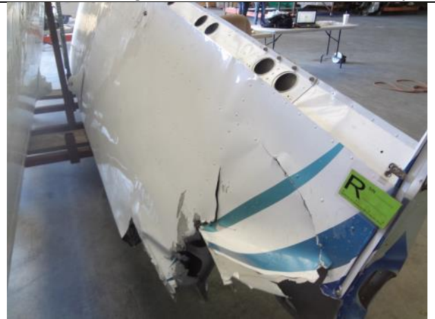
Photo 10: Bottom Outboard of Right Wing - Post Recovery
