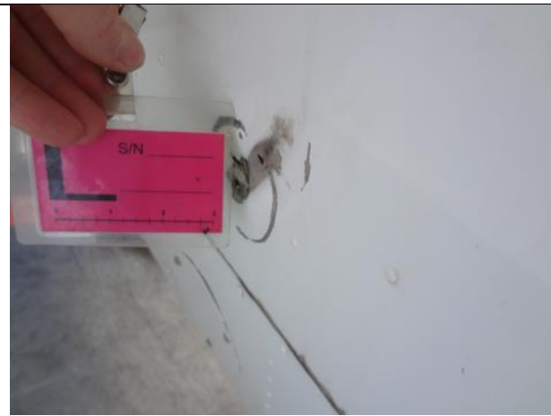
Photo 11: Burn Mark on Bottom Side of Left Wing – Post Recovery
