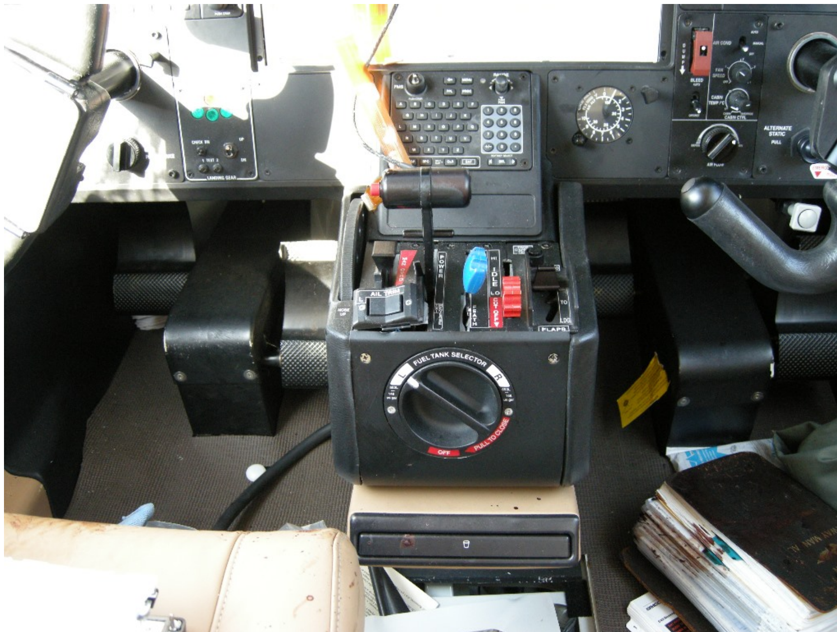
Photo 12 – Engine Controls and Fuel Tank Selector (NTSB Photo)
