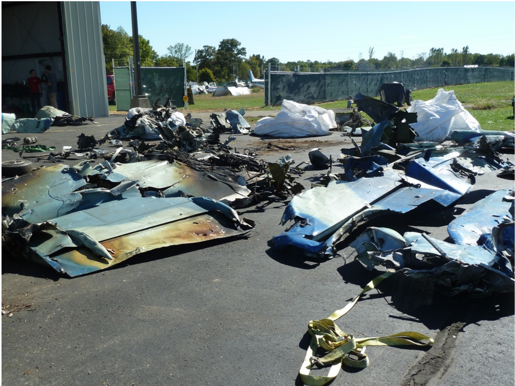
Photo 8 – Wreckage layout at recovery facility
