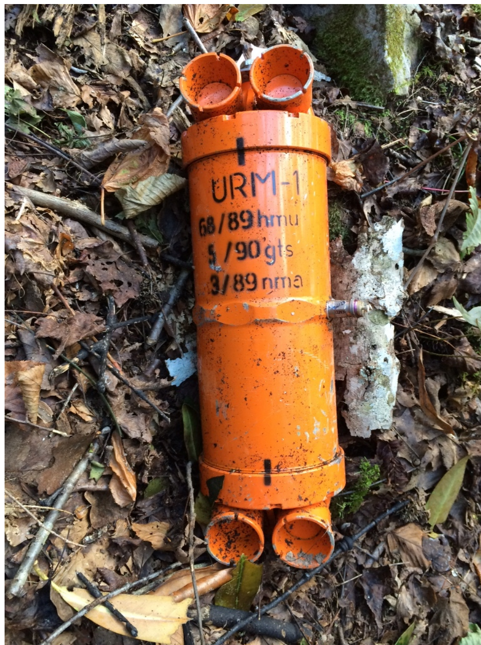
Photo 11 – Undischarged ejection seat rocket motor
