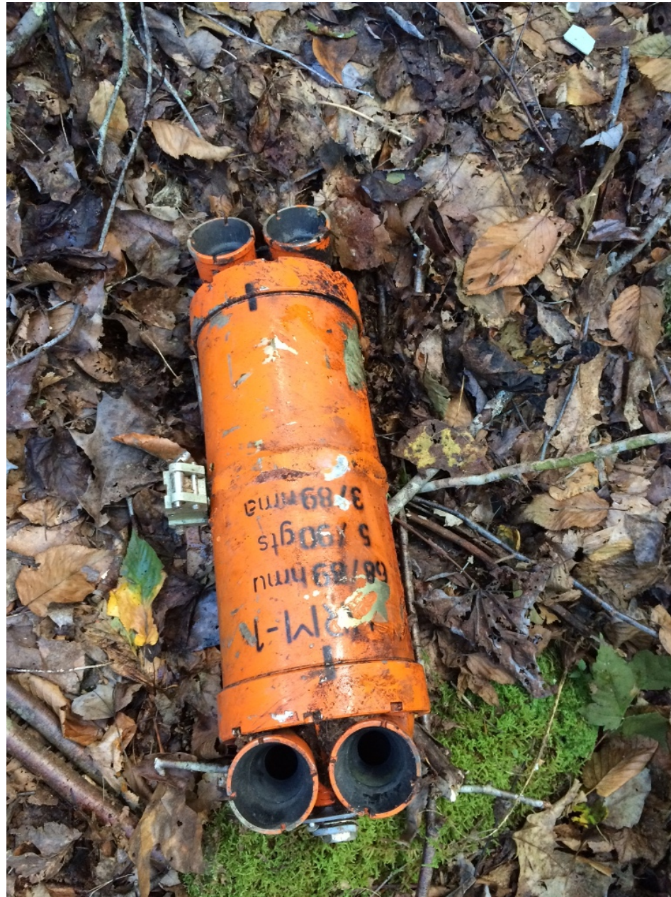
Photo 10 – Discharged ejection seat rocket motor
