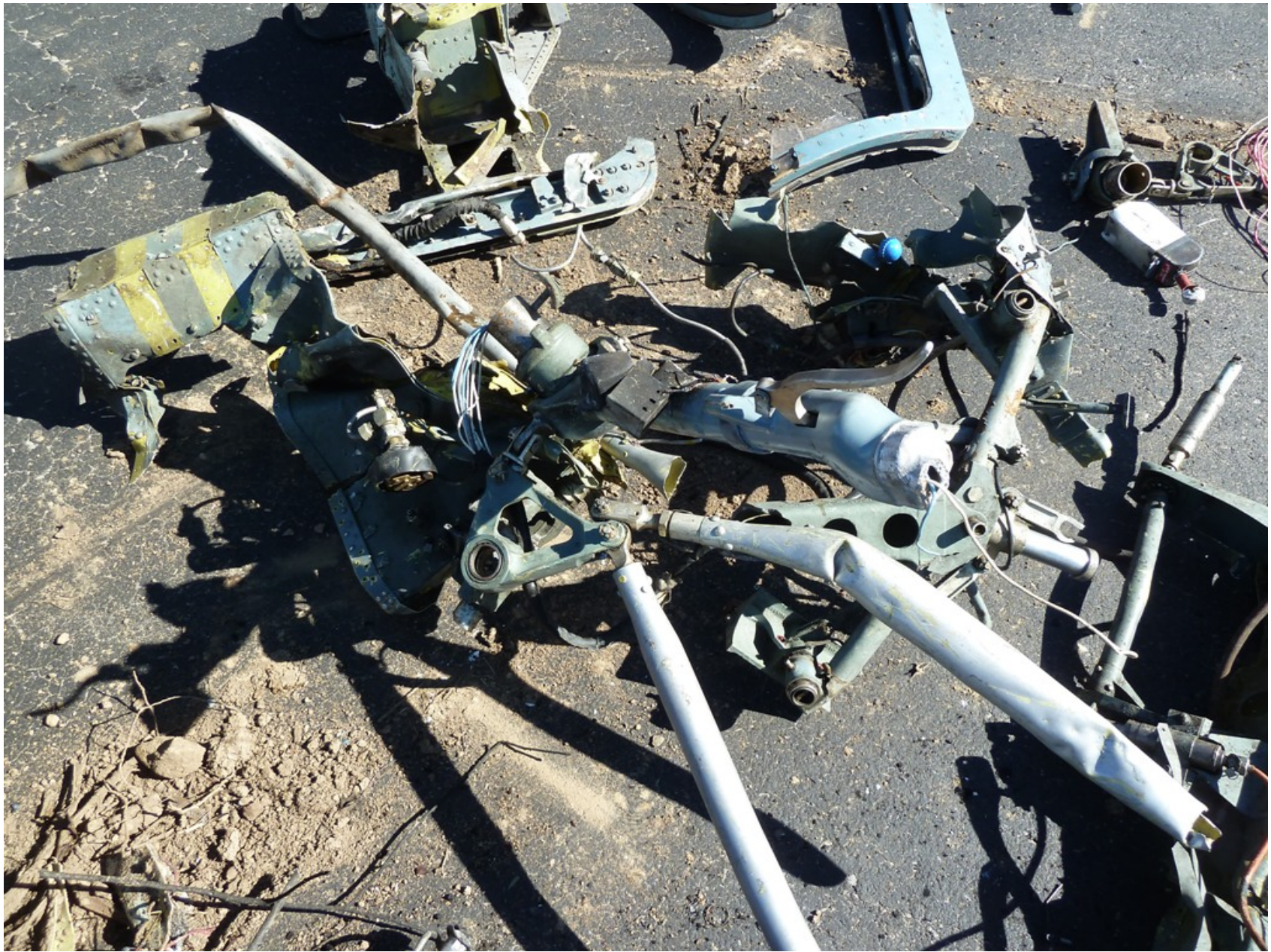
Photo 9 – Cockpit push-pull control tubes
