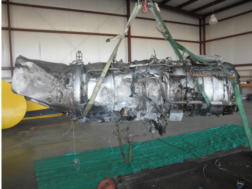
Photo No. 2: View of top of engine showing no uncontainments, case ruptures, or in-flight fire damage.
