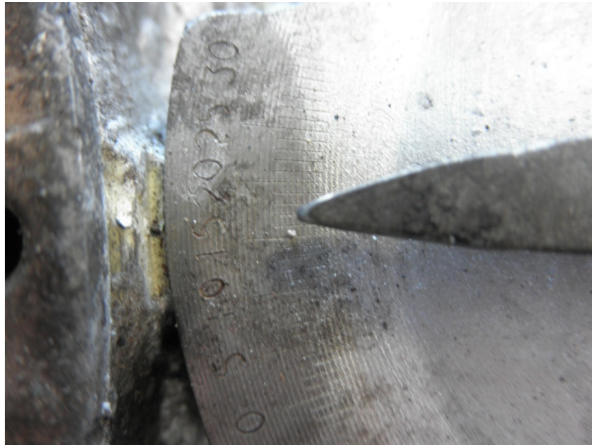
Photo No. 9: Close up view of variable stator vane indicator needle pointing to 17.
