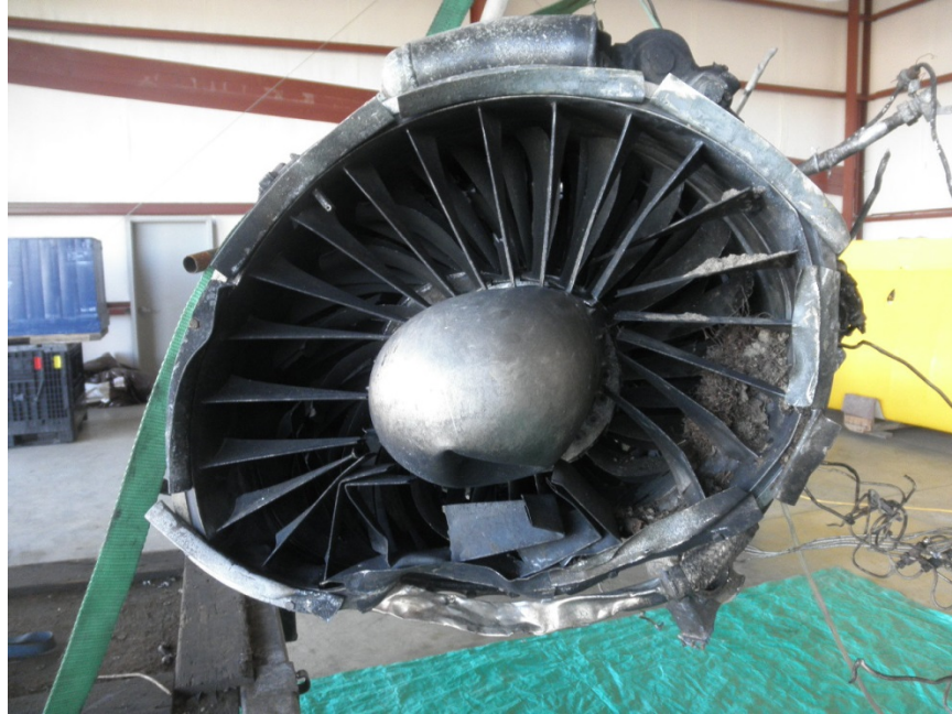
Photo No. 3: View of inlet case showing damage to the inlet guide vanes.
