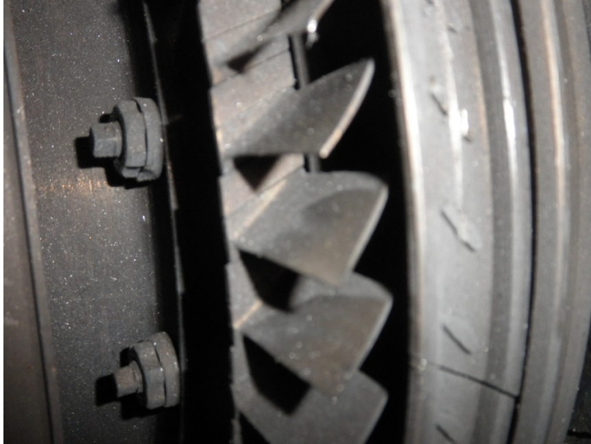
Photo No. 11: Close up of high pressure compressor 8th stage blades showing no damage.
