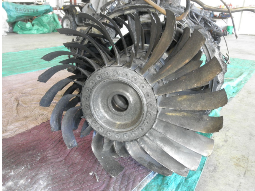
Photo No. 4: View of fan rotor showing fan blades bent opposite the direction of rotation.
