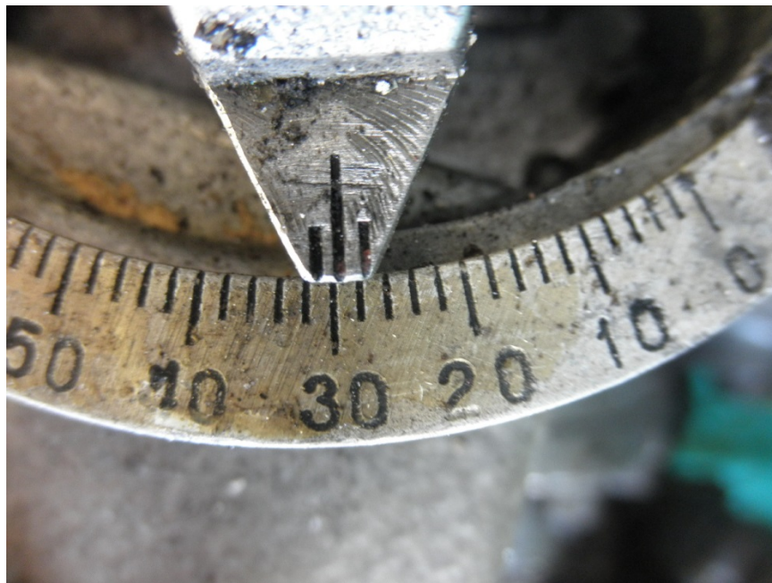
Photo No. 13: Close up view of fuel control throttle protractor indicator pointing to 30.
