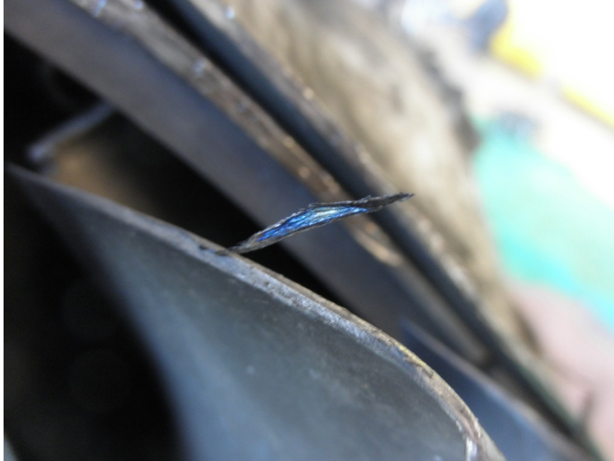
Photo No. 6: Close up of a 1st stage fan blade tip that had circumferential rub mark and tab of metal with heat discoloration.
