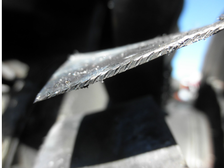
Photo No. 7: Close up of 3rd stage fan blade tip showing marks from shroud rub strip.
