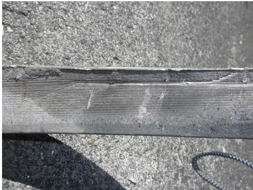
Photo No. 8: Close up of 3rd stage fan rub strip showing imprints of blade tips.
