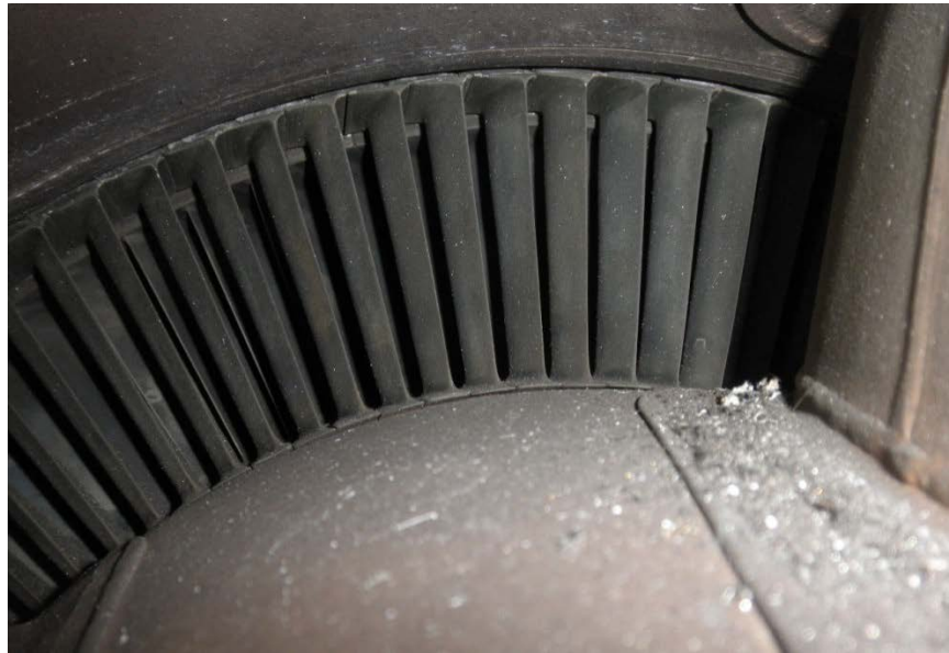
Photo No. 12: View of low pressure turbine 2nd stage blades showing no damage to the airfoils.
