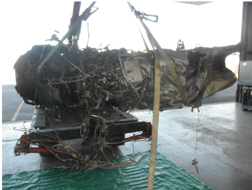
Photo No. 1: View of bottom of engine showing no uncontainments, case ruptures, or in-flight fire damage.
