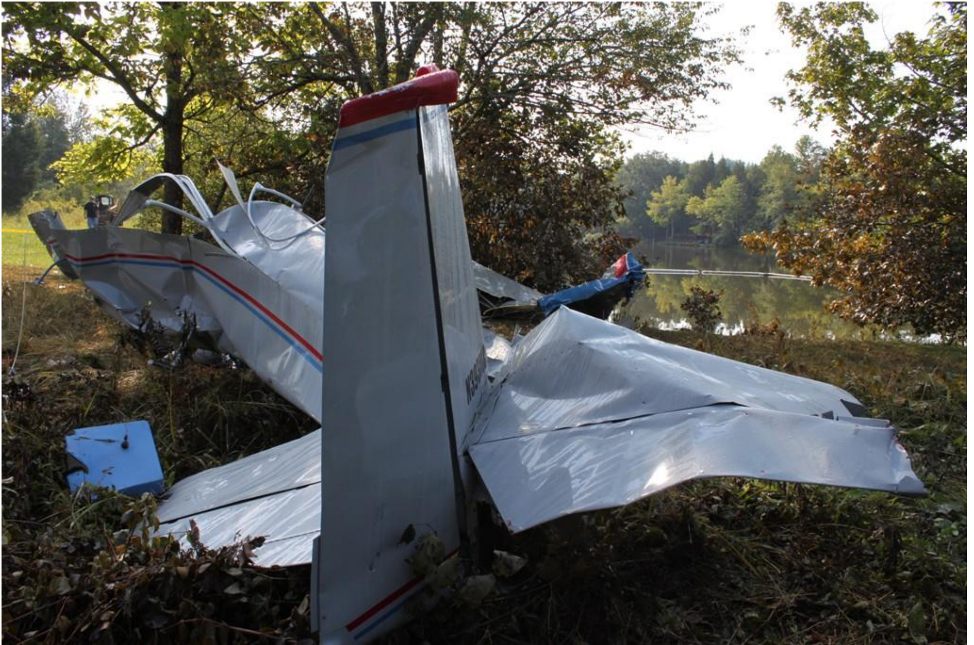
Photo 8 - NTSB Digital Photograph. Rear View of the Empennage.
