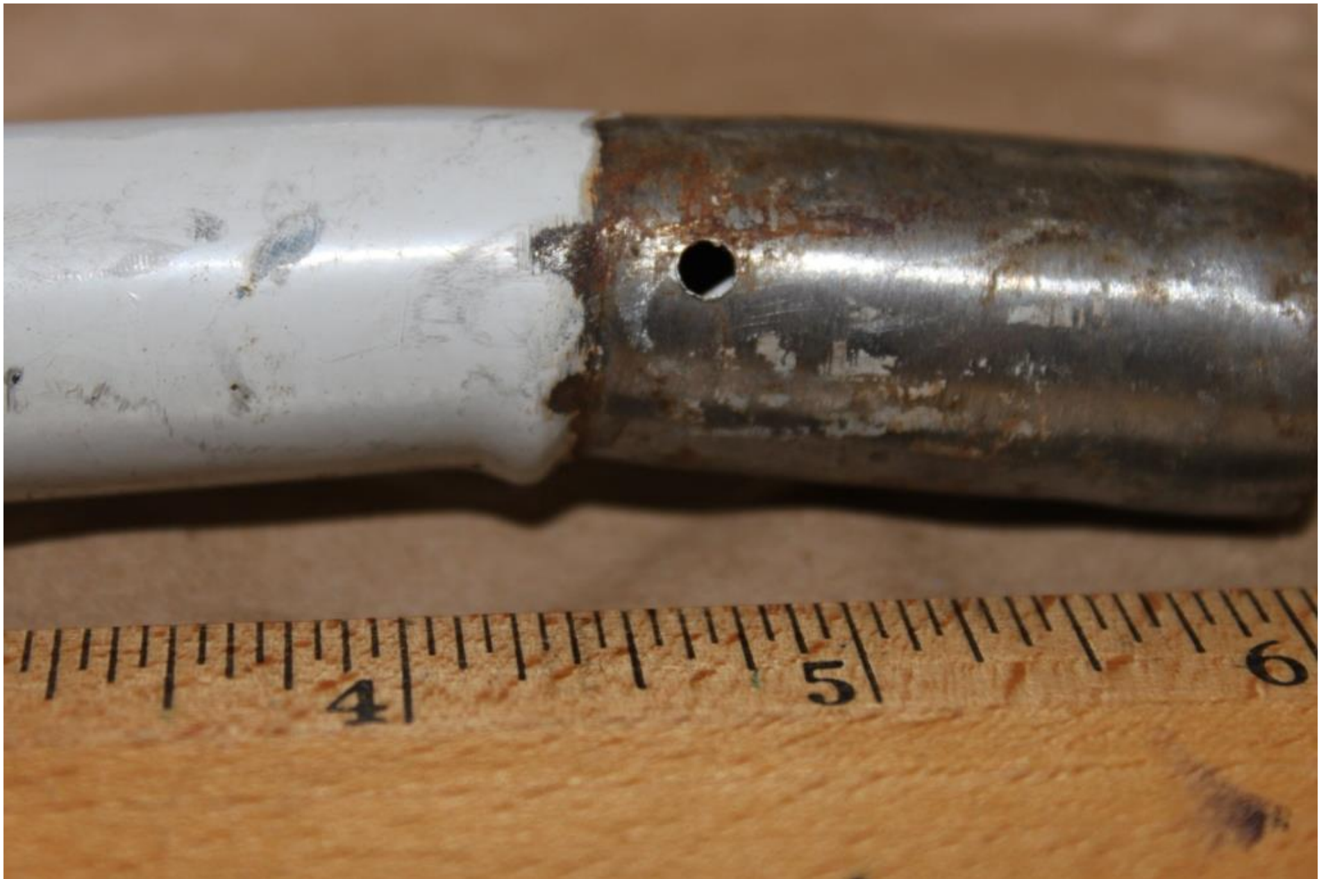
Photo 13 - NTSB Digital Photograph. Close-Up view of the Left Side of the Rear Seat Control Stick. Note the Bulging on the Forward Portion of the Control Stick.
