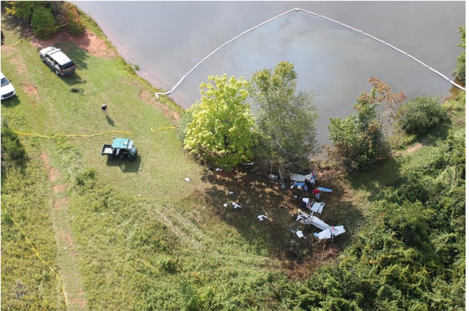
Photo 2 - NTSB Digital Photograph. Close-Up Aerial View of the Accident Site. Note the fuel sheen on the water.
