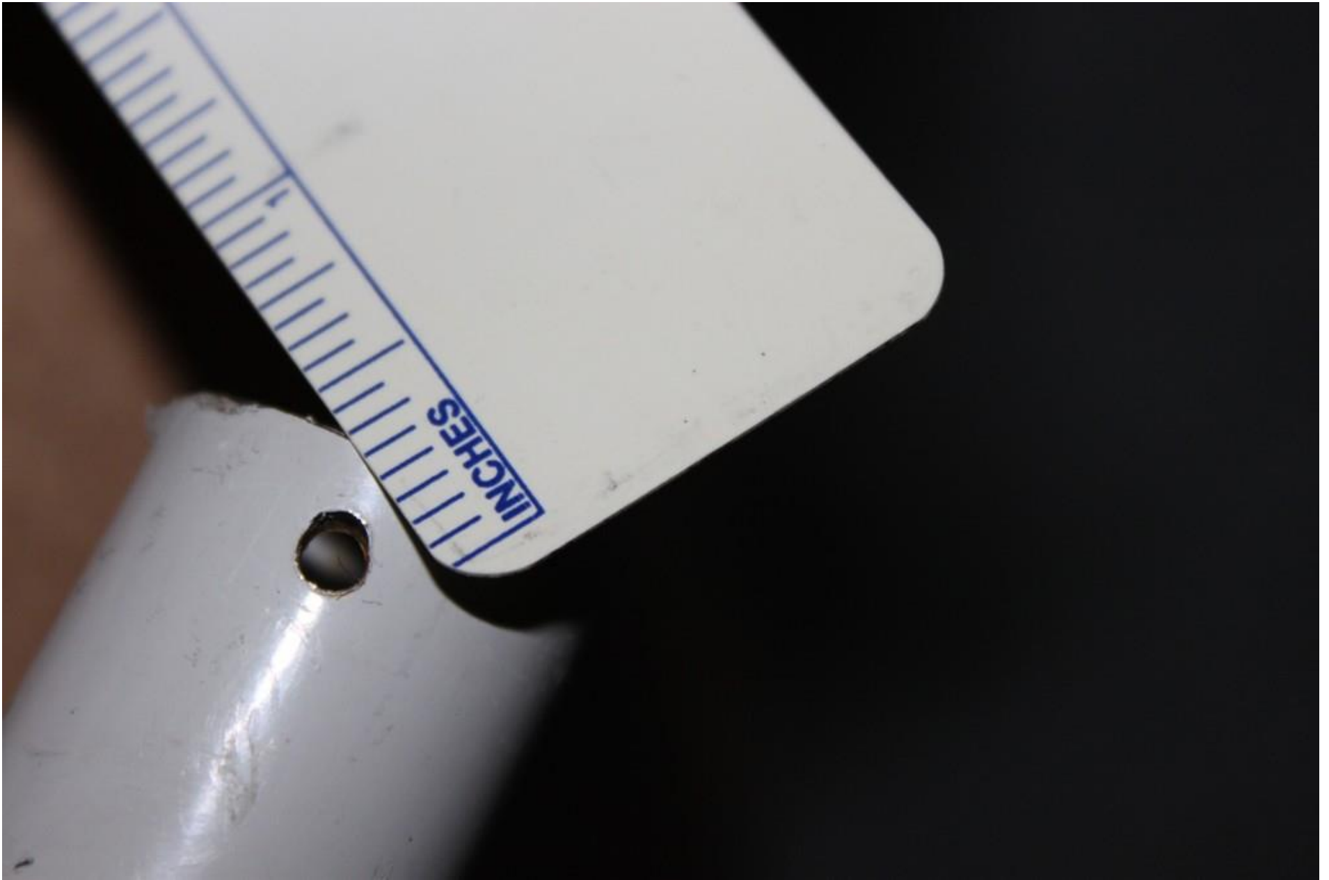
Photo 14 - NTSB Digital Photograph. Close-Up view of the Left Side of the Rear Seat Control Stick Base. Note the Deformation of the Upper Portion of the Hole.
