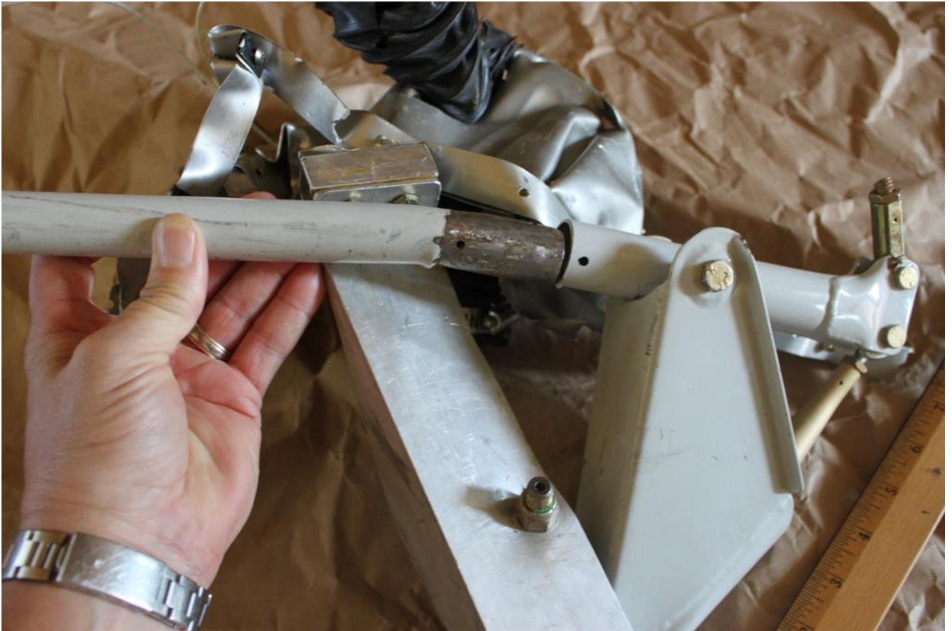
Photo 12 - NTSB Digital Photograph. Left Side View of the Rear Seat Control Stick and Control Stick Base. Note the bulging on the Forward Portion of the Control Stick.
