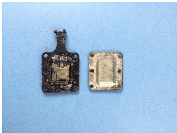
Figure 6. DFC-90 memory module open and microSD card shown seated.
