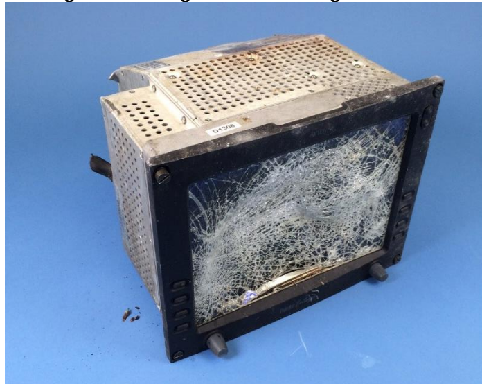
Figure 1. Damaged exterior of flight recorder.
