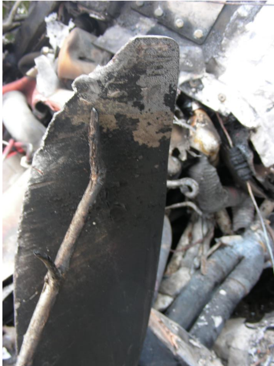
Photo 3 – View of Damaged Propeller Blade.
