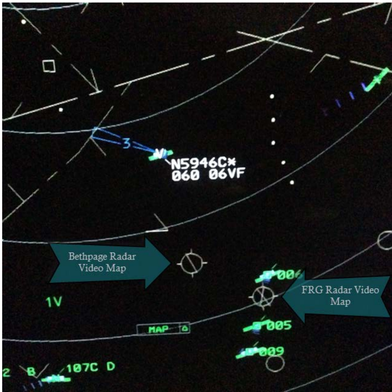
Figure 5 – Radar presentation of N5946C as seen by the N90 LGA area controller. The RVM for Bethpage and FRG are indicated by green arrows.
