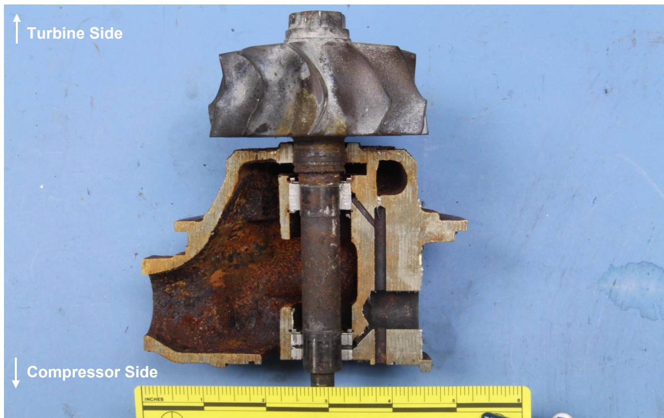
Figure 6 – The sectioned center housing of the turbocharger, showing the location of the turbine wheel along the internal bearings.
