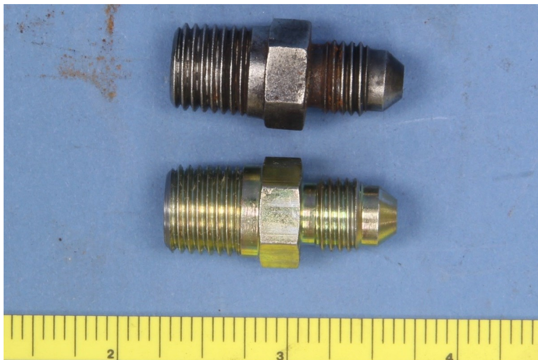
Figure 13 – The accident oil check valve (above) and an exemplar (below).
