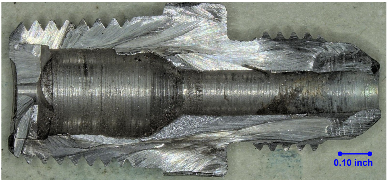
Figure 19 – One of the exemplar check valves, after sectioning.
