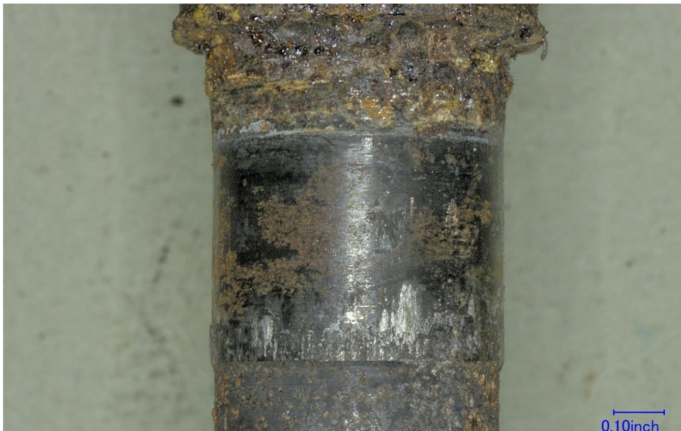
Figure 12 – The turbine side of the turbine wheel shaft, which mated against the turbine side bearing in the center turbine housing. The shaft shows rotational and longitudinal wear marks.
