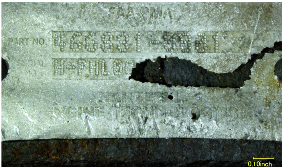
Figure 2 – The label plate on the upper side of the center turbocharger housing.
