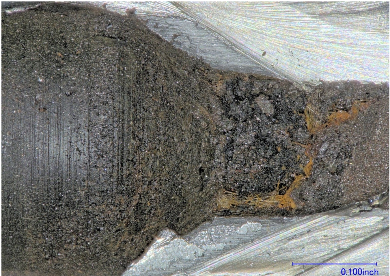
Figure 18 – The mating side of the sectioned accident check valve, showing contamination in the channel.
