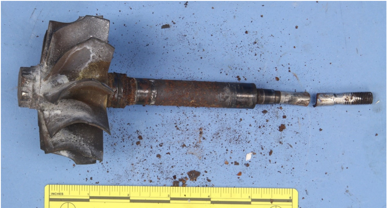
Figure 10 – The turbine wheel assembly, showing both fractured portions of the shaft segment from the compressor side.
