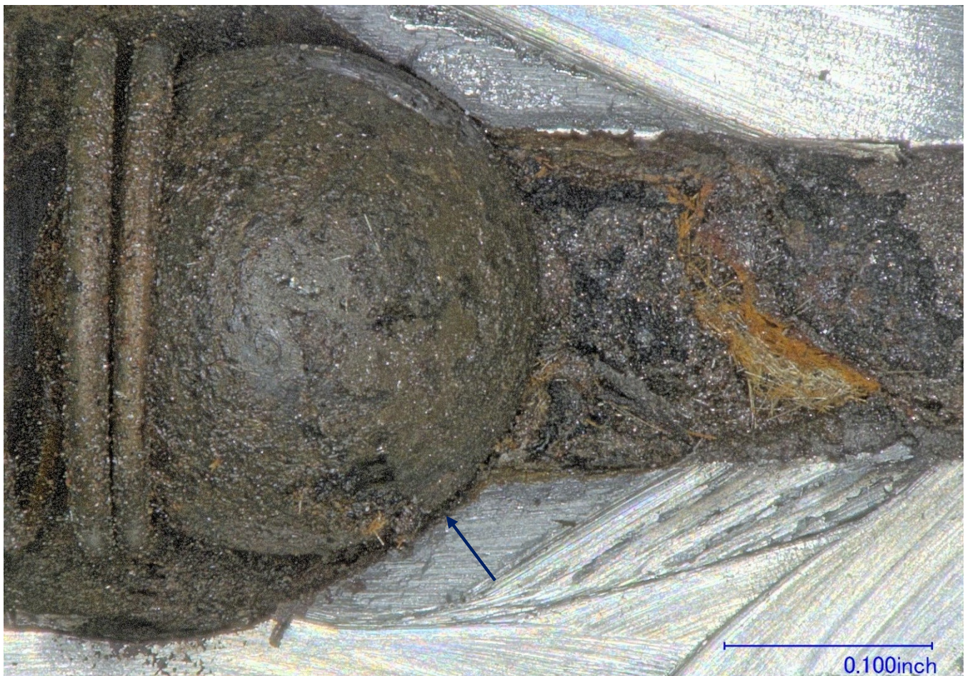
Figure 16 – Closer view of the ball valve of the accident check valve, showing a gap (arrow) with foreign material.
