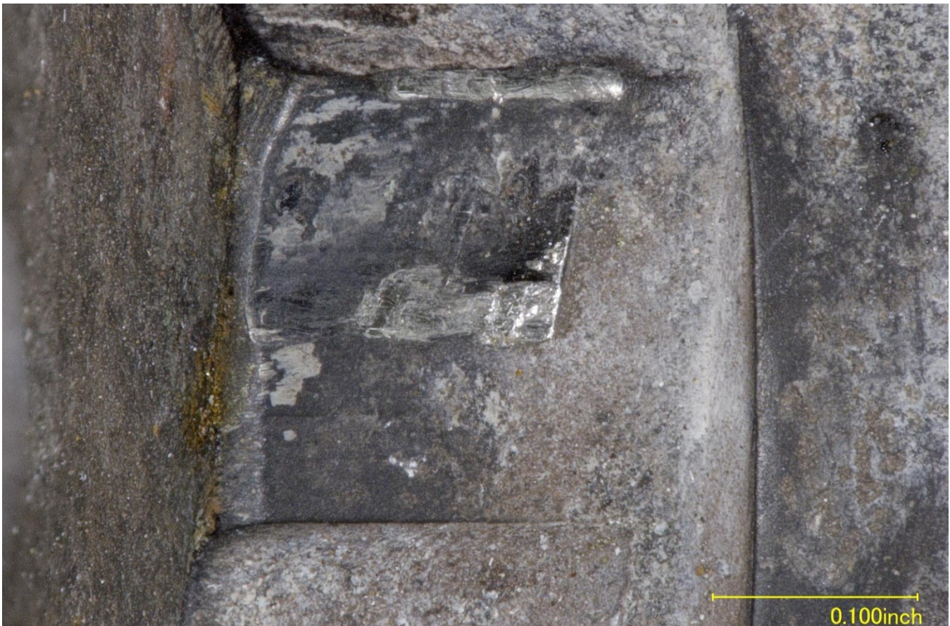
Figure 11 – Witness marks on the turbine side of the wheel.
