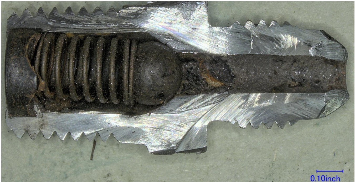
Figure 15 – The accident check valve, after sectioning the inner channel, with the spring and ball still present.
