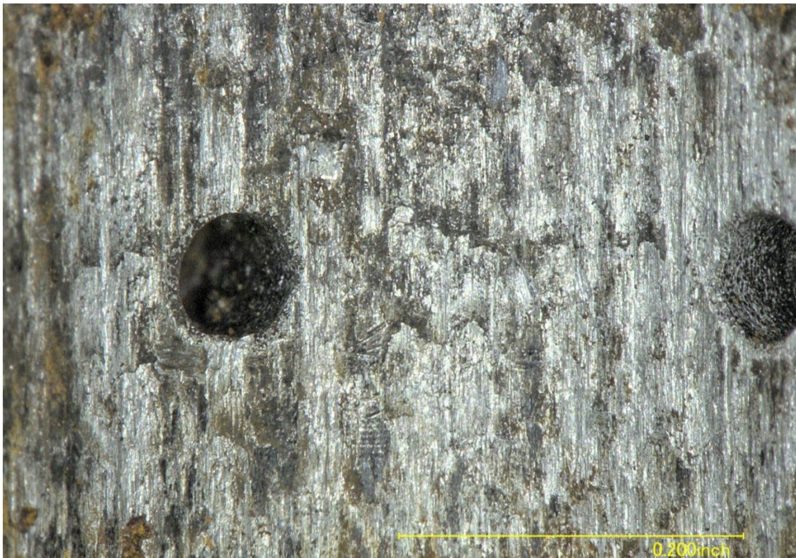
Figure 8 – A closer view of the sectioned turbine side bearing inside the center turbo housing.
