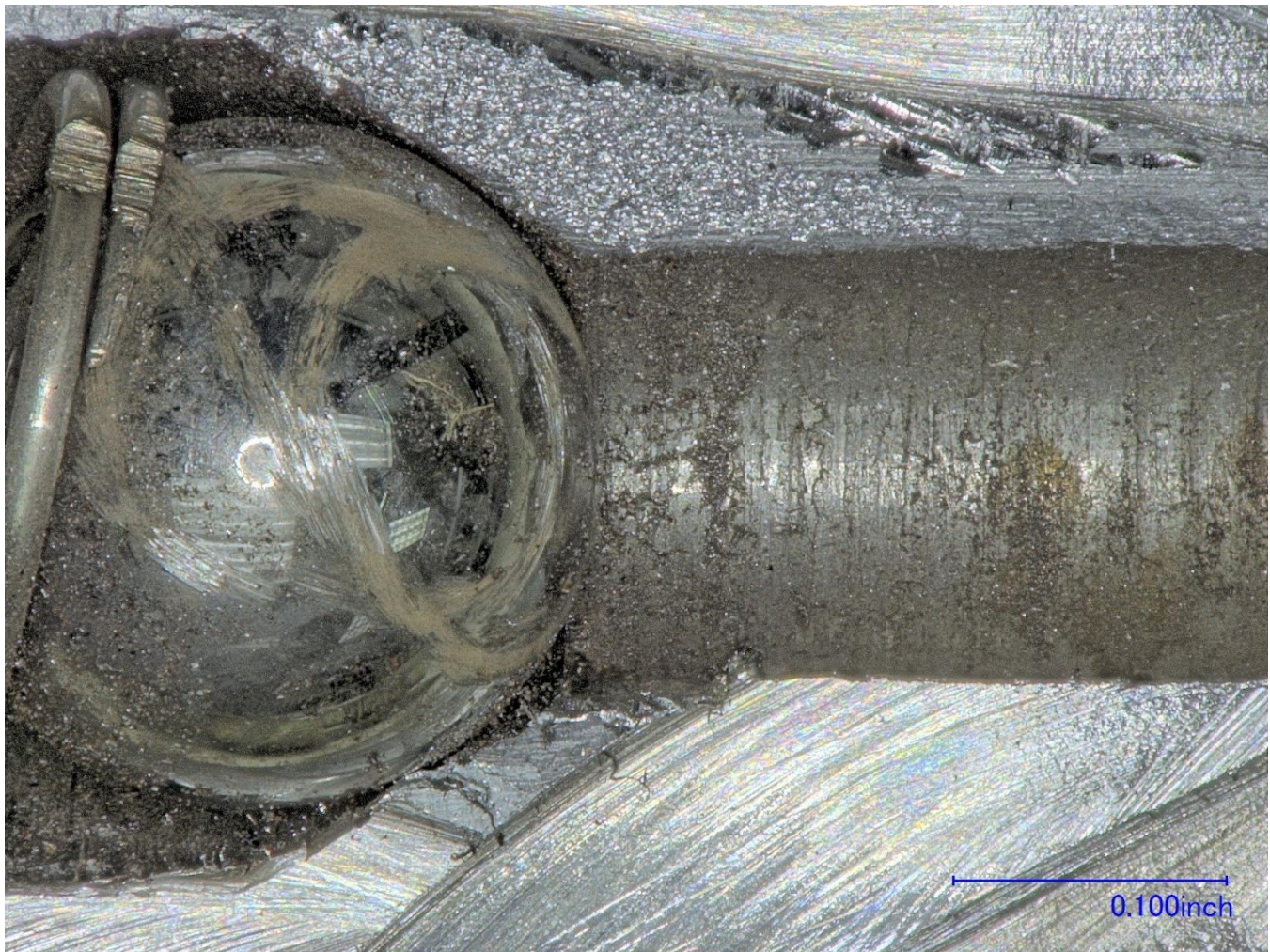
Figure 21 – The mating side of the sectioned check valve from Figure 19, showing the position of the ball and spring.
