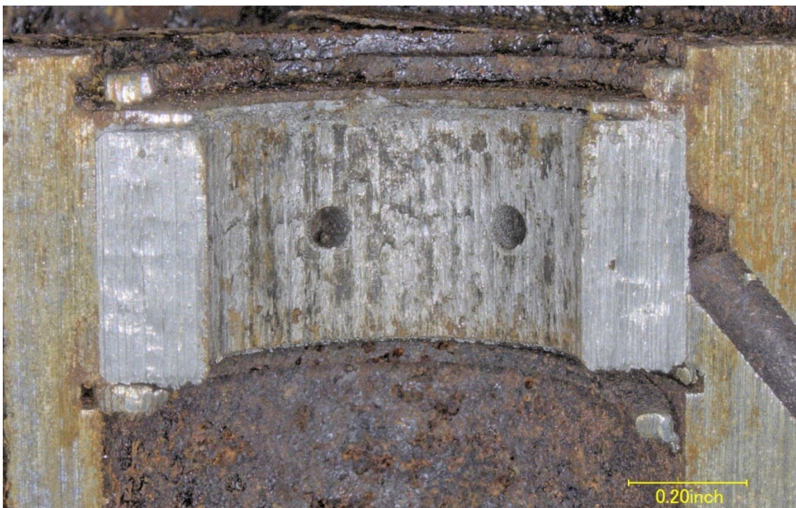
Figure 7 – A closer view of the sectioned turbine side bearing inside the center turbo housing.
