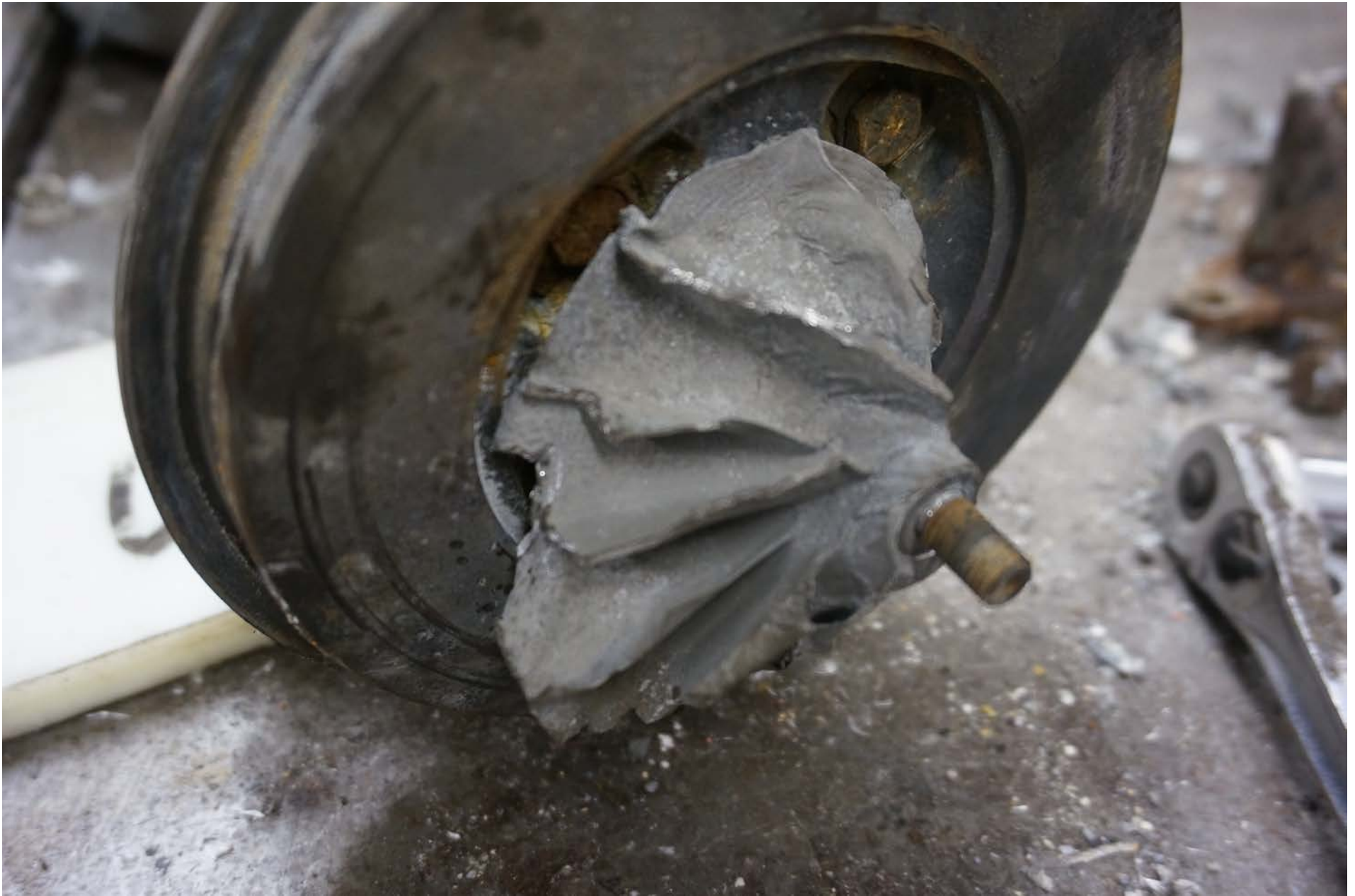
Photo 16 – Compressor Wheel after Removal of Remains of Compressor Housing
