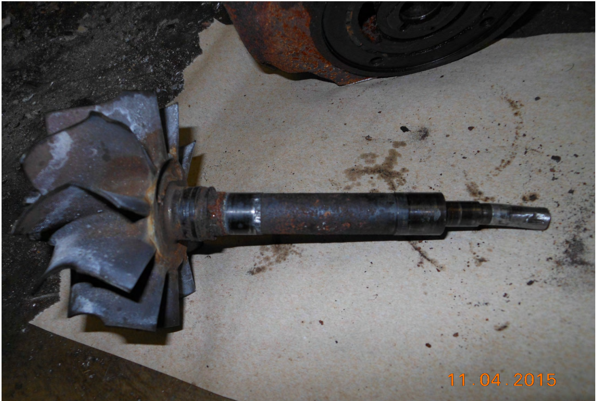
Photo 19 – Turbine Wheel Assembly with Piston Ring – Courtesy of Hartzell Engine Technologies
