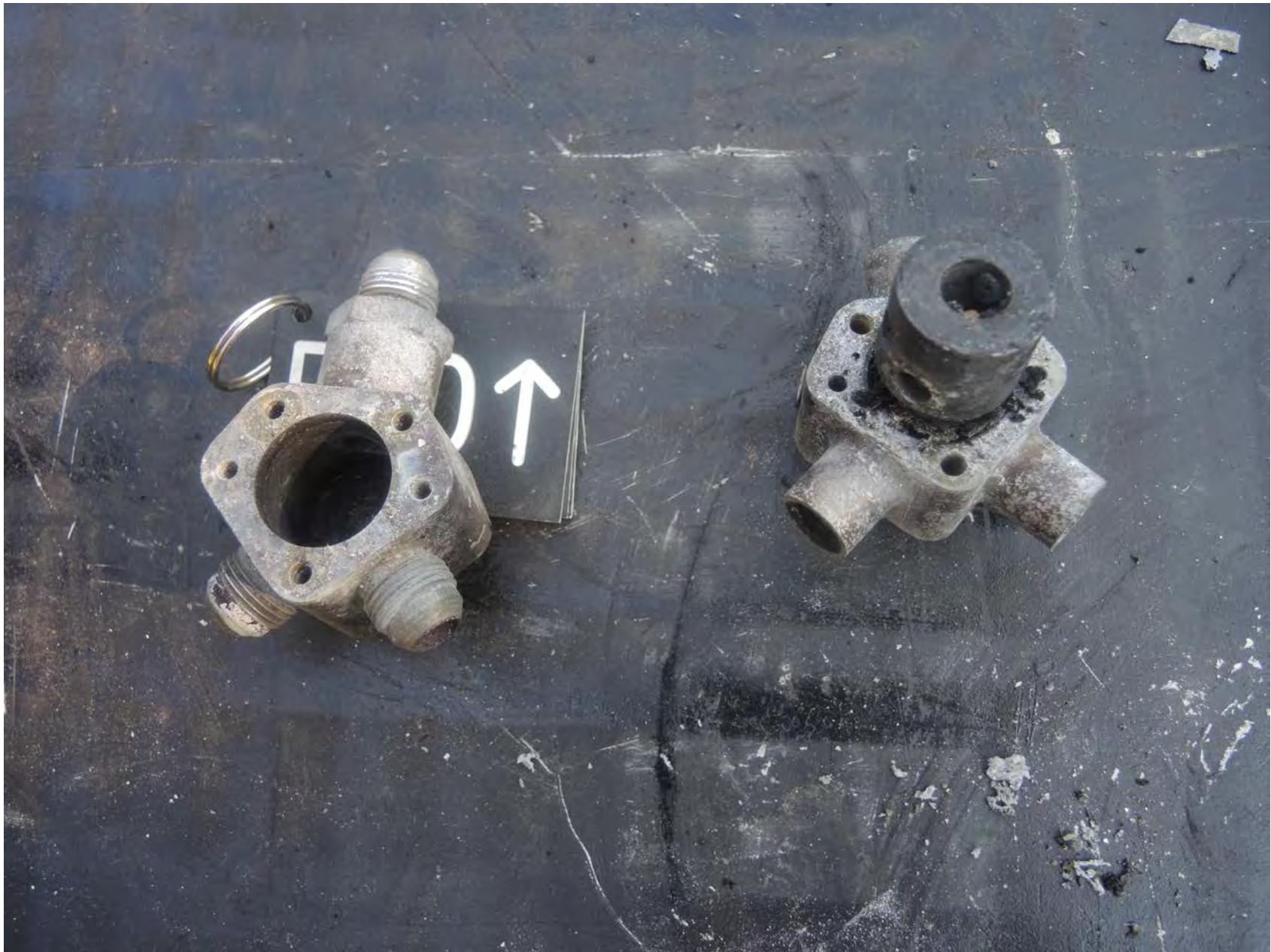
Photo 10 – Fuel Selector Valve – Courtesy of Textron Aviation
