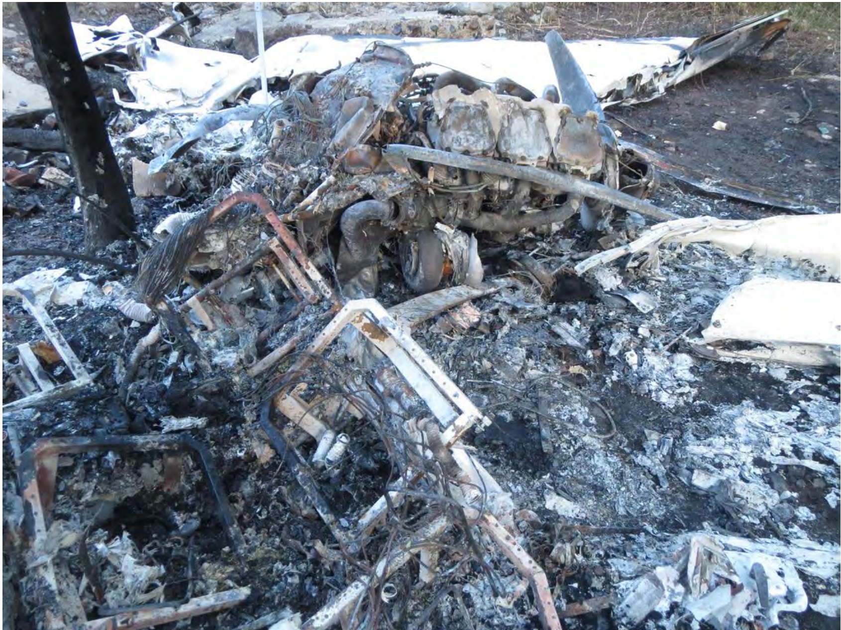
Photo 5 – Right Side of Engine Showing Turbocharging System
