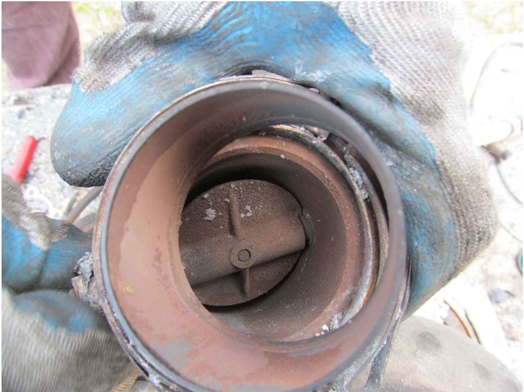
Photo 14 – Exhaust Bypass Valve (Wastegate) – Courtesy of Lycoming Engines
