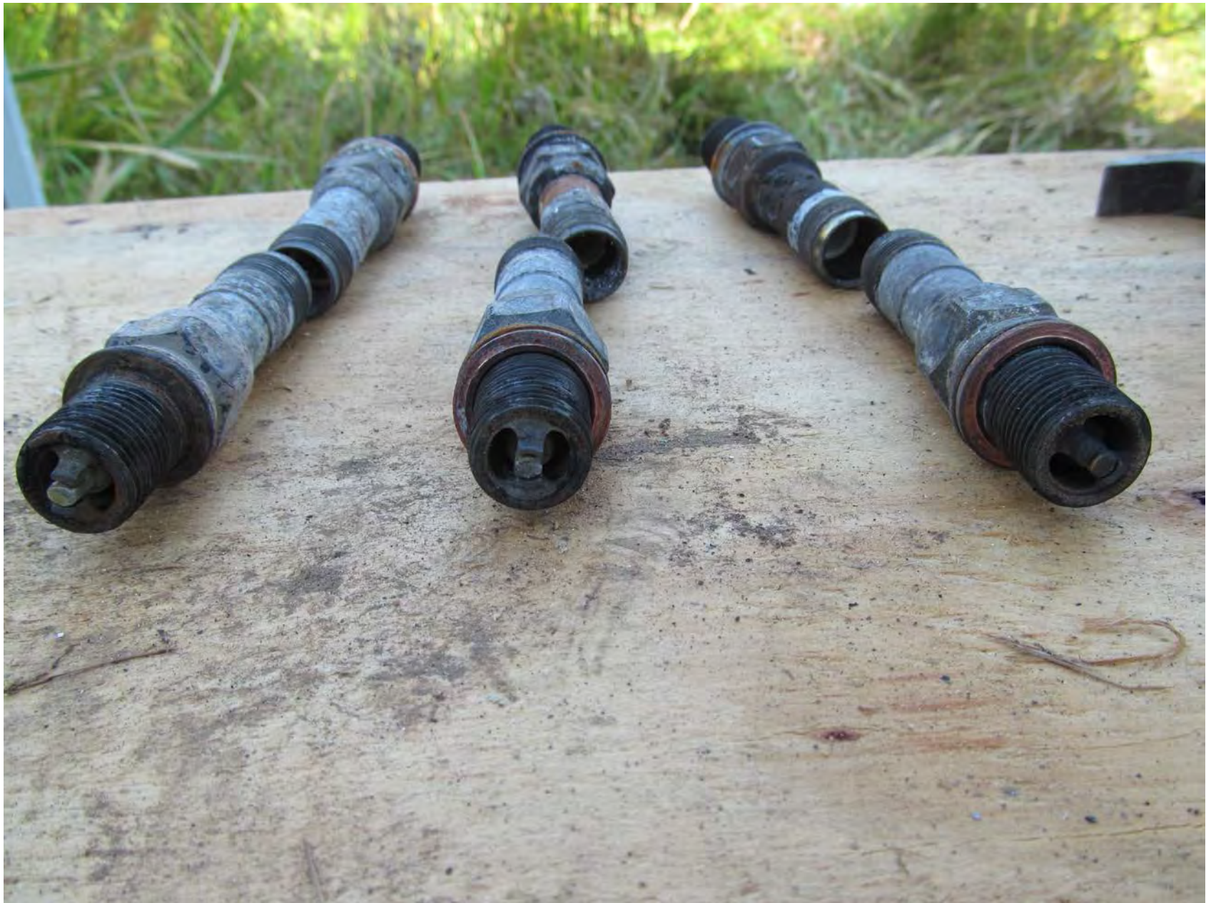
Photo 13 – Close Up of Upper Spark Plugs (No.2, No.4, and No.6) – Courtesy of Lycoming Engines
