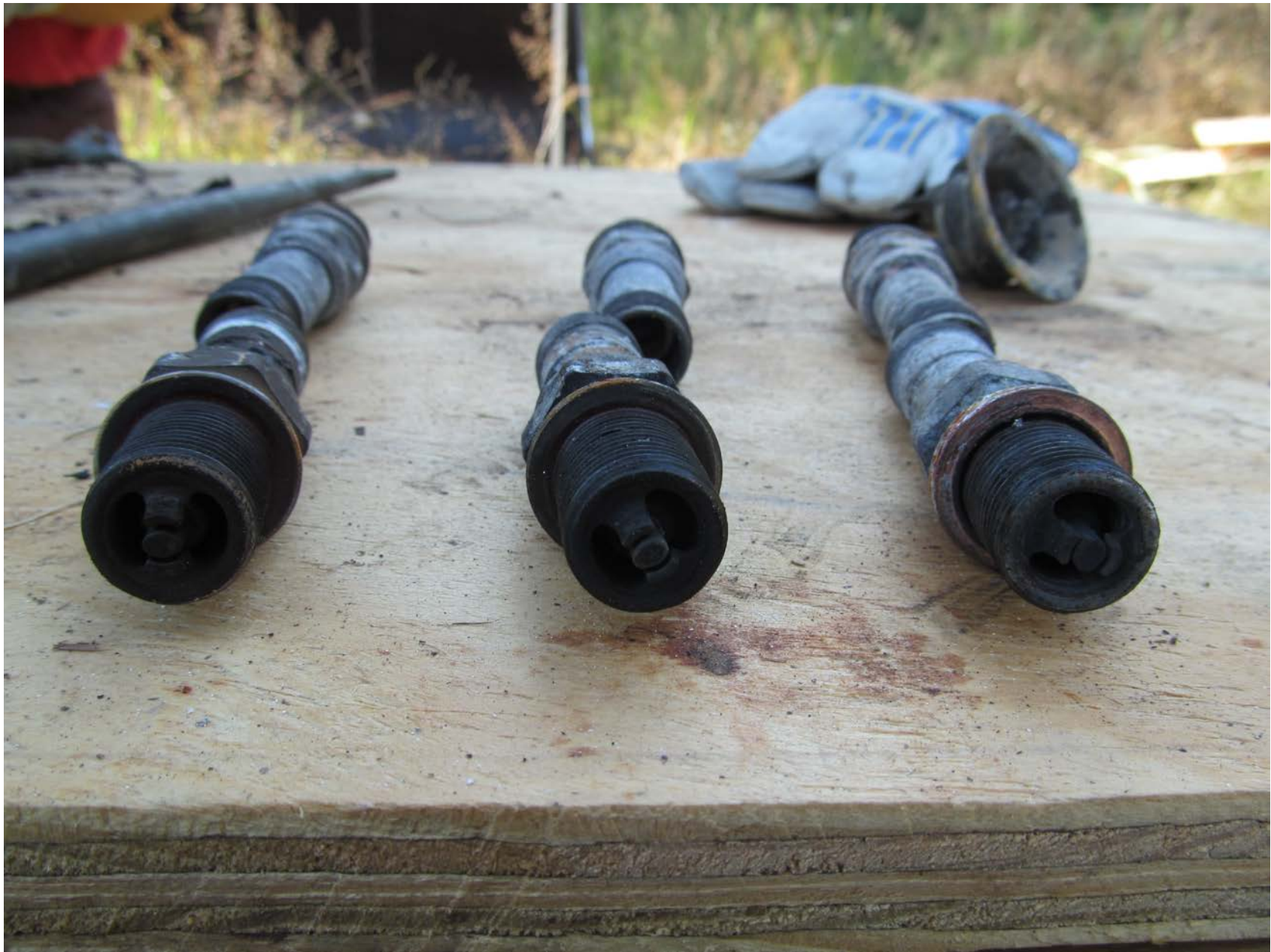
Photo 12 – Close Up of Upper Spark Plugs (No.1, No.3, and No.5) - Courtesy of Lycoming Engines
