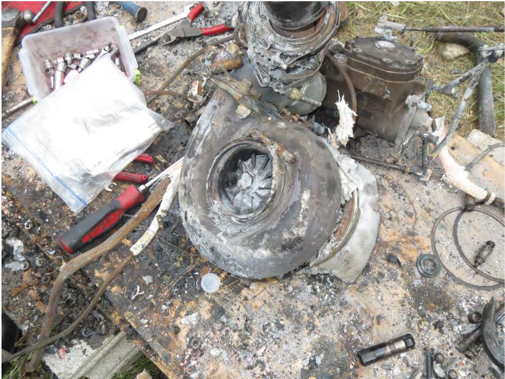
Photo 6 – Turbocharger (Turbine Wheel and Turbine Wheel Housing)
