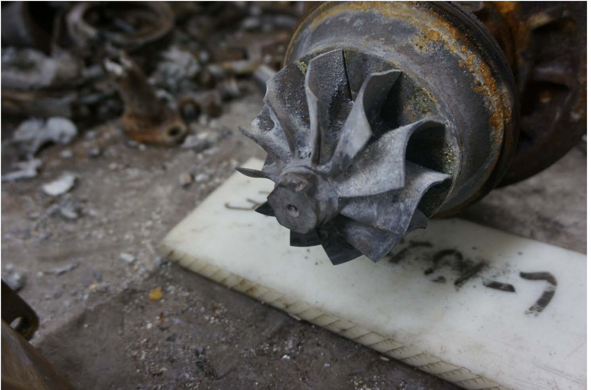
Photo 15 – Turbine Wheel After Removal from Turbine Housing
