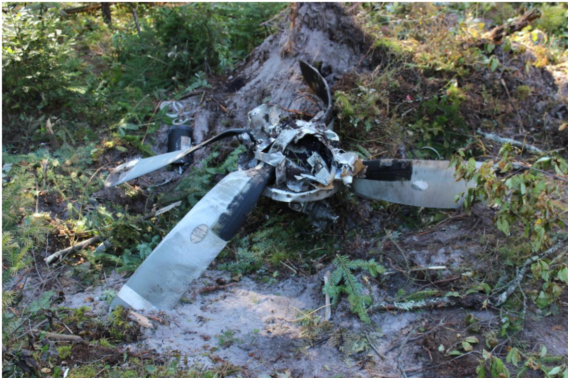
Photo No. 3, View of the propeller and a section of the front reduction gearbox
