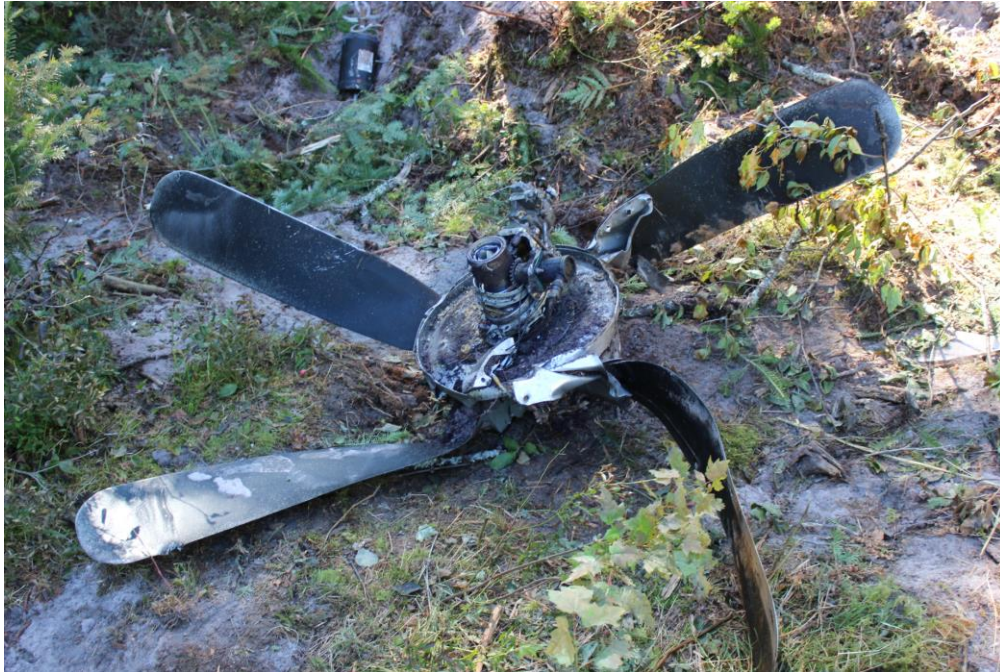
Photo No. 8, A view of the of the reduction gearbox components attached to the propeller
