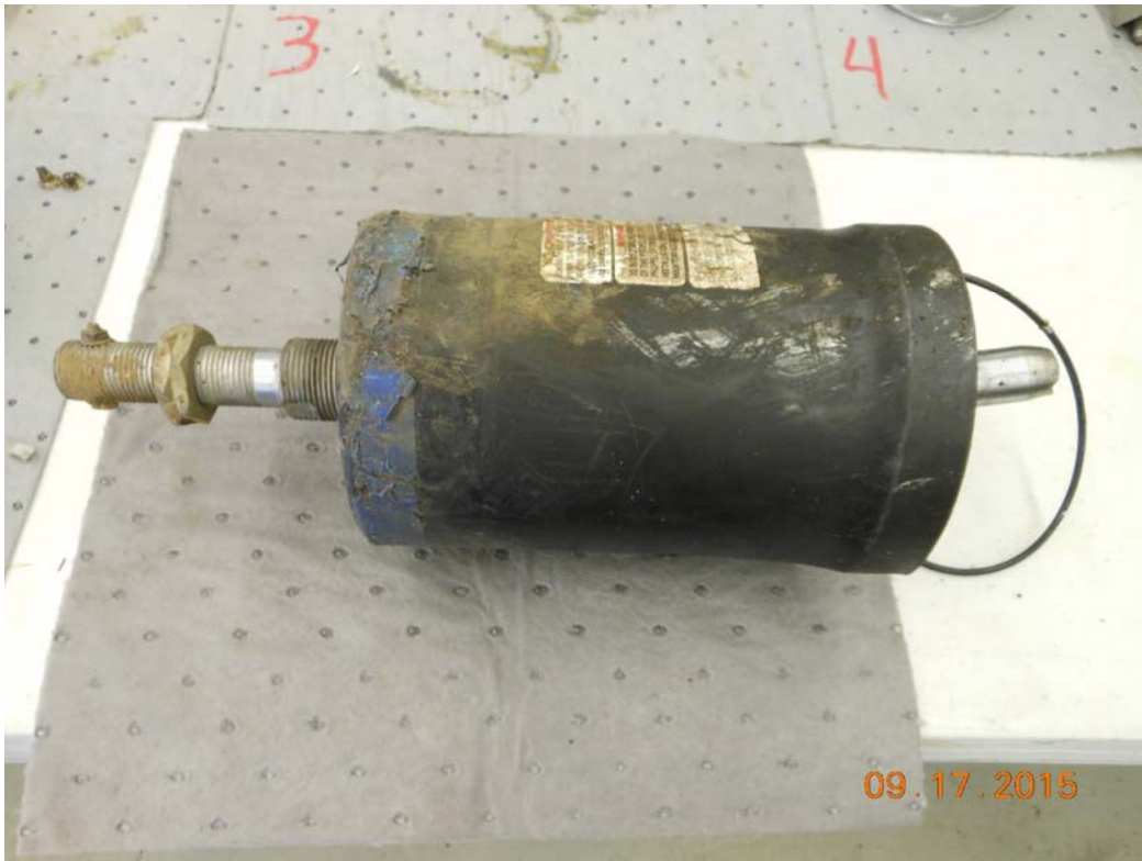
Photo #4 – As received – Fractured Hydraulic Unit
