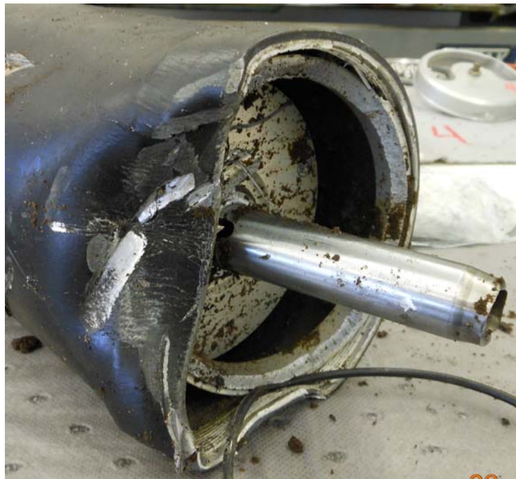
Photo #5 –Retained Piston/Feathering Spring
