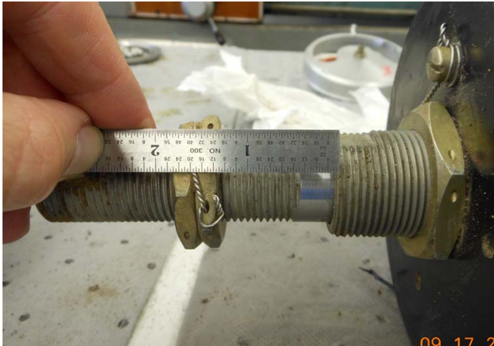
Photo #6 – Pitch Change Rod Extension
