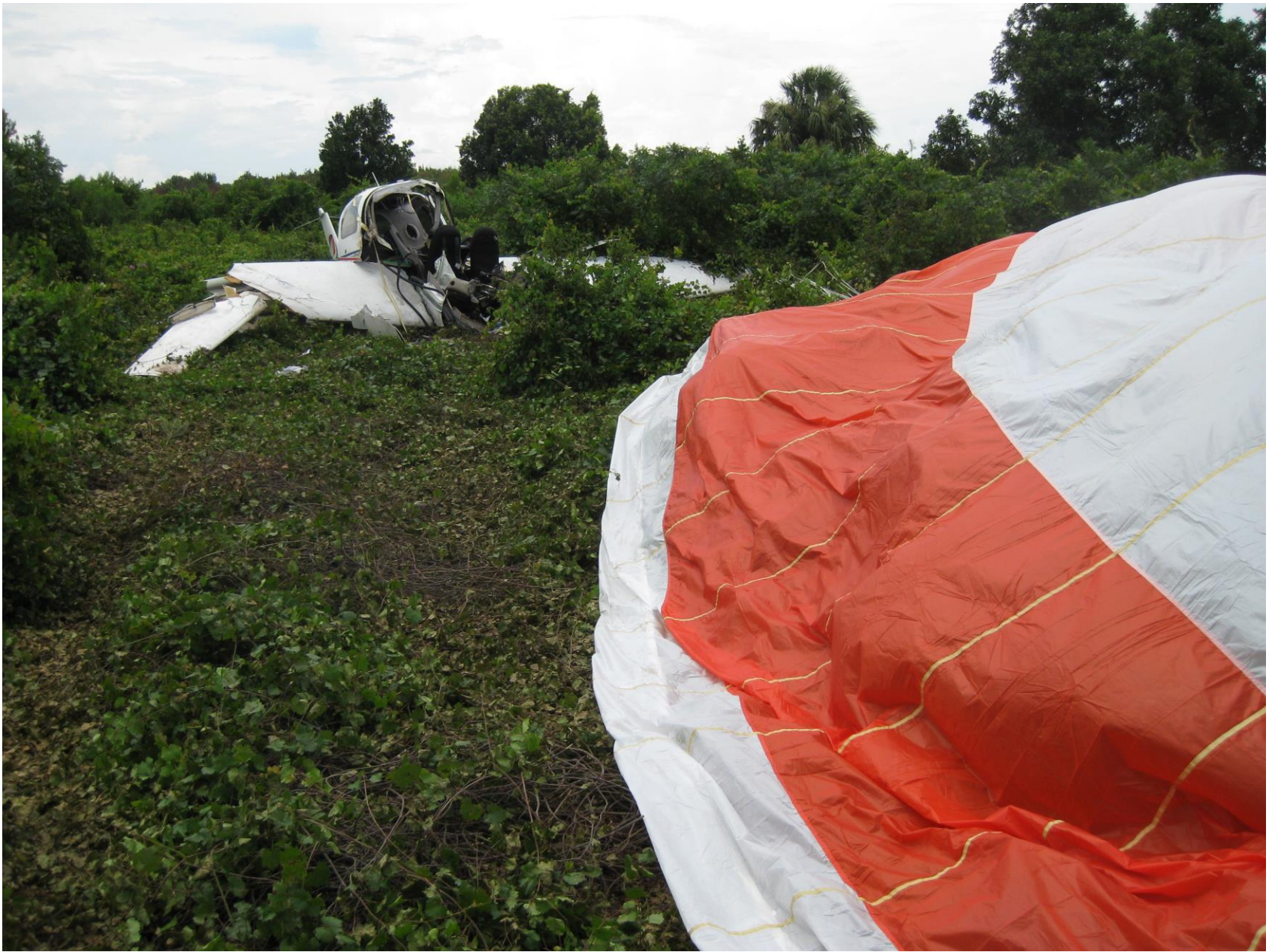
Photo 6 – View of CAPS deployed and airplane wreckage
