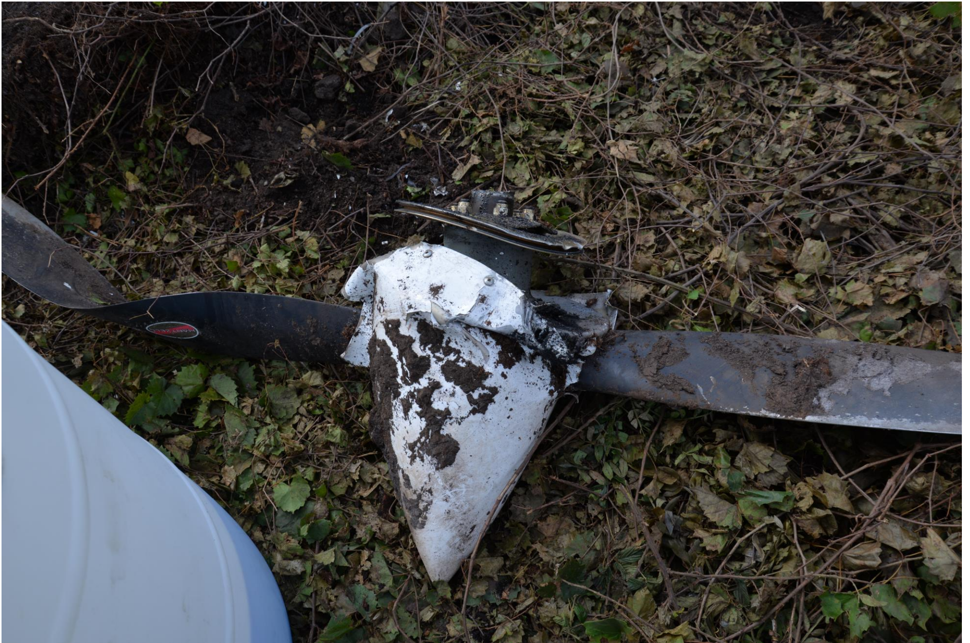
Photo 8 – View of separated propeller
