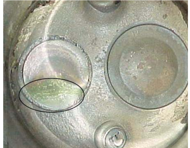
Burned Exhaust Valve
