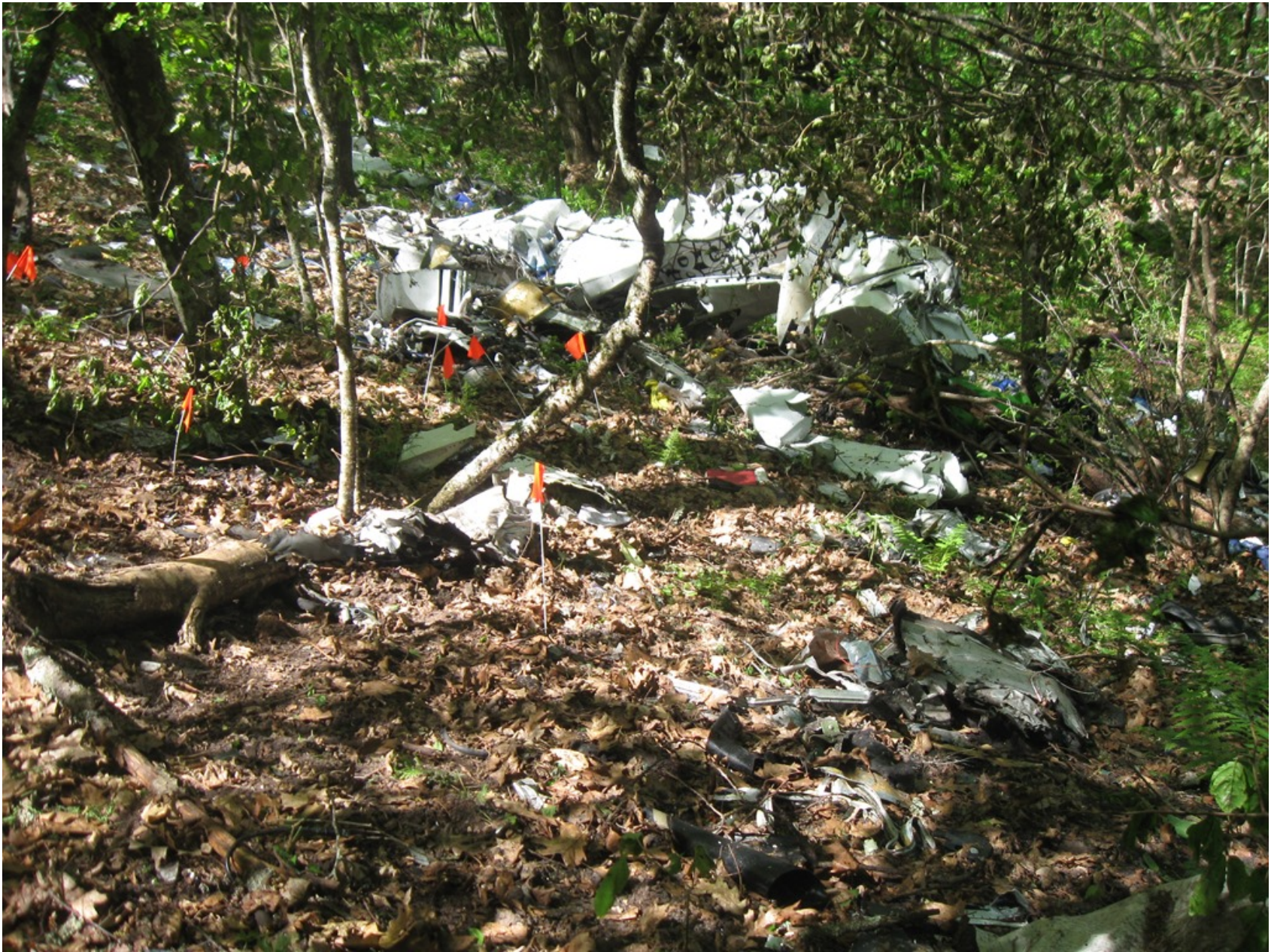
Photo 2 – View of Debris Path and Aft Fuselage
