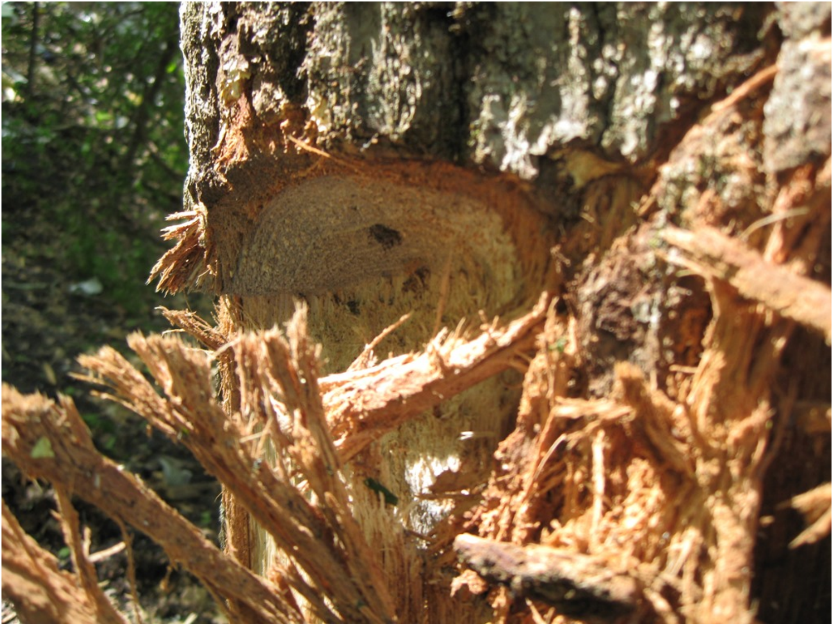
Photo 4 – View of Slashed Tree Trunk with Paint Transfer (FAA)
