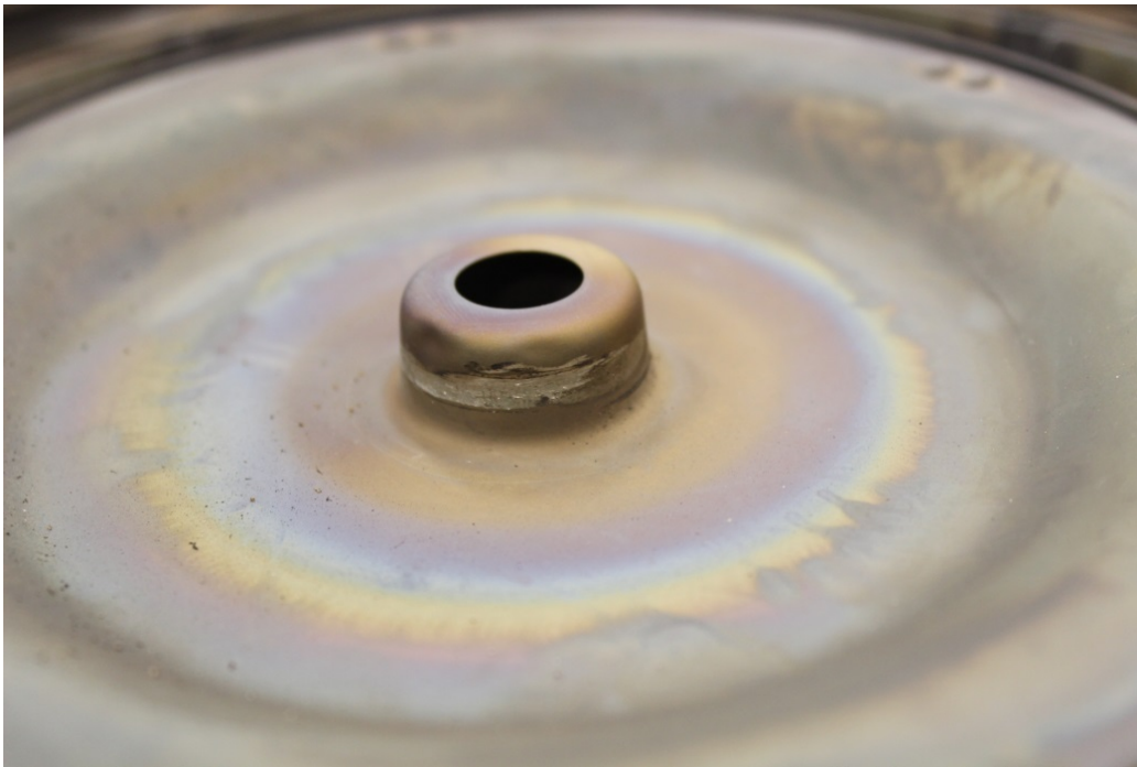
Photo 8- Turbine Baffle Center Bore Rub
