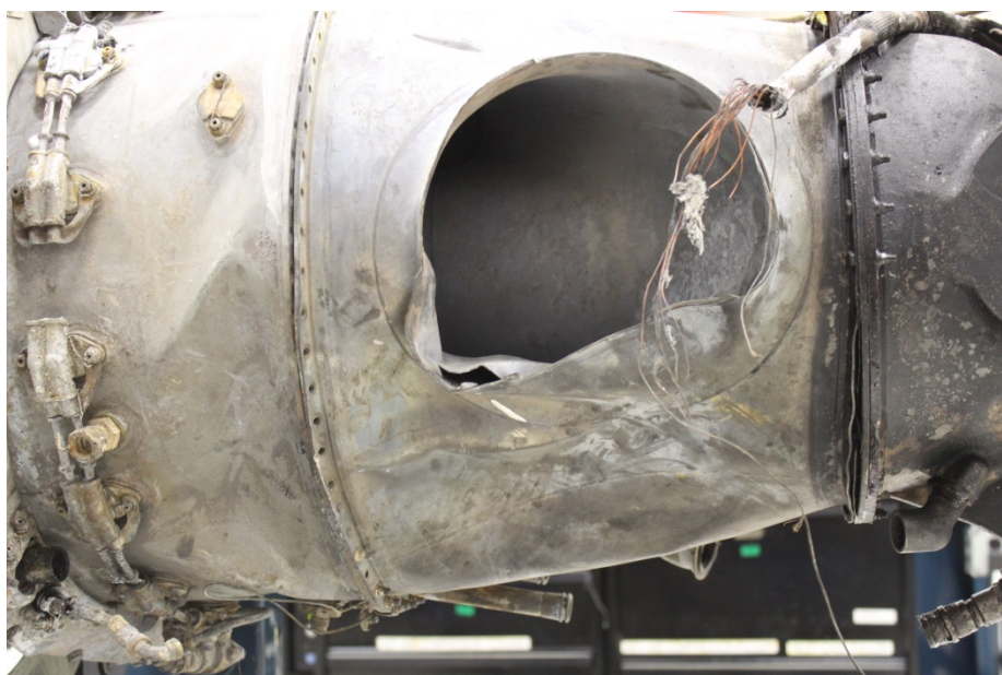
Photo 4- Right Side Exhaust Port and Stack Separated, Exhaust Case Impact Deformation
