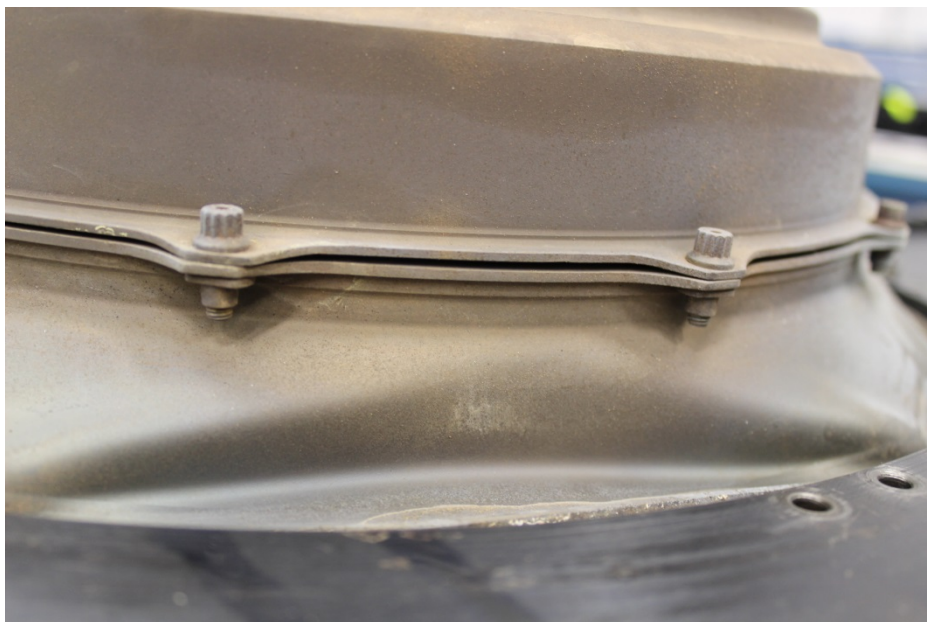
Photo 9- Power Turbine Case to Exhaust Duct Mating Flange Separation
