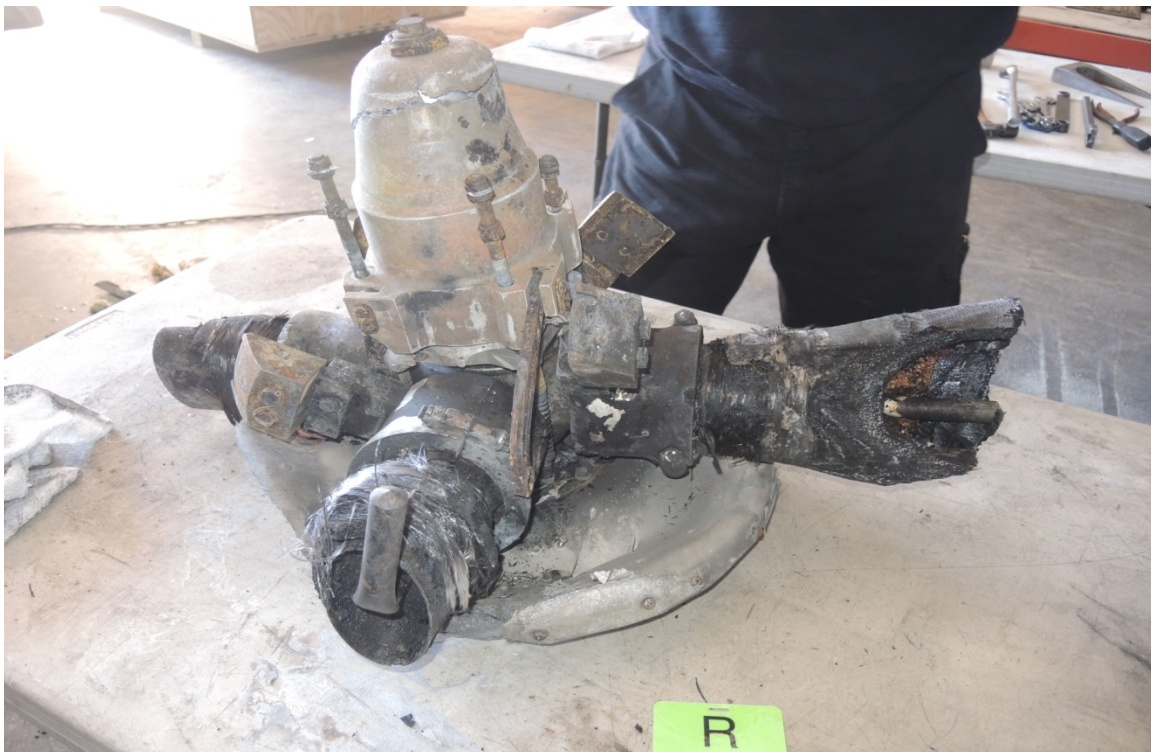
Photo #2, right propeller as received.
