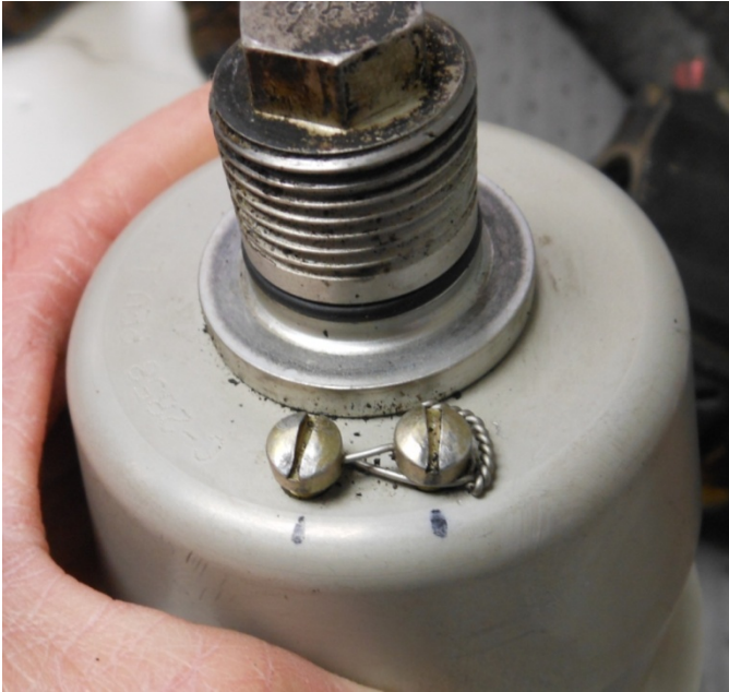
Photo #9, damaged feather stop screws.
