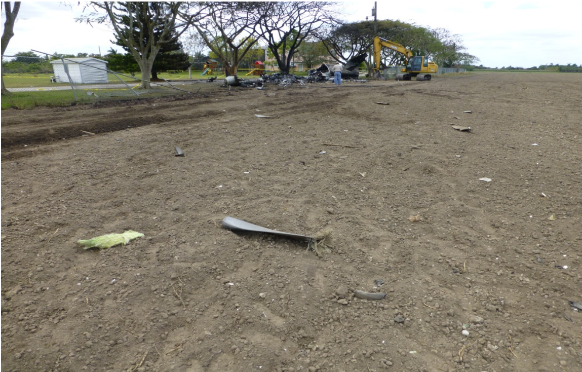
Photo #3, fragmented propeller blades.
