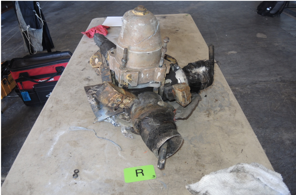
Photo #1, right propeller as received.
