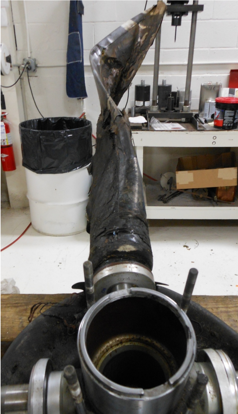
Photo #11, Blade #1 with impact marks aligned.
