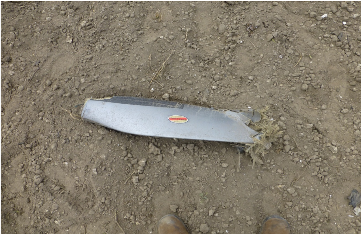
Photo #4, fragmented propeller blade.
