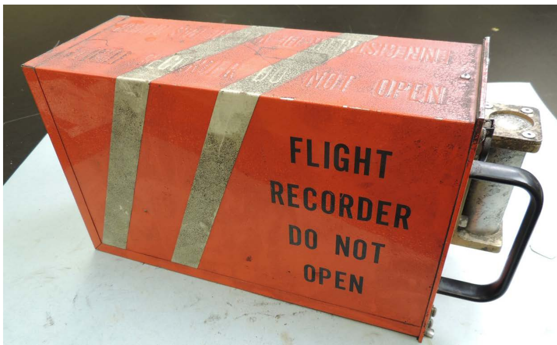
Figure 1. Fairchild A-100S CVR recovered from the Beech 1900C, YV1674.
