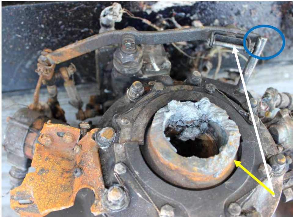
Photo No. 1, The carbon block is missing (white arrow). The propeller reversing lever is above its respective guide pin (blue oval). Sectioned end of the propeller shaft (yellow arrow).
