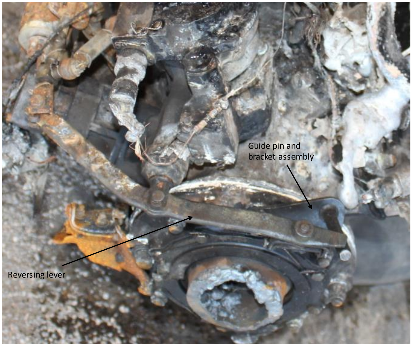
Figure 1 Image of side A (see Figure 3) of the reversing lever and guide pin and bracket assembly as-installed on the engine after the accident.
