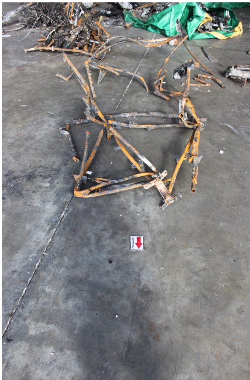
Photo 7 - NTSB Digital Photograph. View of the Tubular Structure From Fuselage Stations 91.25 to 168.5.
