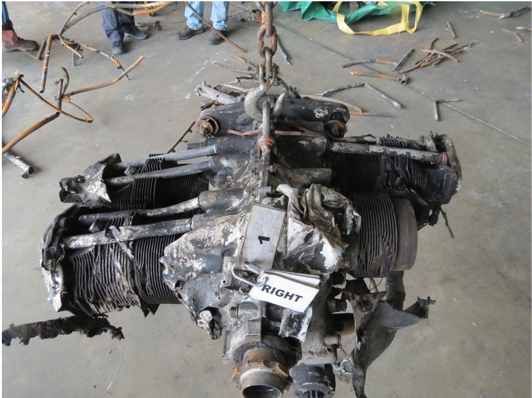
Photo 9 - Lycoming Digital Photograph. View of the Right Engine Assembly.
