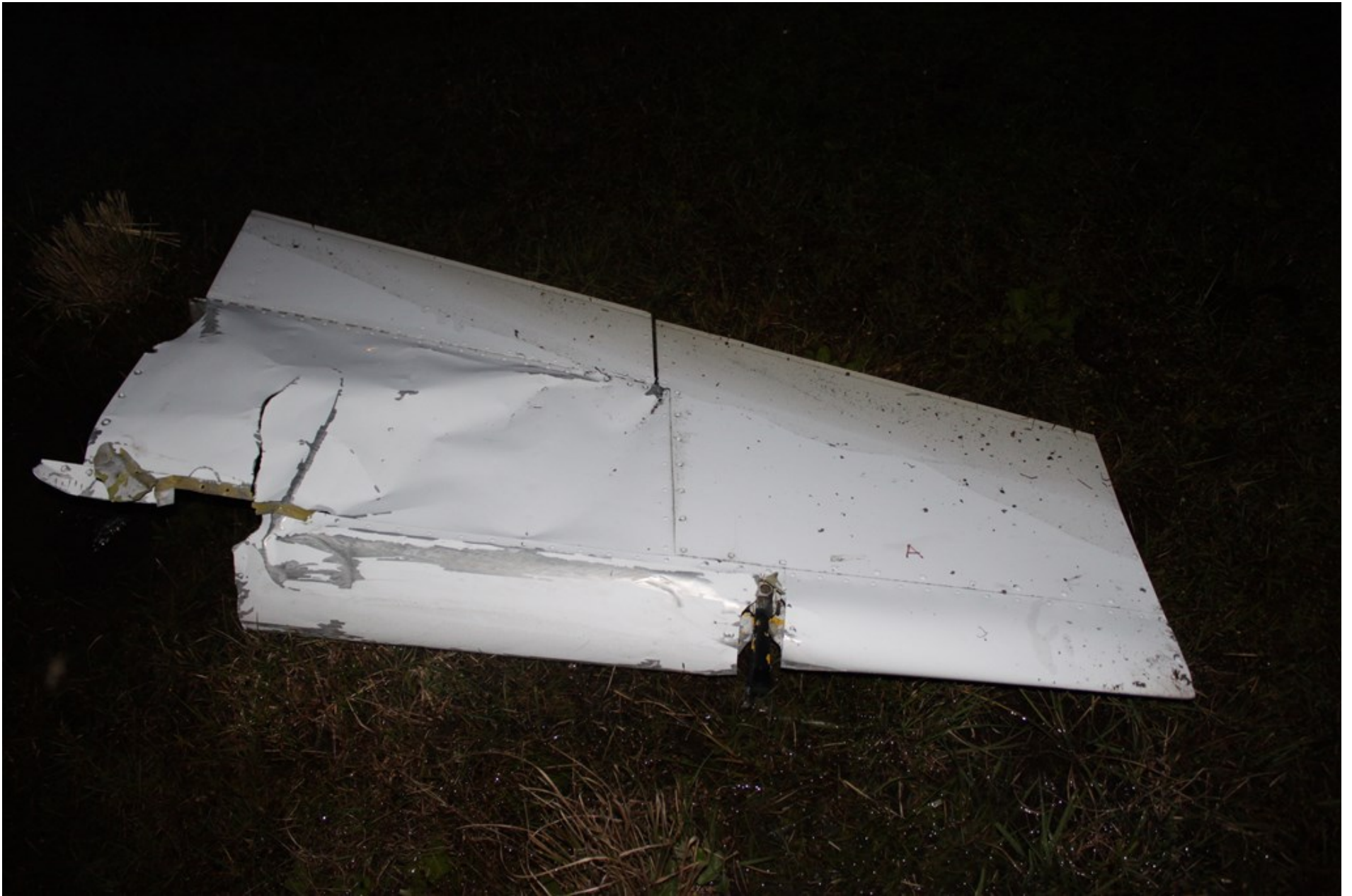
Photo 2 - NTSB Digital Photograph. View of the Separated Rudder with Rudder Trim Tab in the As-Found Location.
