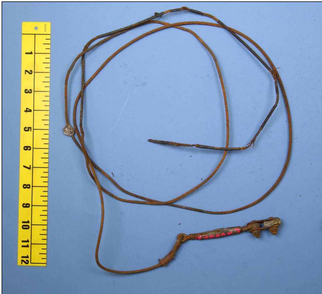
Figure 6. Overall image of the rudder cable as-received.
