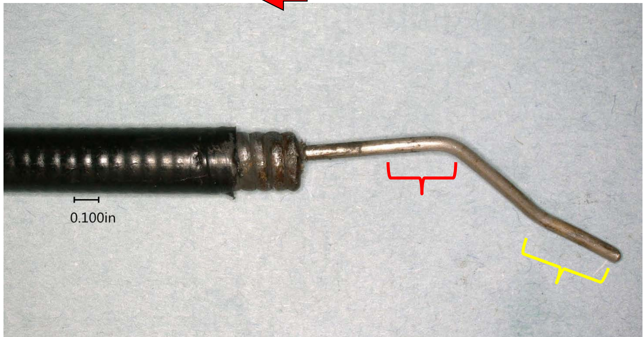
Figure 3. view of the trim cable with the inner wire retracted (top) and extended (below). The wear area is denoted by the red bracket. The yellow bracket highlights the area of the inner wire shown in figure 5.
