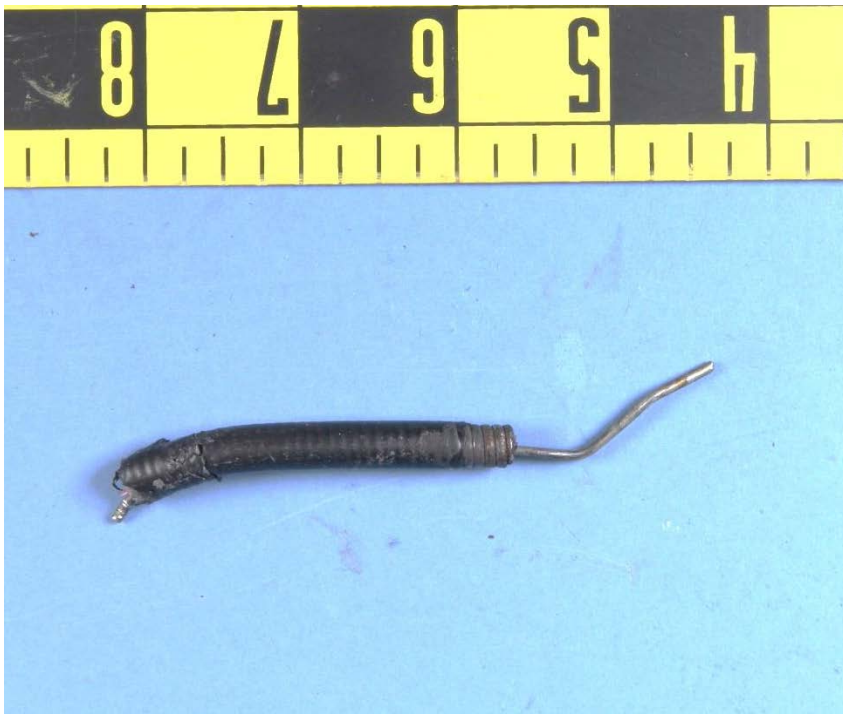
Figure 1. Overall views of the as-received elevator horn, looking aft (top) and elevator trim cable section looking outboard (below).
