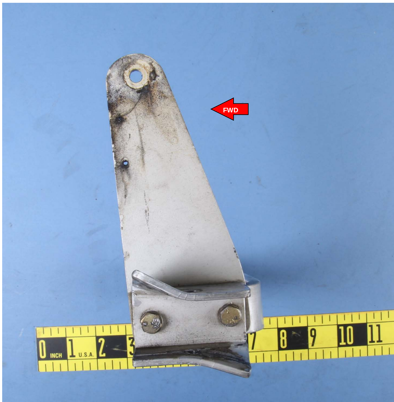
Figure 2. View of the left side of the elevator horn showing the deformation of the left elevator attachment channel.
