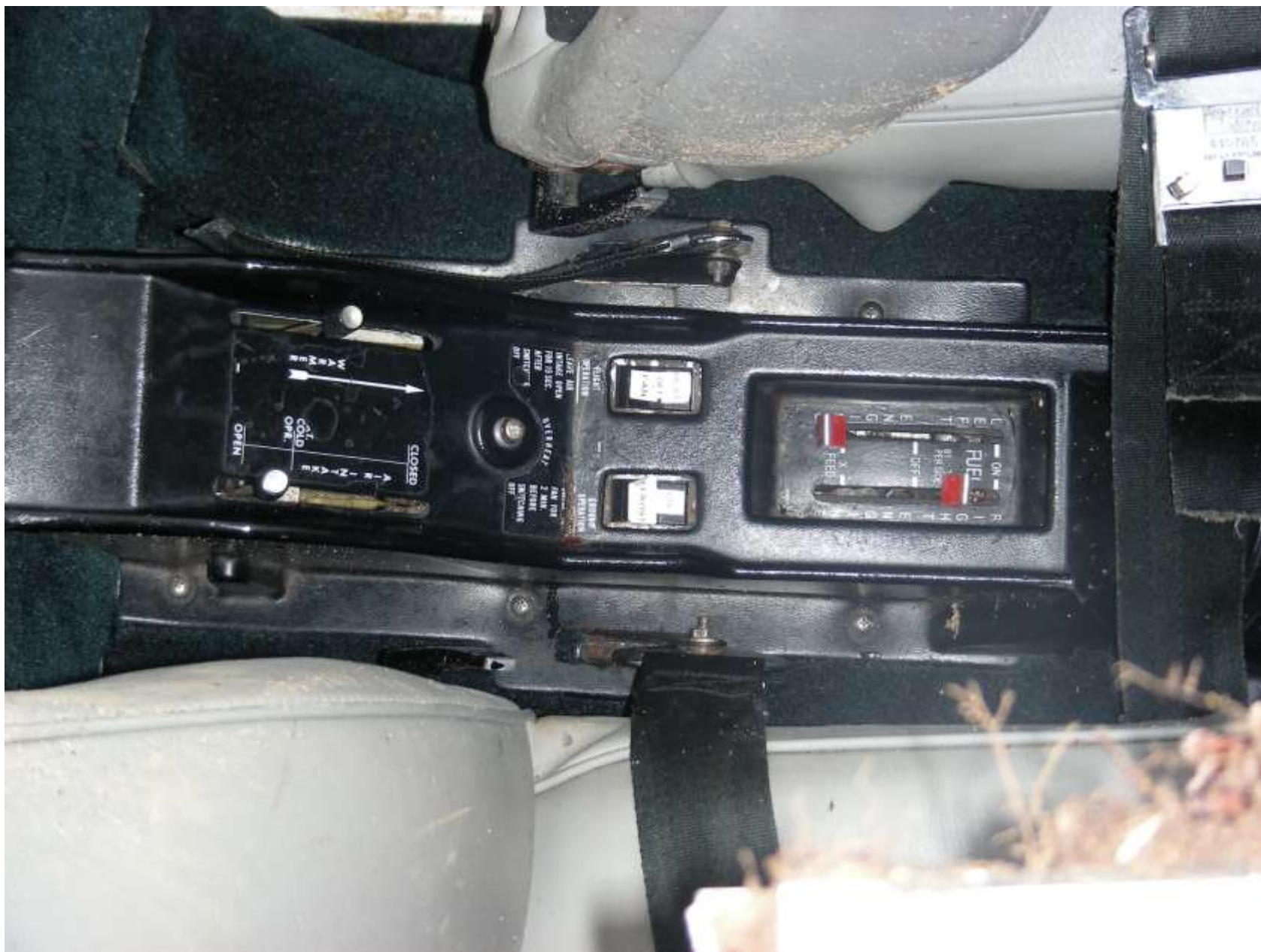
Photo 6 – View of Fuel Selectors as Found
