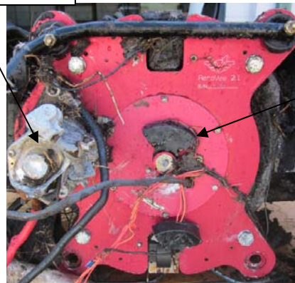
Ignition system and starter mount
