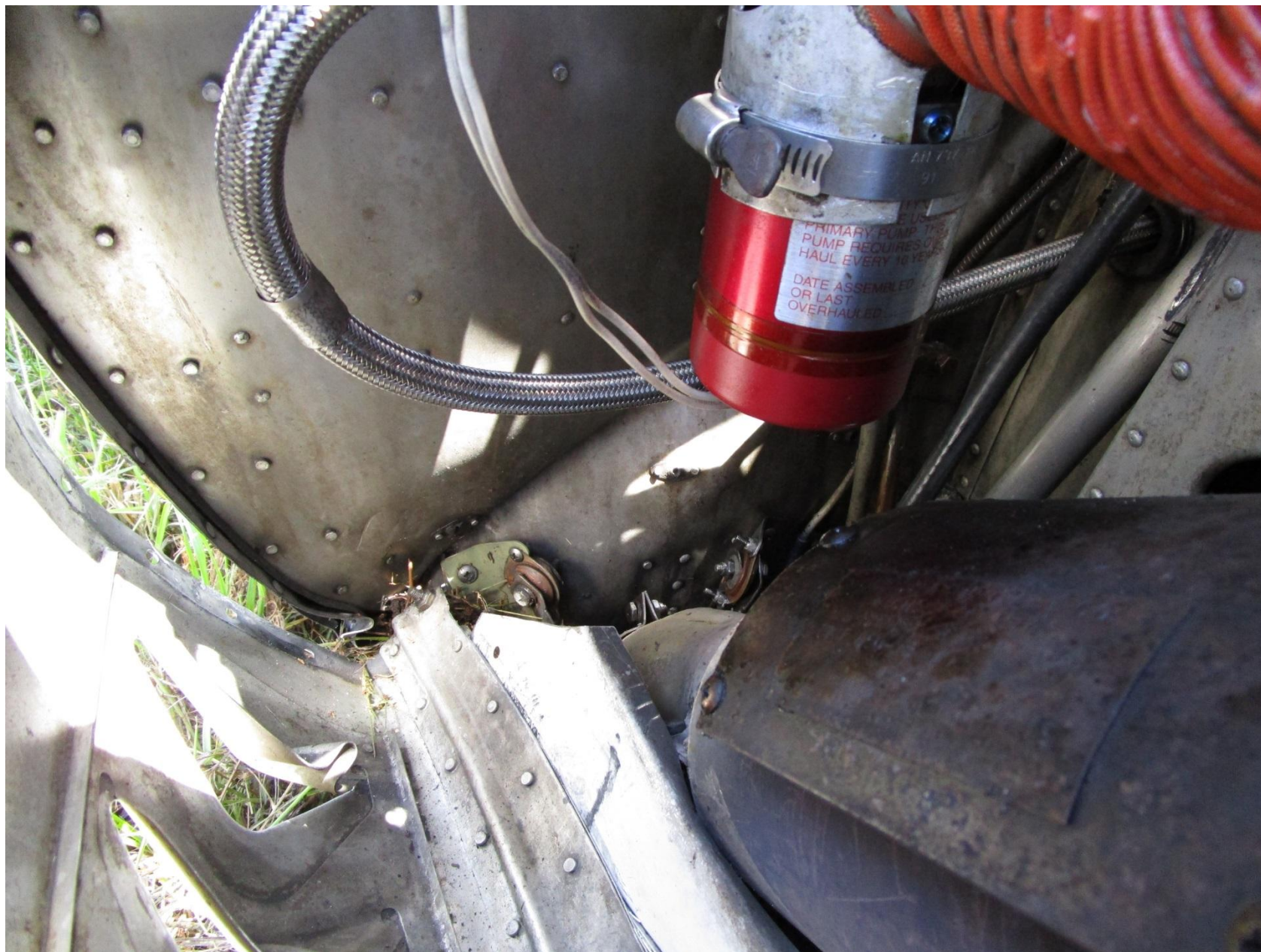
Photo 1-View of buckled firewall
