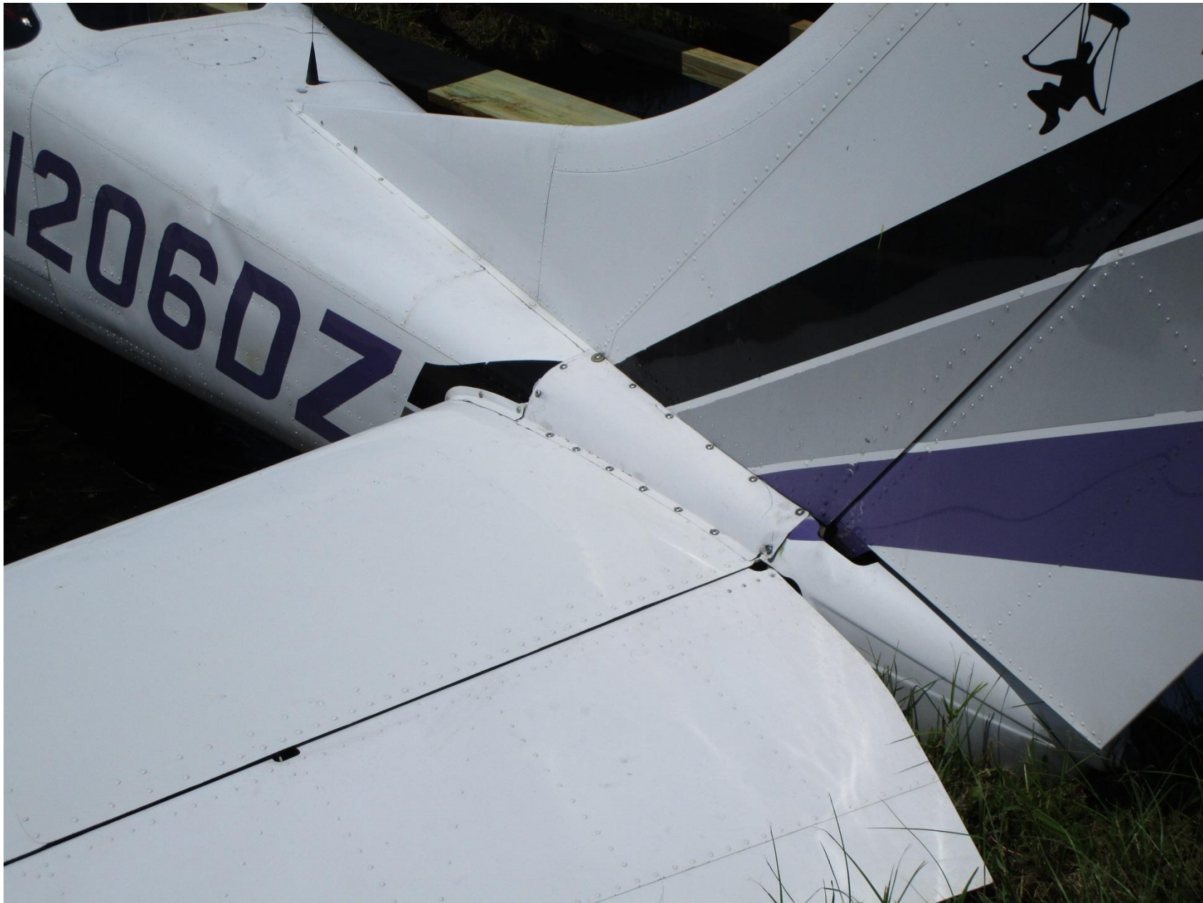
Photo 2-View of buckled empennage
