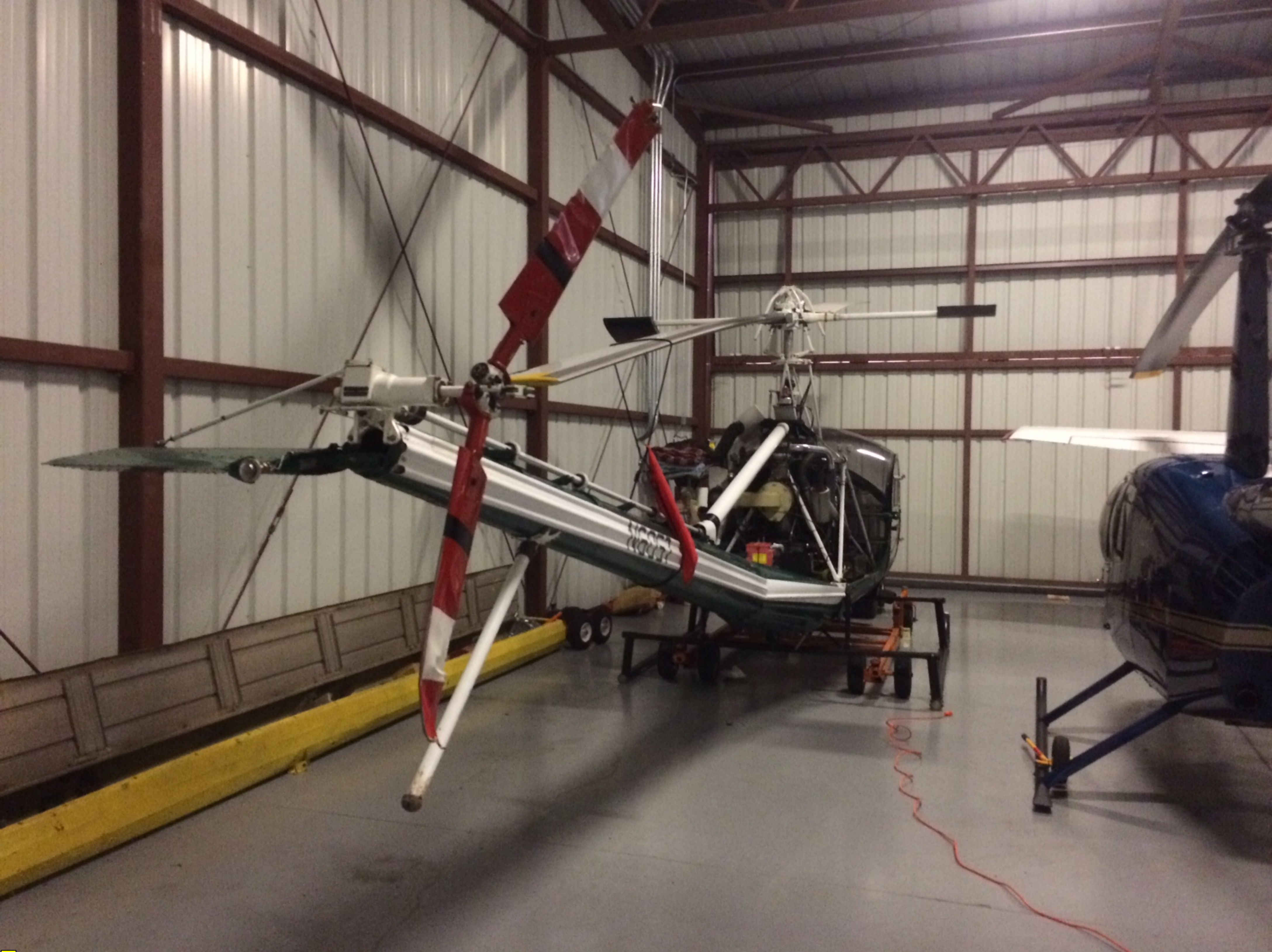
Photo 2 – View of Damage to Tail Rotor (Photo Courtesy of Flight Instructor)
