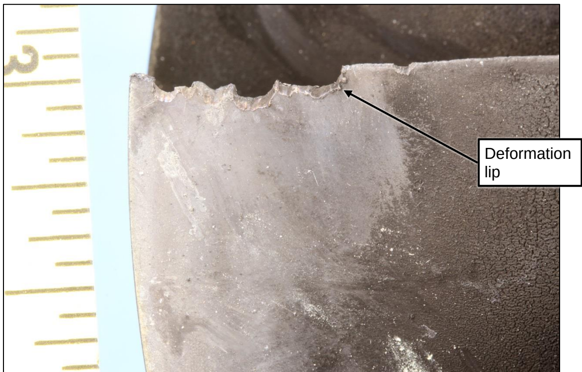
Figure 5. Close views of impact damage near the tips of axial compressor blades.
