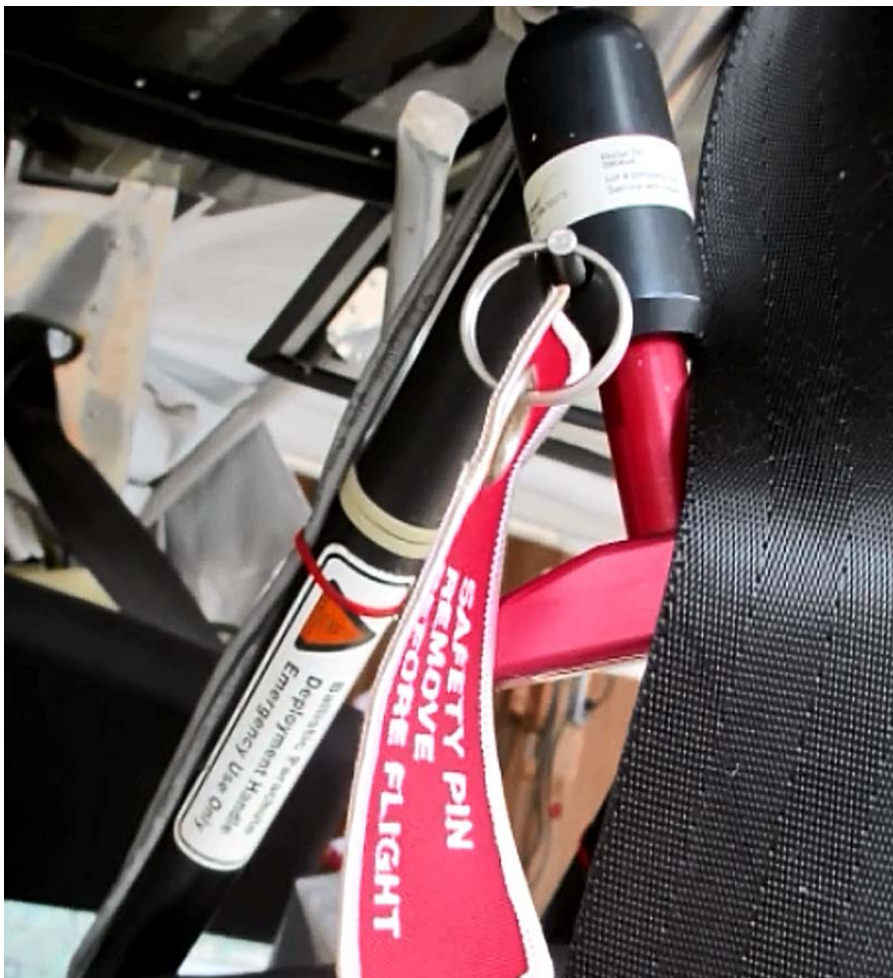
Photo 4: BRS Safety Pin in Place - Post Recovery
