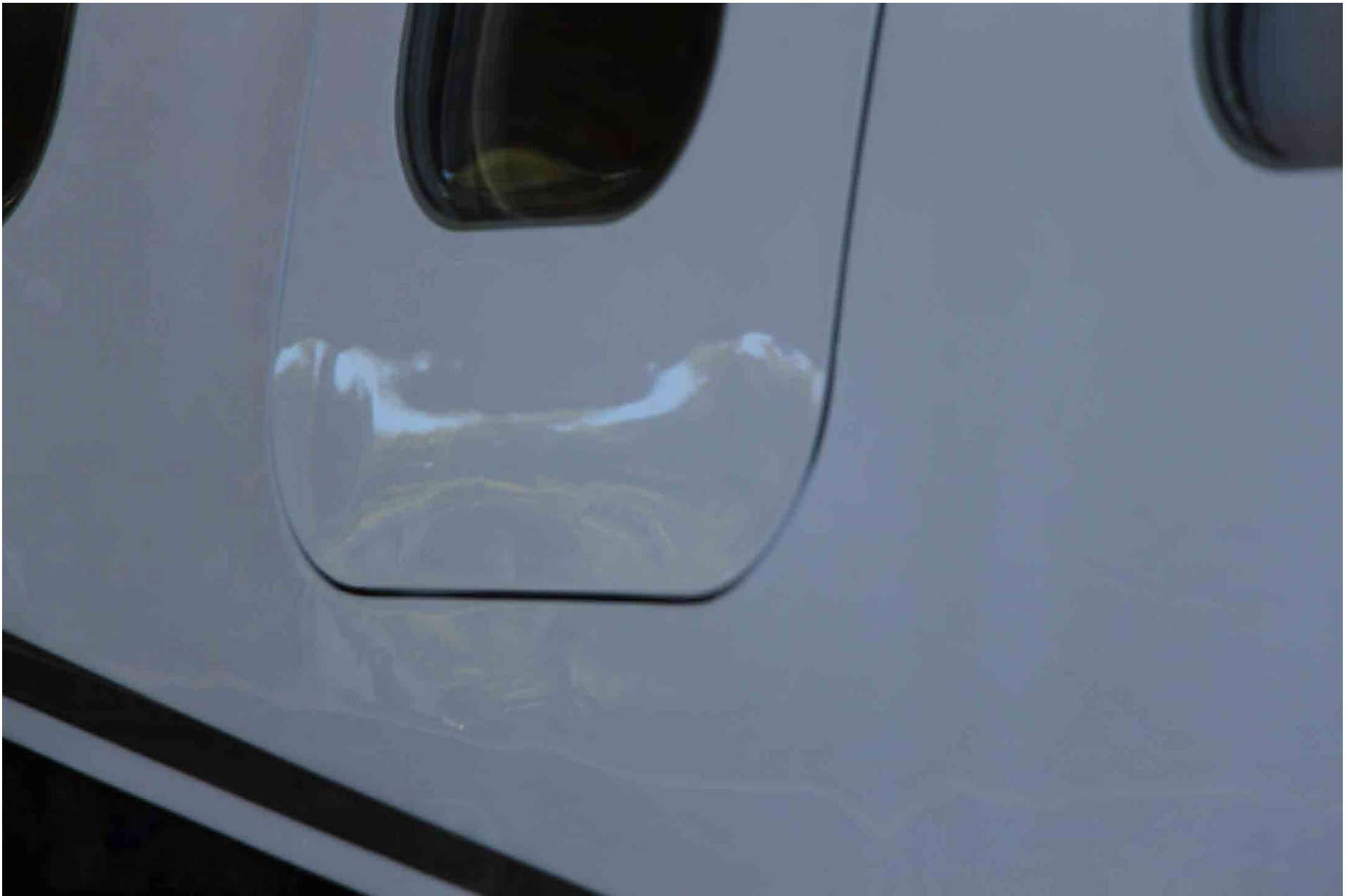
Photo 5 – View of a TBM900 Emergency Exit Door
