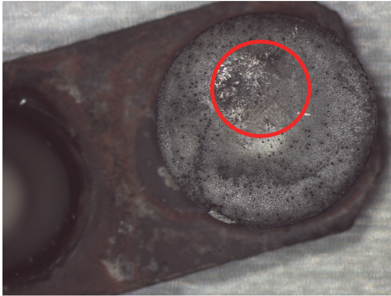
Figure 22. Material transfer pit on contact surface denoted by circle. The armature which the contact is mounted to is normally shiny, but was coated with brown rust.
