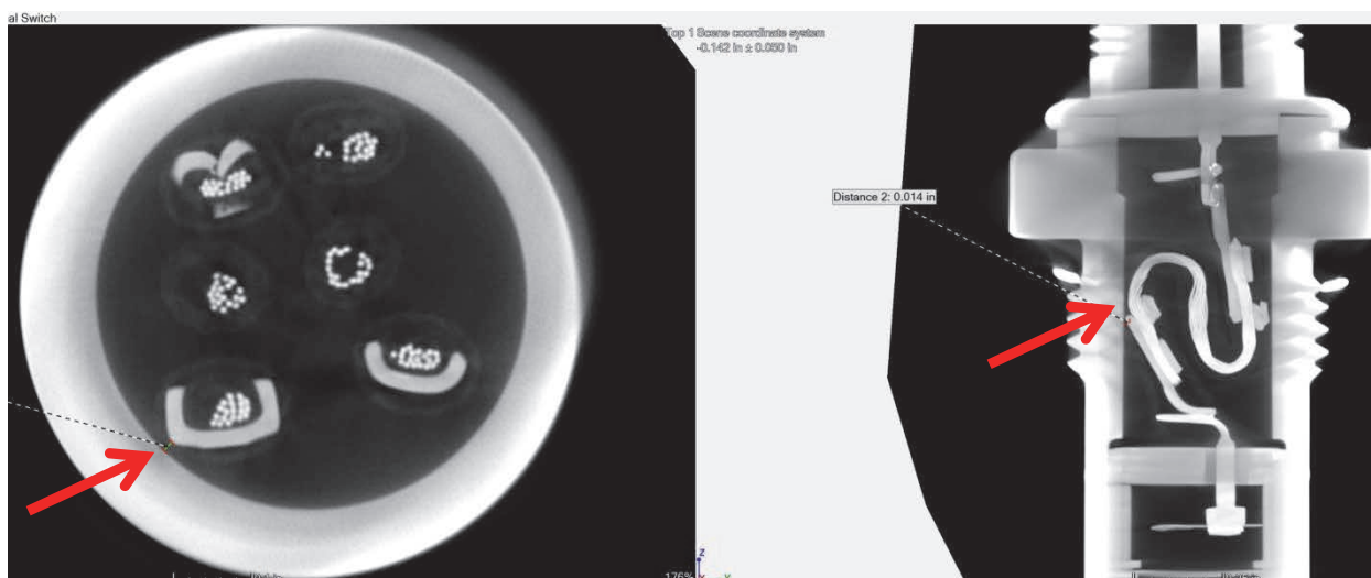
Figure 15. CT images with arrows showing .014" measurement.
