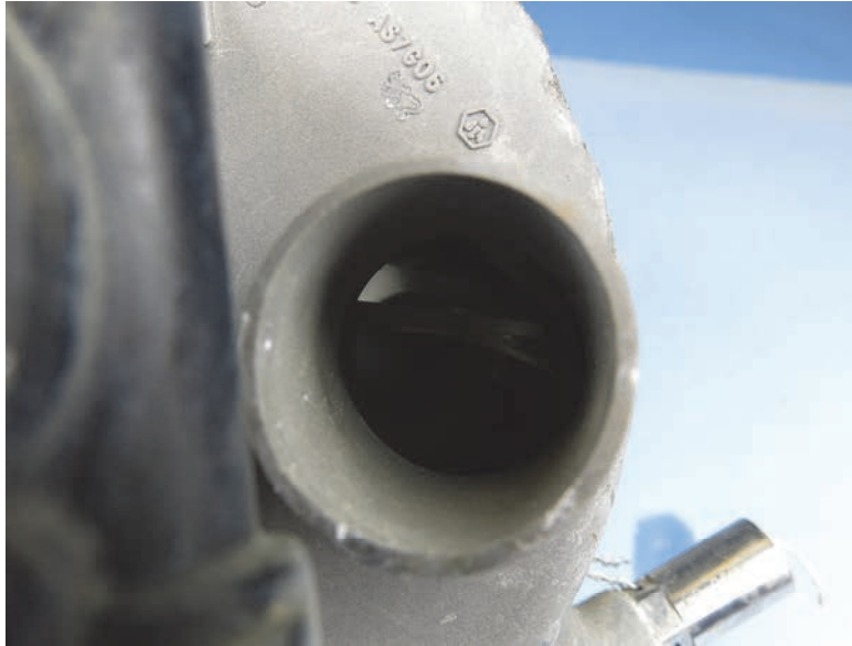
Figure 48. Position of hot air distributor valve.
