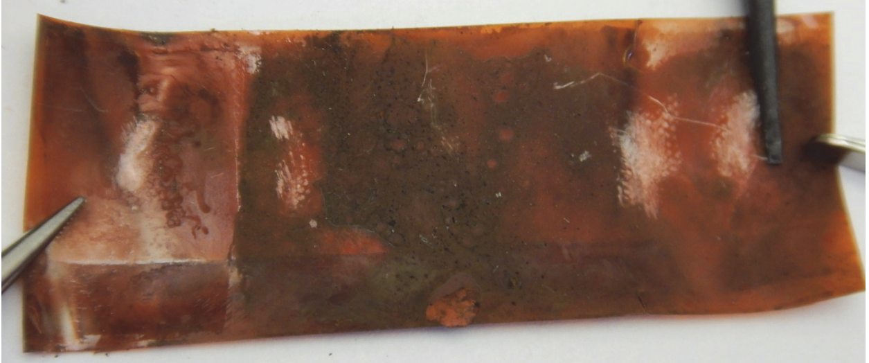
Figure 19. Residue on unrolled Kapton liner.
