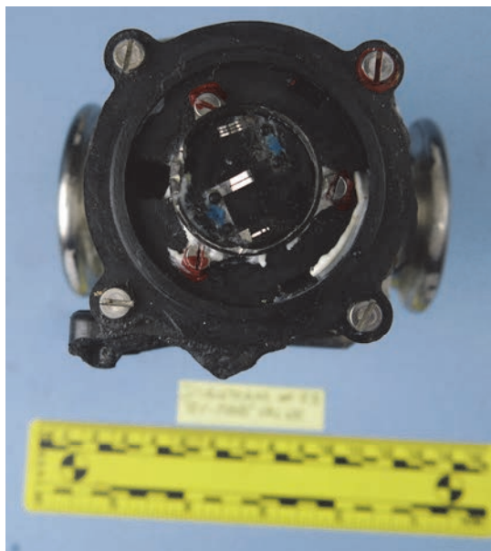
Figure 37. Exposed switch contacts.
