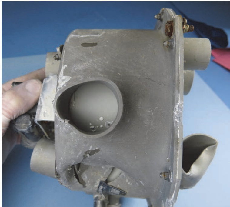
Figure 47. Position of hot air distributor valve.
