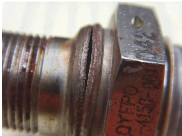
Figure 14. N900KN OTSW after the welded area burst when heated.
