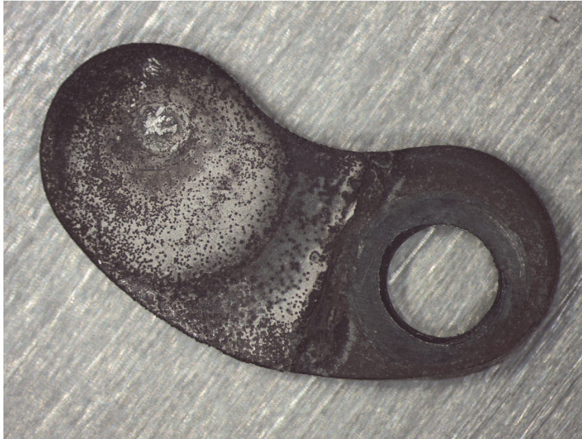
Figure 24. Contact material transferred.
