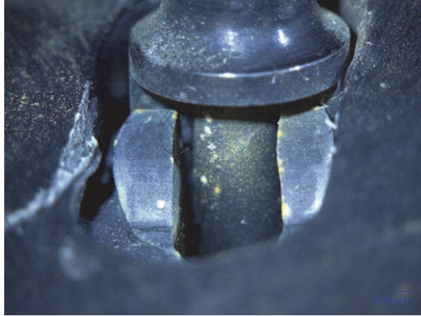
Figure 55. The PRES MODE switch was found in the AUTO position. The locking gate had no imprints or scars on the MAX DIF side of the lock shown here.
