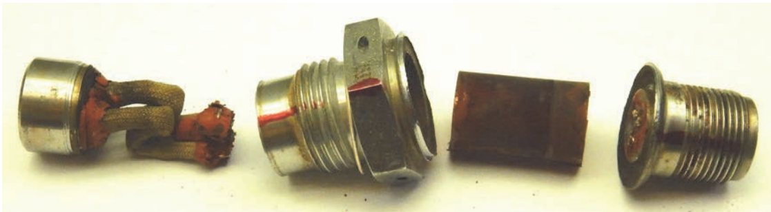
Figure 13. This photo of the disassembled N900KN OTSW shows the capsule containing the thermal switch at the left, the mounting body to the left of center, an insulating Kapton liner to the right of center, and the electrical connector (shown at top in previous photo) on the right. The wires had to be cut during the examination at the base of the electrical connector and a small split in the Kapton was created.
