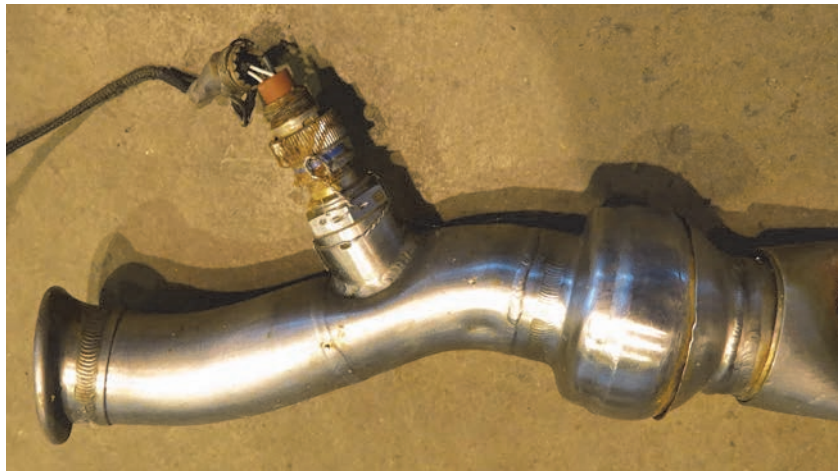
Figure 9. OTSW switch prior to removal from wreckage on June 4, 2015.
