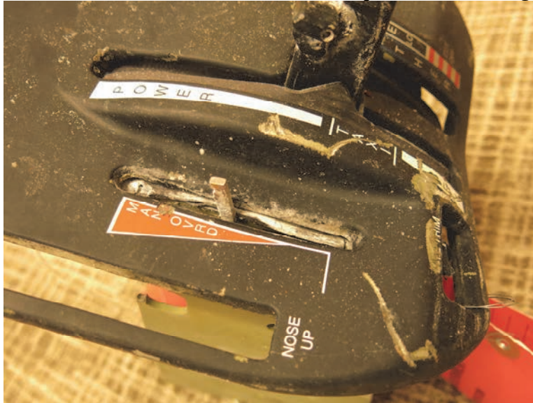
Figure 65. Throttle quadrant position of power lever, manual over-ride, and missing pitch trim indicator.
