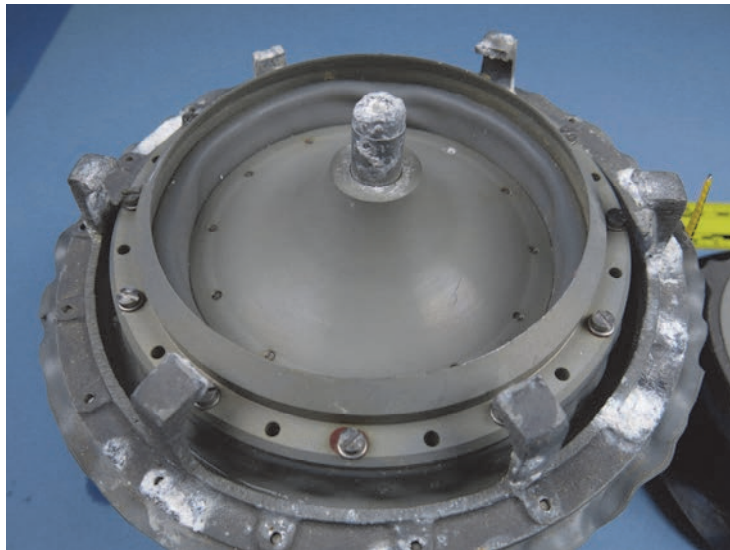
Figure 34. The main valve body on the broken central shaft. The shaft broke flush with where it had entered the mounting flange visible in the next photo.
