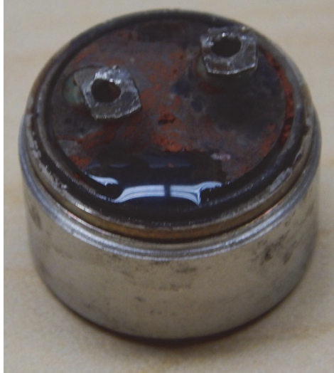
Figure 21. Water on surface of switch module.
