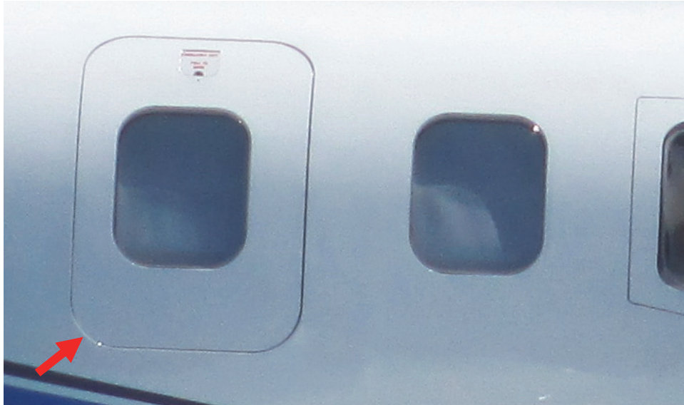
Figure 7B. The red arrow in this enlarged and cropped photo shows sunlight reflecting off of the emergency escape hatch frame. The hatch is designed to slightly protrude when the cabin is pressurized and the sunlight reflection would not be possible in that position.
