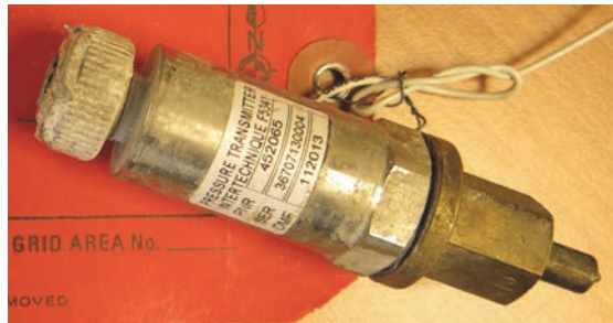
Figure 60. Intertechnique pressure transmitter. Note: The wire is loosely attached to keep the switch from being lost.
