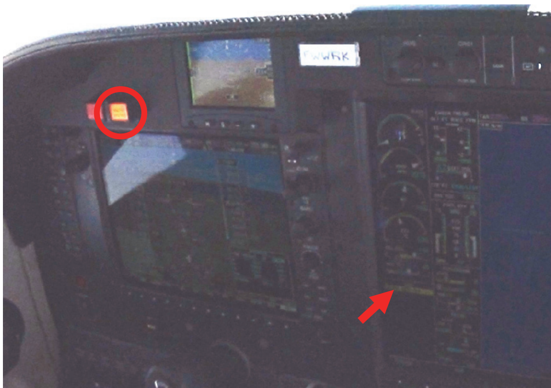
Figure 5. Master Warning Annunciator illuminated (see circle) and CAS message (see arrow) being displayed. The engine torque display is not visible.
