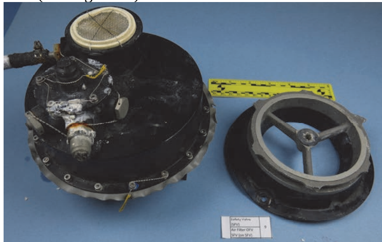
Figure 33. The complete two portions of the safety valve.
