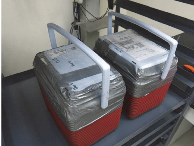
Figure 27. Examples of the sealed cooler boxes filled with water and pressurization parts.
