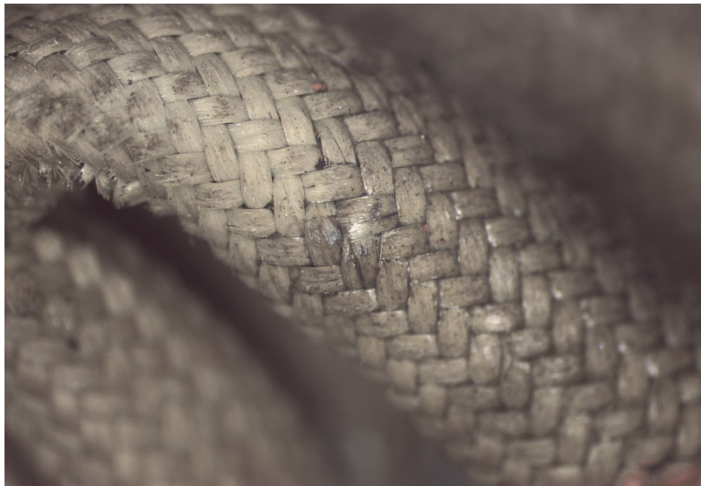
Figure 18. Worn area of wire insulation. (typical)
