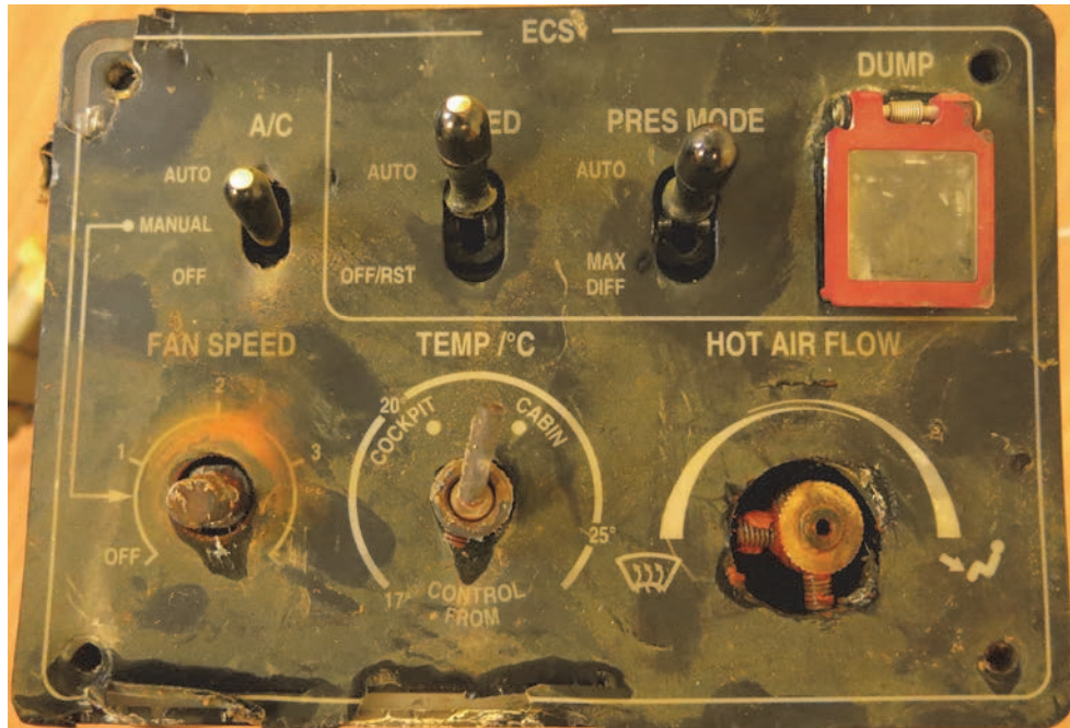
Figure 49. Face of the ECS Control Panel with brown rust deposits.
