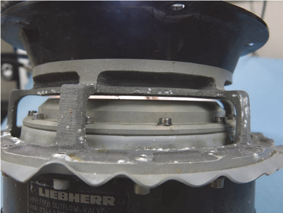
Figure 31. Close-up view of the 0.07” opening of the outflow valve main valve body when placed with the poppet resting on the internal spring. The white areas are organic ocean material and corrosion.
