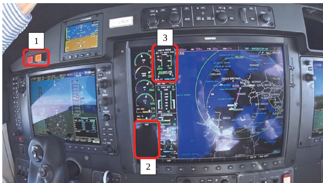
Figure 4. Left and center flight displays at FL280. (1) denotes Master Warning annunciator in red and Master Caution annunciator in amber. (2) denotes CAS message area. (3) denotes pressurization display.
