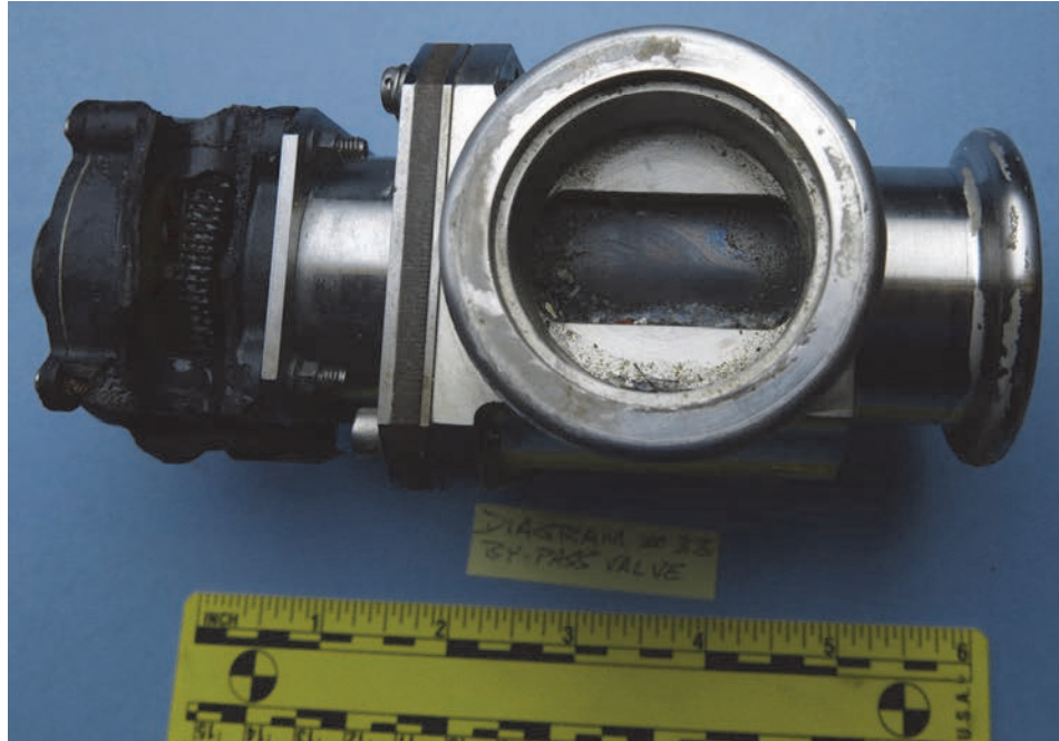
Figure 40. Closed bypass valve opening.
