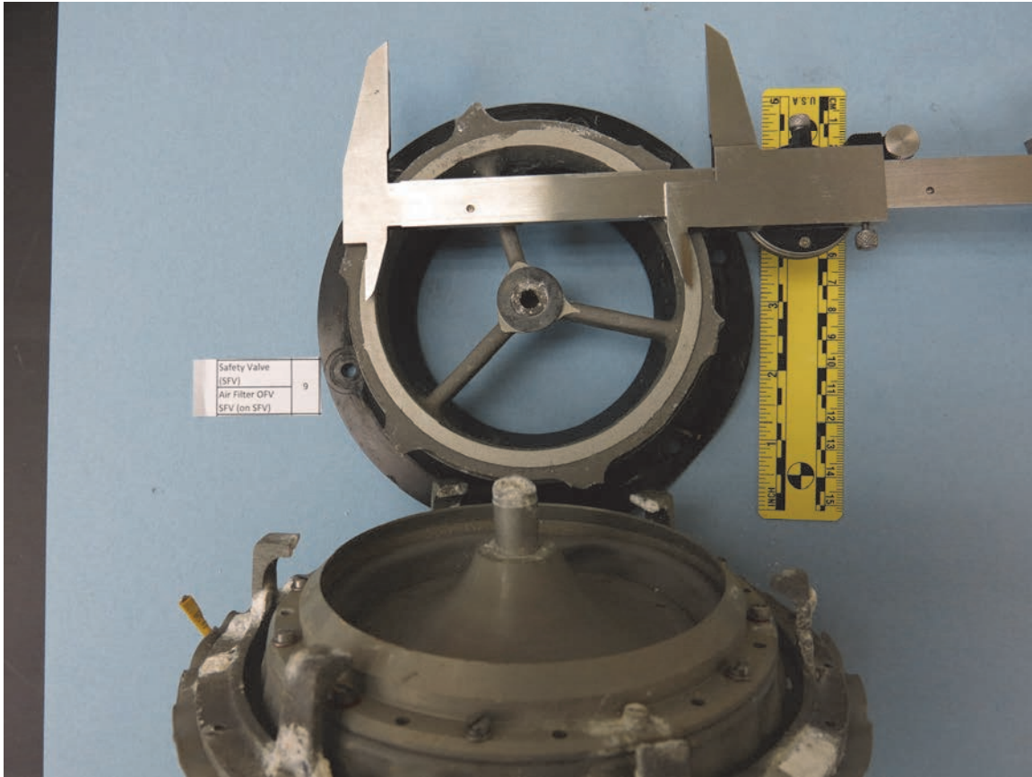
Figure 35. The calipers are set to the diameter of the main valve body knife-edge, and placed on the seating surface which the knife-edge would rest against in an intact valve.
