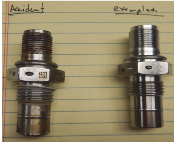
Figure 10. OTSW switch from N900KN and an exemplar. The electrical connector is at top and the capsule with the switch contacts is at the bottom.
