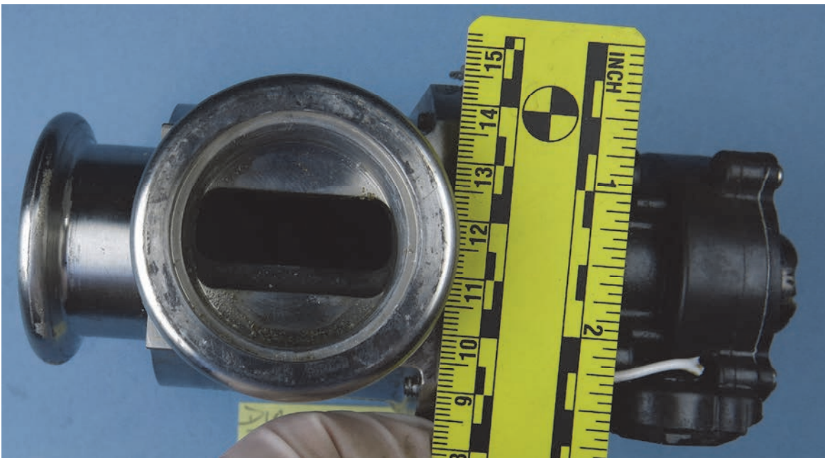
Figure 39. Partially closed bypass valve opening.
