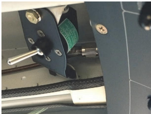
Figure 64. A switch installed in an exemplar airplane with the toggle in the OFF position. The view is from the copilot seat, so forward would be to the right of the photo.
