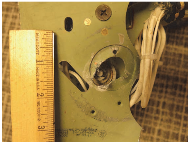
Figure 66. Tearing and displacement of throttle quadrant axle.
