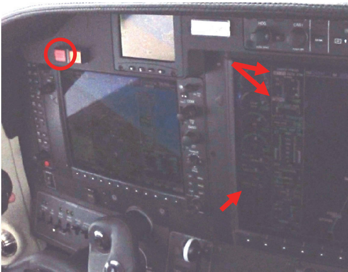
Figure 6. Master Caution Annunciator illuminated, (see circle) CAS message (see single arrow), and double pressurization message (see double arrow).
