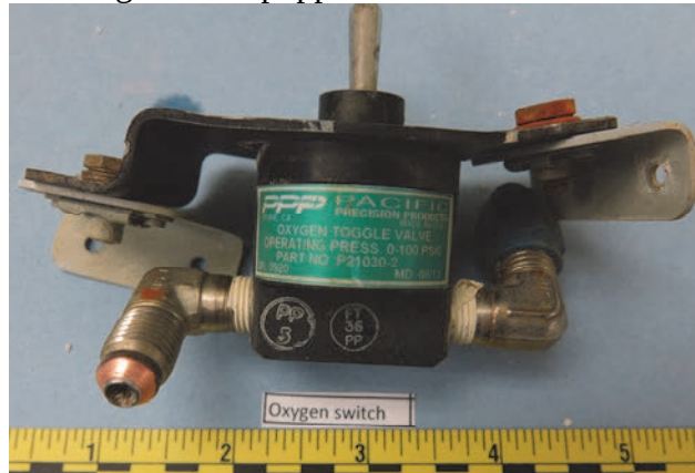
Figure 63. Supplemental oxygen switch. The scale at the bottom is marked in inches.
