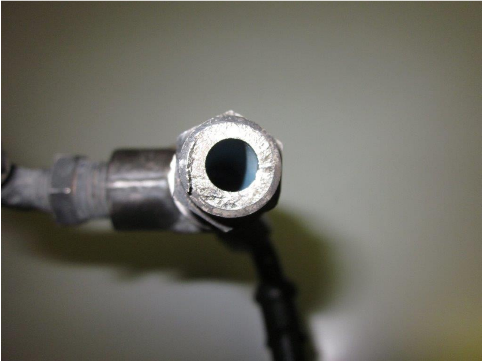
Photo 5 – Nipple Fracture Face – Opposite Side (Courtesy FAA)
