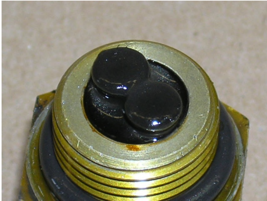
Photo No. 12 Reduction gearbox chip detector.
