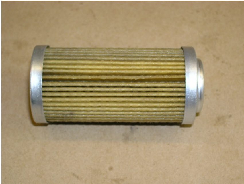
Photo No. 14 Fuel filter.
