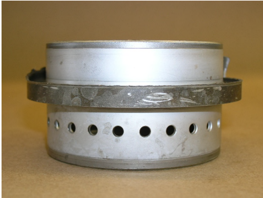
Photo No. 44 Compressor 3 rd stage spacer, centered at position “X”
