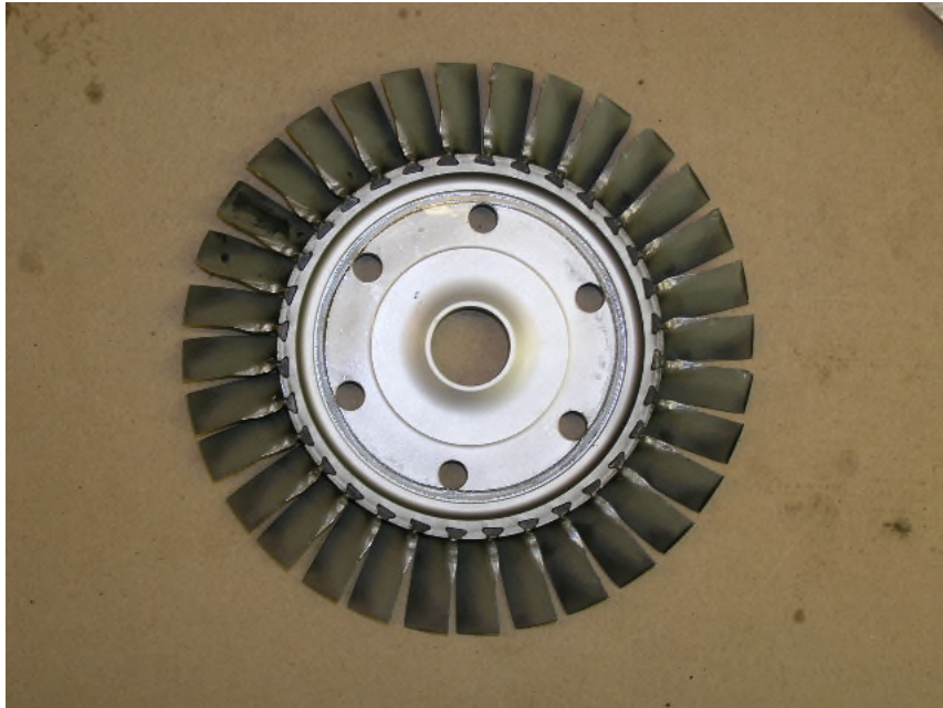
Photo No. 24 Compressor 2 nd stage disc and blades downstream side.
