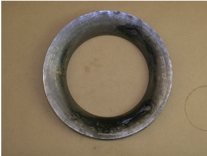
Photo No. 48 Centrifugal impeller shroud.
