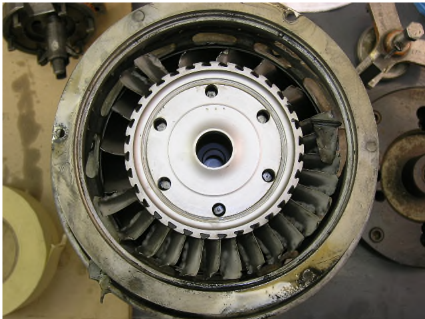
Photo No. 25 Compressor 3 rd stage disc and blades upstream side, in-situ.
