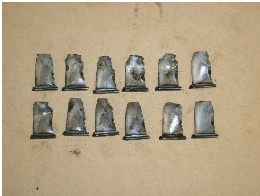
Photo No. 29 Recovered 3 rd stage blade airfoils, alternate view.
