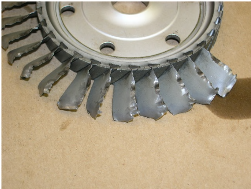
Photo No. 27 Compressor 3 rd stage disc and blades, downstream side.
