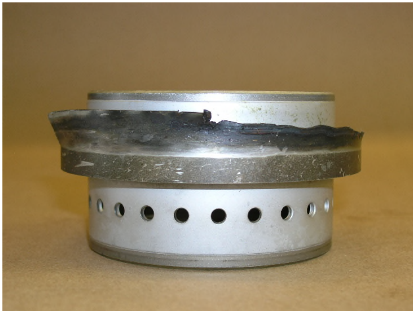
Photo No. 45 Compressor 3 rd stage spacer, centered at position “Z”
