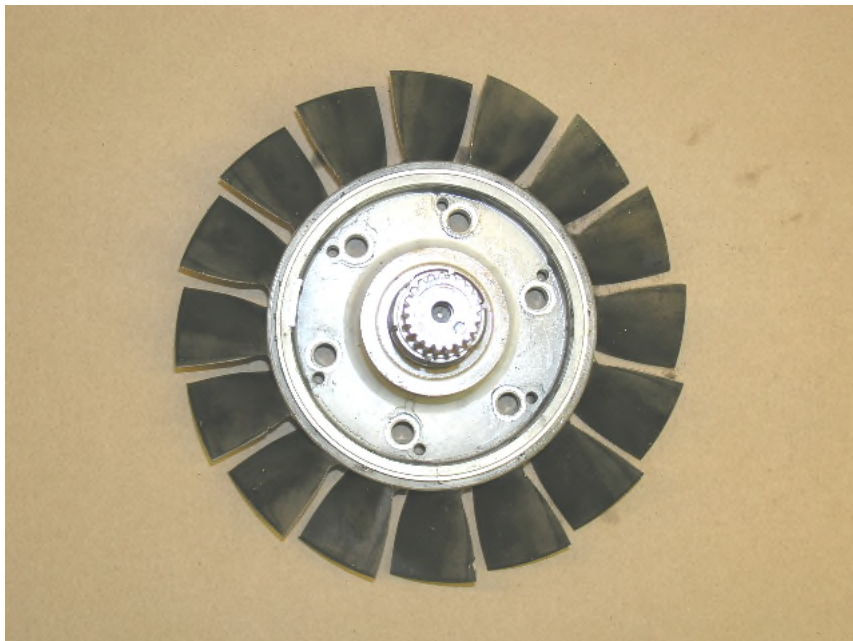
Photo No. 21 Compressor 1 st stage disc and blades, upstream side.
