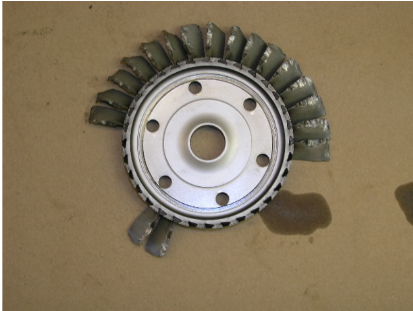
Photo No. 26 Compressor 3 rd stage disc and blades, downstream side.
