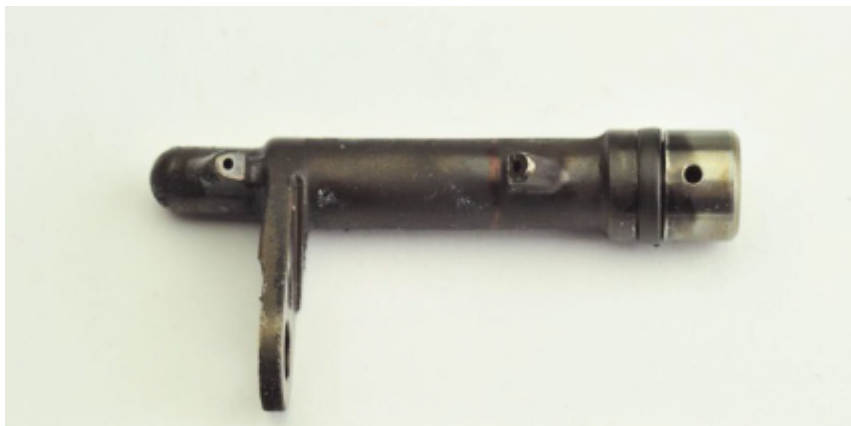
Photo No. 67 No. 2 bearing oil nozzle.
