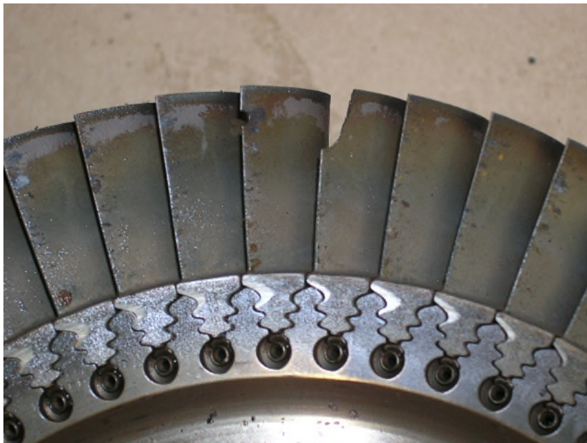
Photo No. 77 Compressor turbine downstream side, detail.
