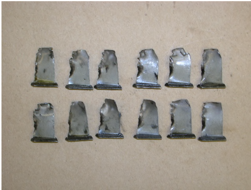
Photo No. 28 Recovered 3 rd stage blade airfoils.
