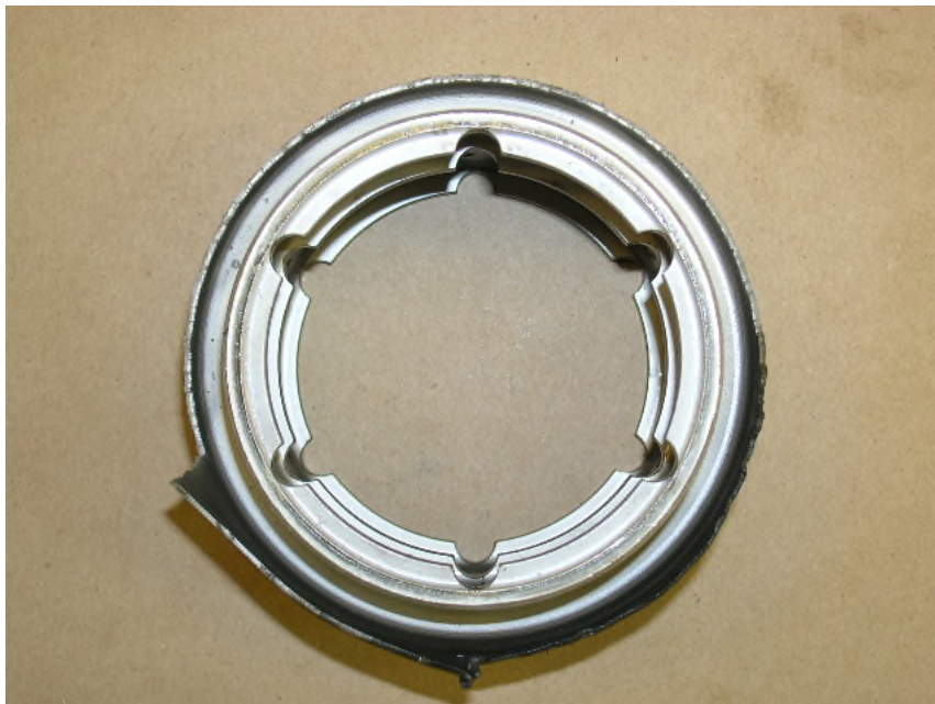
Photo No. 43 Compressor 3 rd stage spacer upstream side, position "X" at 12:00.
