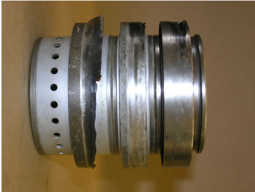
Photo No. 42 1 st , 2 nd , and 3 rd stage compressor spacers quadrant "Z".
