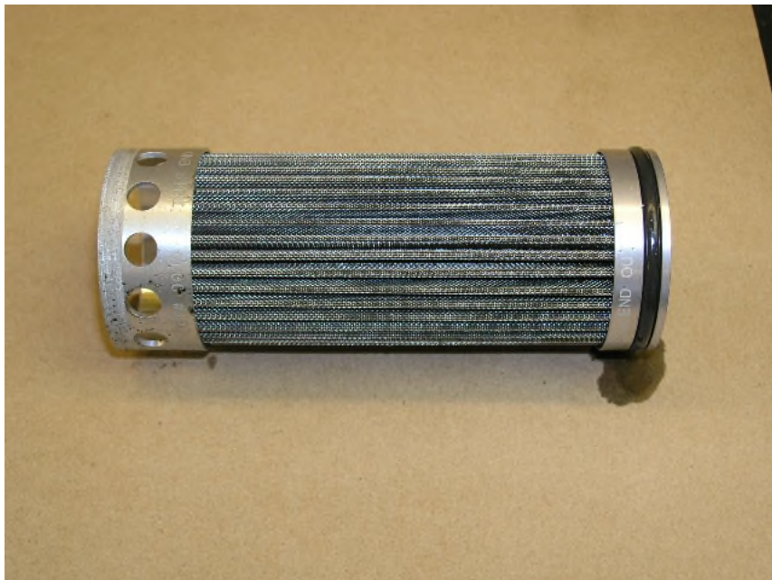
Photo No. 13 Oil filter
