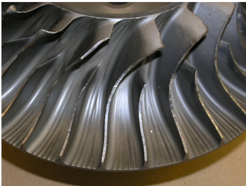
Photo No. 47 Centrifugal impeller, detail.
