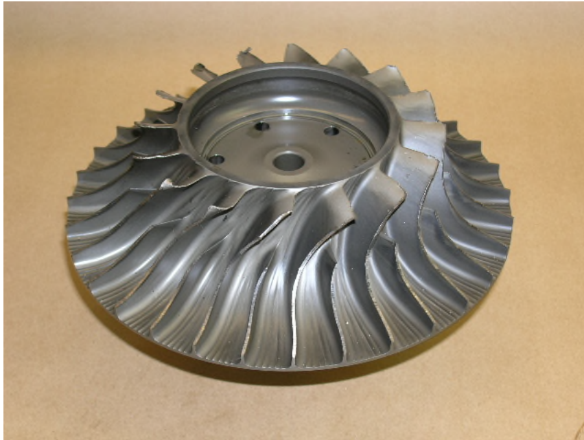
Photo No. 46 Centrifugal impeller.
