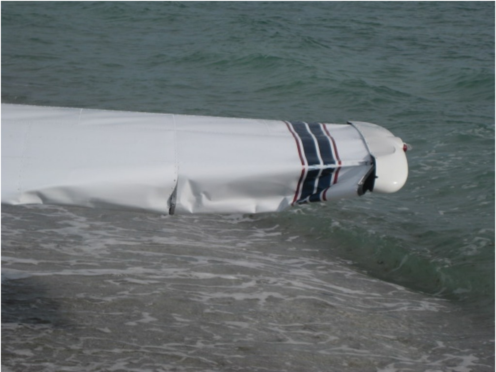
Photo 2 – Left Wing Leading Edge Damage (Courtesy FAA)
