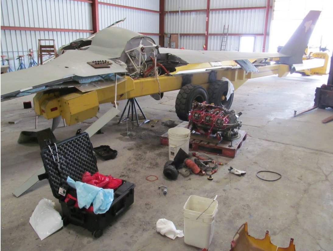
Photo 11: Engine as Left - Following Examination (Courtesy of Lycoming)
