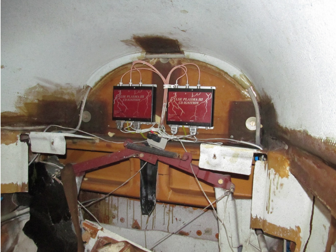
Photo 8: Dual Light Speed Ignition System as found - Post Recovery (Courtesy of Lycoming)
