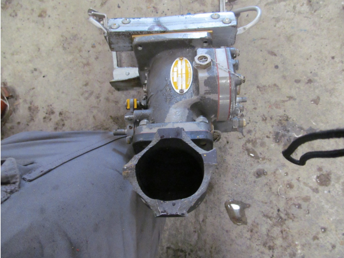
Photo 9: Fuel Injector Servo - Post Removal (Courtesy of Lycoming)
