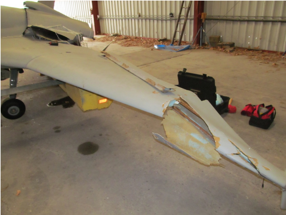
Photo 2: Damage to Left Wing - Post Recovery (Courtesy of Lycoming)
