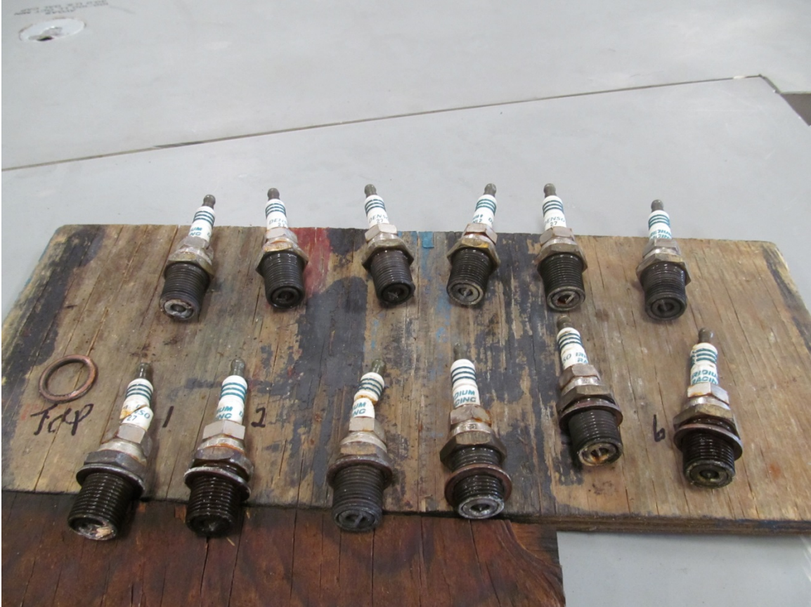
Photo 10: Spark Plugs - Post Removal (Courtesy of Lycoming)
