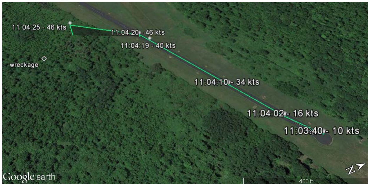
Figure 3. Aircraft take-off roll, flight, and wreckage location. Times and calculated true airspeeds are shown for each GPS point.
