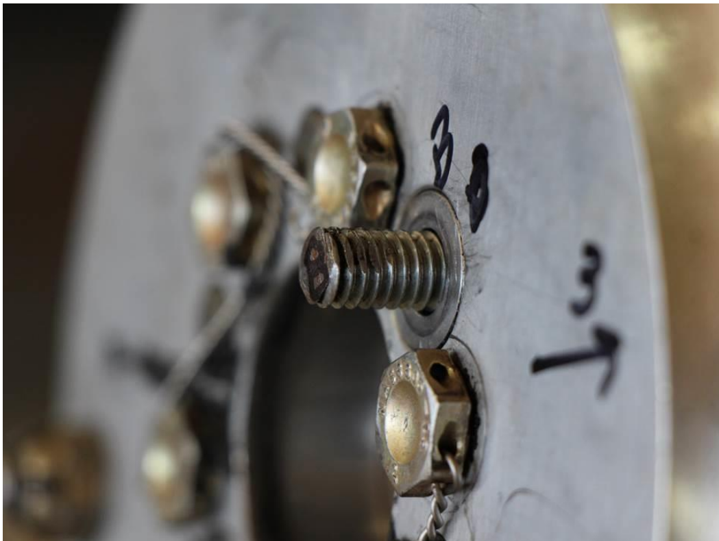
Photo 5 - Damage to the fine pitch adjusting bolt (B).
