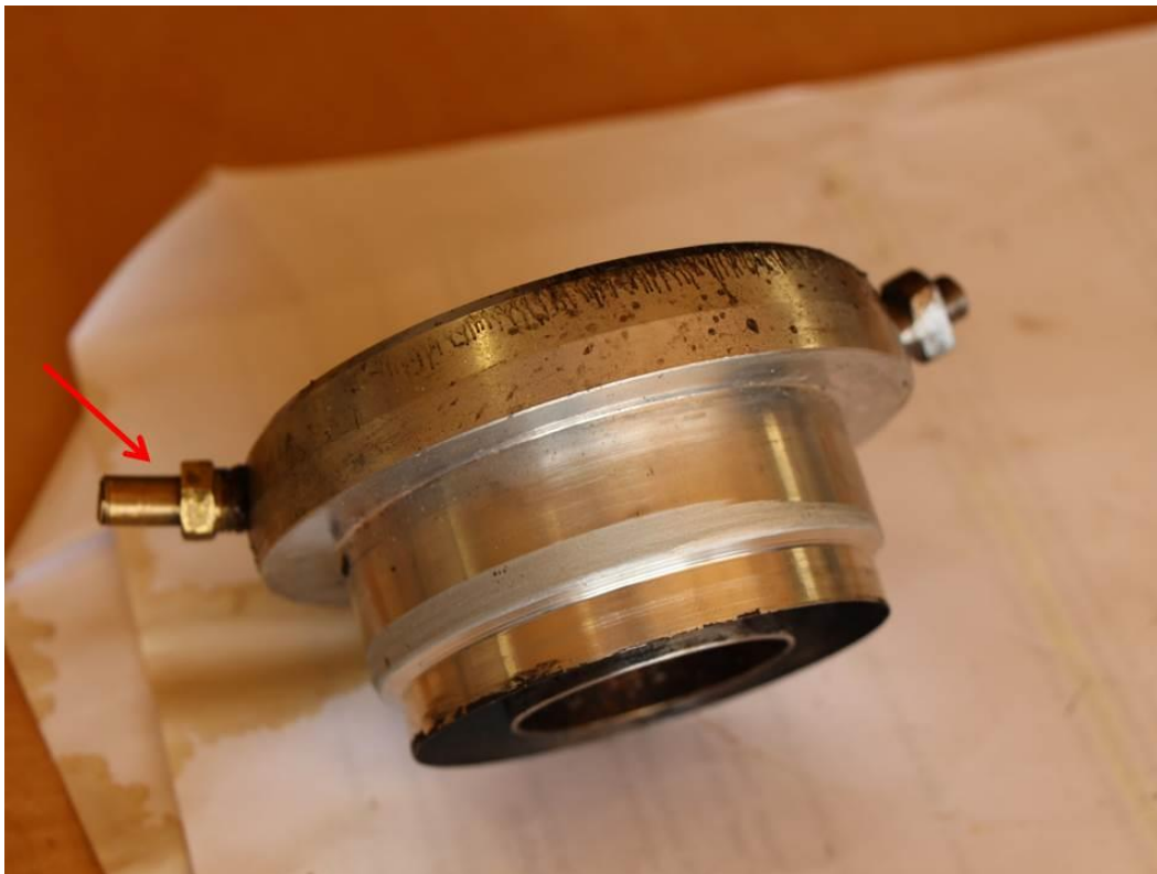
Photo 17 - The slave piston cup with hydraulic fittings.
