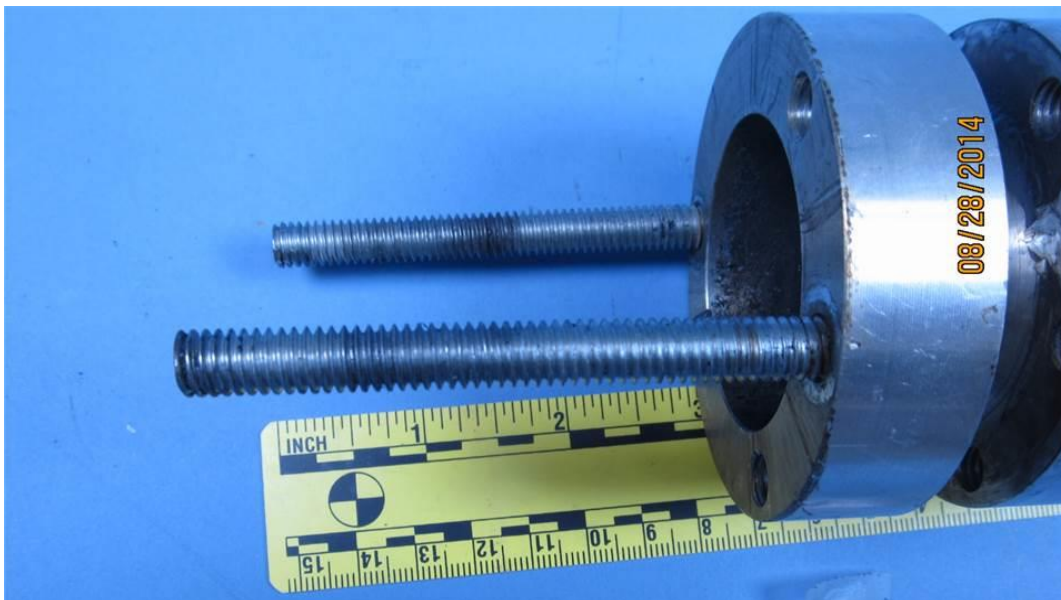
Photo 11 – Fine pitch adjusting bolts. Examination of the bolts did not disclose any evidence of damage or remnants that could be attributed to the elastic stop nut being present.
