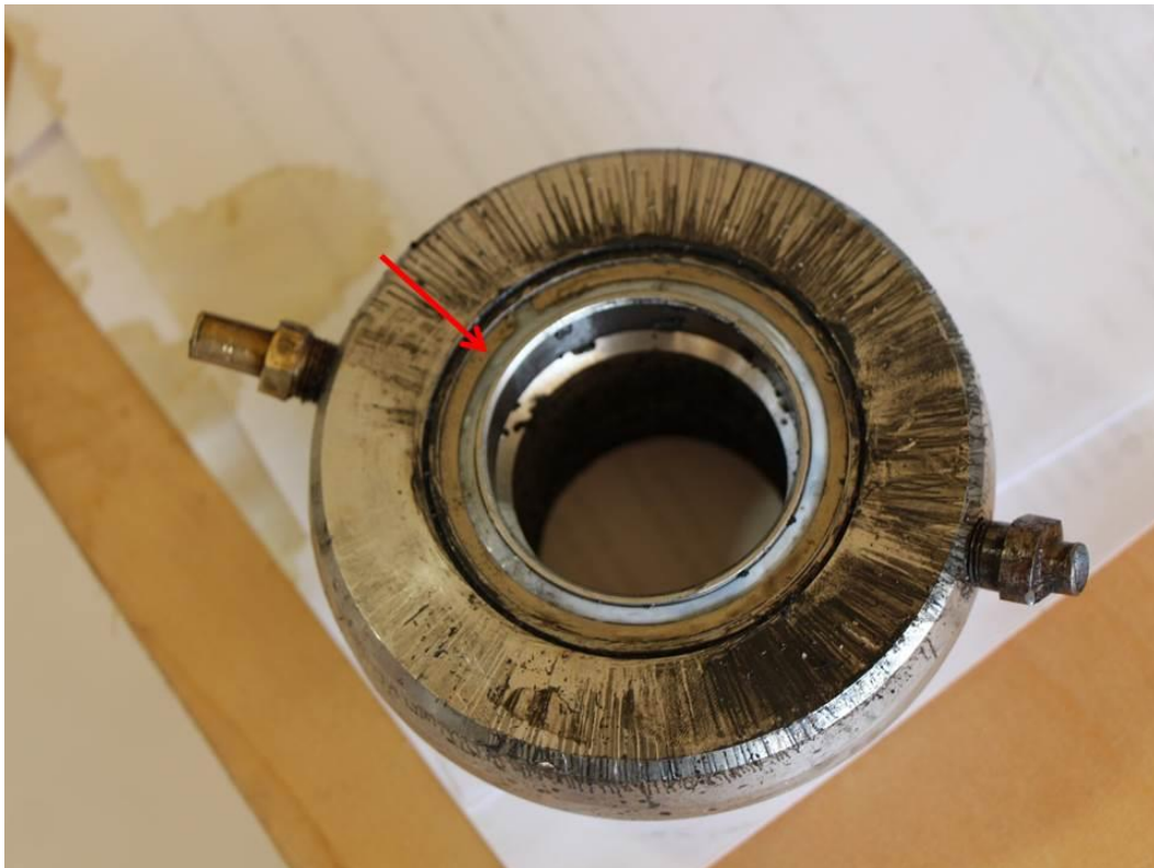
Photo 19 - The arrow points to the ball bearing snap ring on the slave servo.
