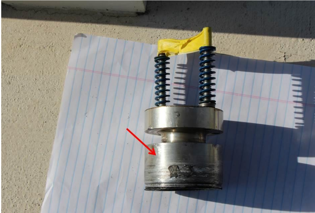
Photo 28 - The arrow points too galling damage to the side of the blade pin spool. The damage is consistent with damage to the inside of the slave piston collar. The blade pin spool should rotate while the slave piston collar remains stationary.
