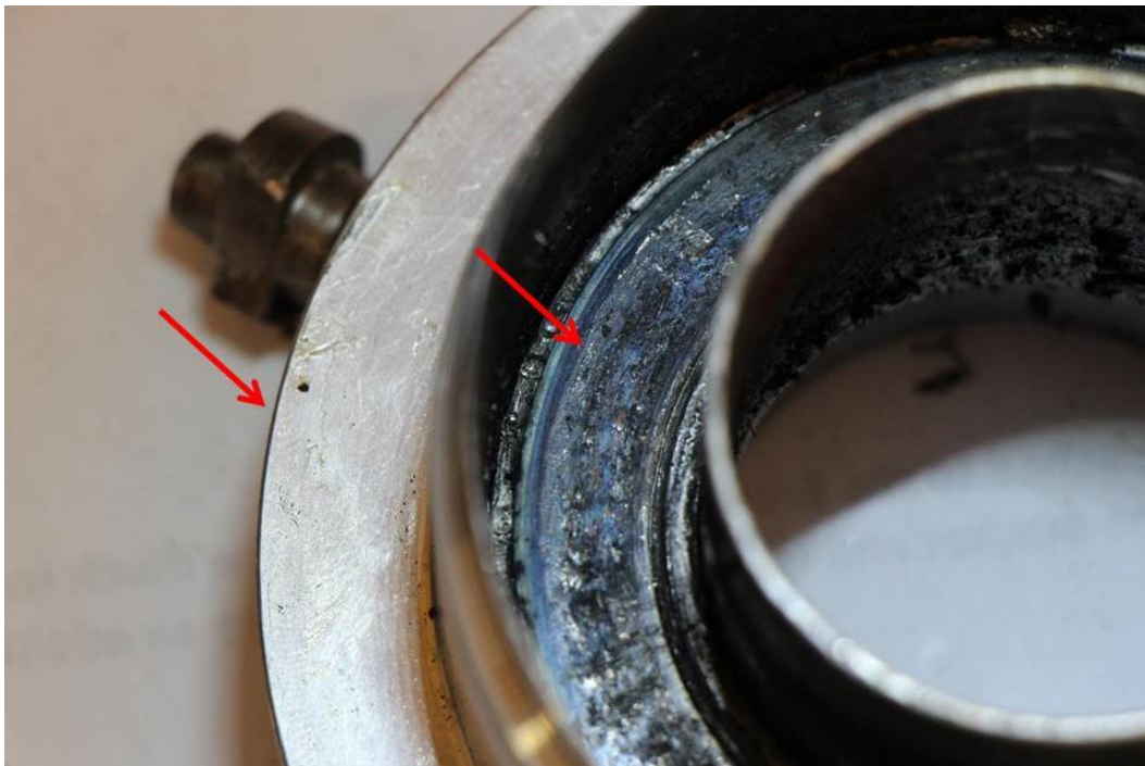
Photo 15 – The right arrow points to mechanical and heat damage at the slave piston collar bearing race that supports the needle thrust bearing. Grease was not present. The collar is still stuck to the slave piston cup (left arrow). The collar should be free to move fore and aft inside the slave piston and should not rotate relative to the slave piston. The blade pin spool rotates inside the slave piston collar.
