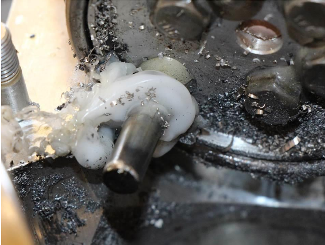
Photo 26 - Melted Delrin bushing and pitch change pin.
