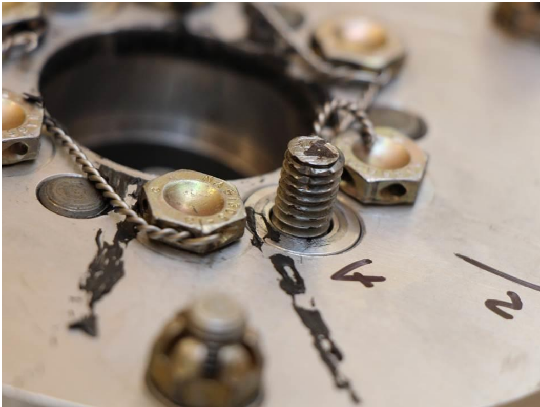
Photo 8 - Damage to the fin pitch adjusting bolt (A).
