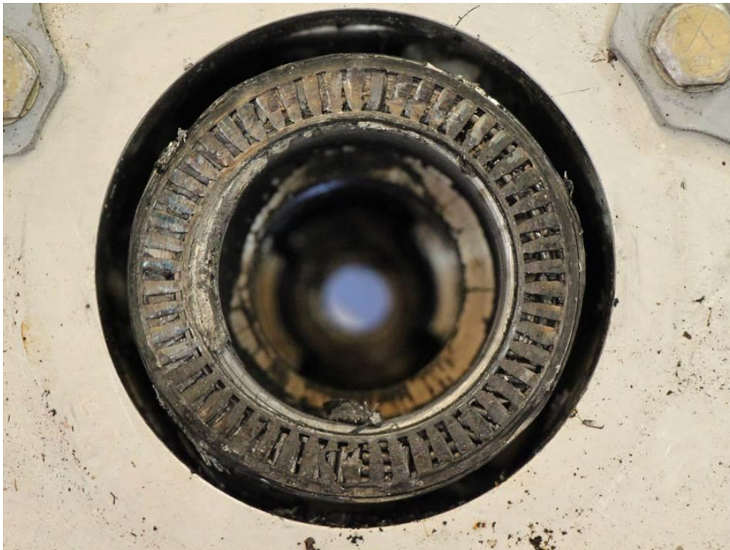
Photo 13 - Damage to the needle thrust bearing. Grease was not present. Many needle rollers were either mispositioned or loose. The examination disclosed that the needle rollers and the bearing race were damaged. All of the needle rollers had separated and were loose or displaced within the bearing. Severe heat damage was present in all parts near the needle thrust bearing.
