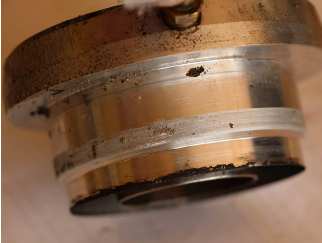
Photo 18 - Galling and heat damage on the slave piston cup.
