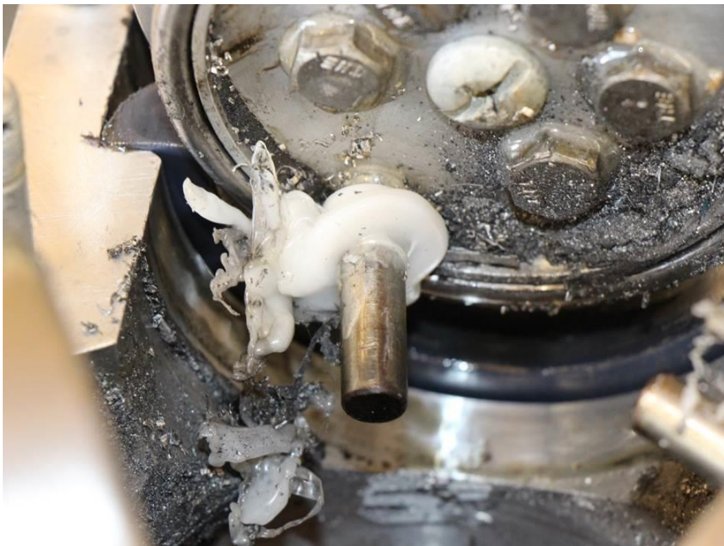
Photo 25- Melted Delrin bushing and bent pitch change pin.
