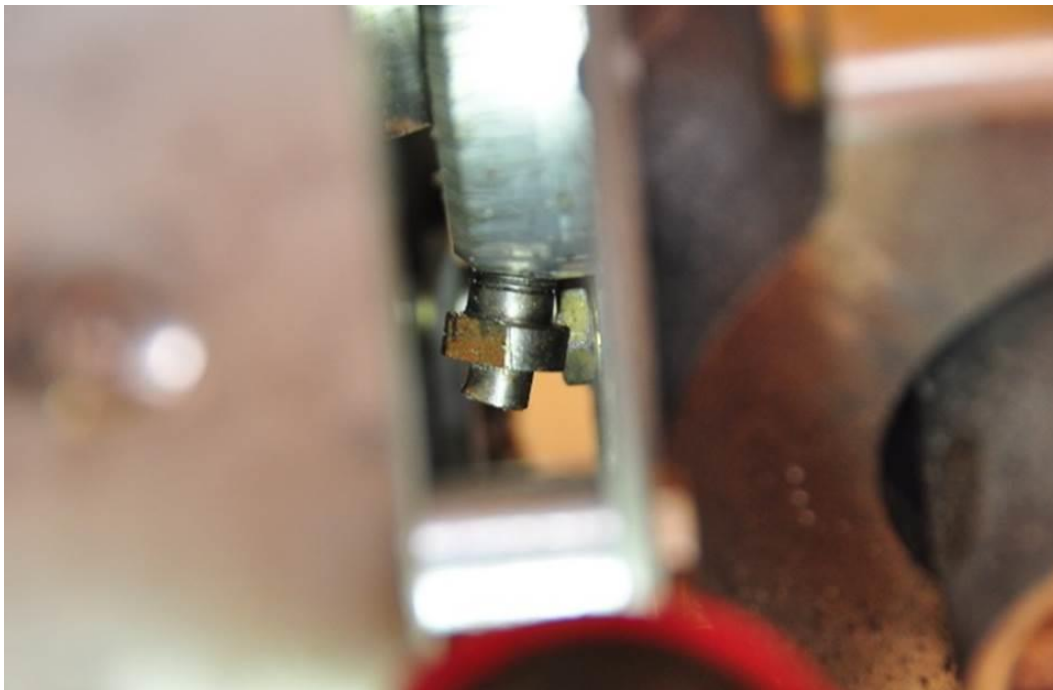
Photo 3 – The fractured hydraulic line fitting at the slave servo.
