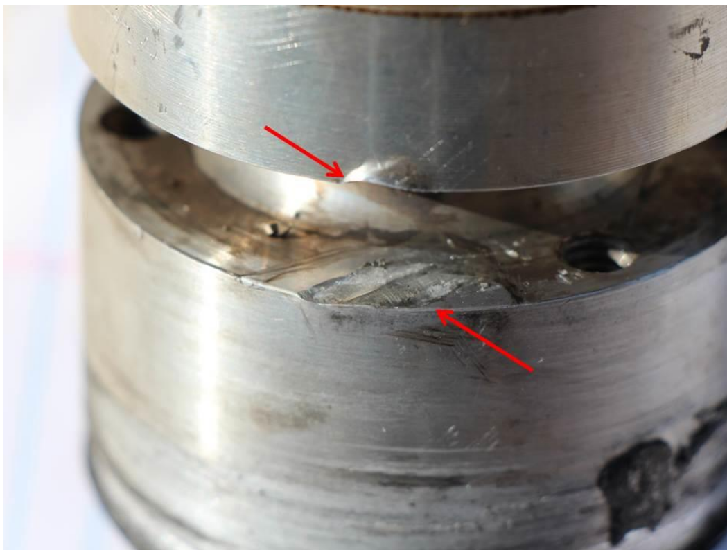
Photo 29 – Damage to the blade pin spool from the blade pitch change pins after the Delrin sleeve has melted.
