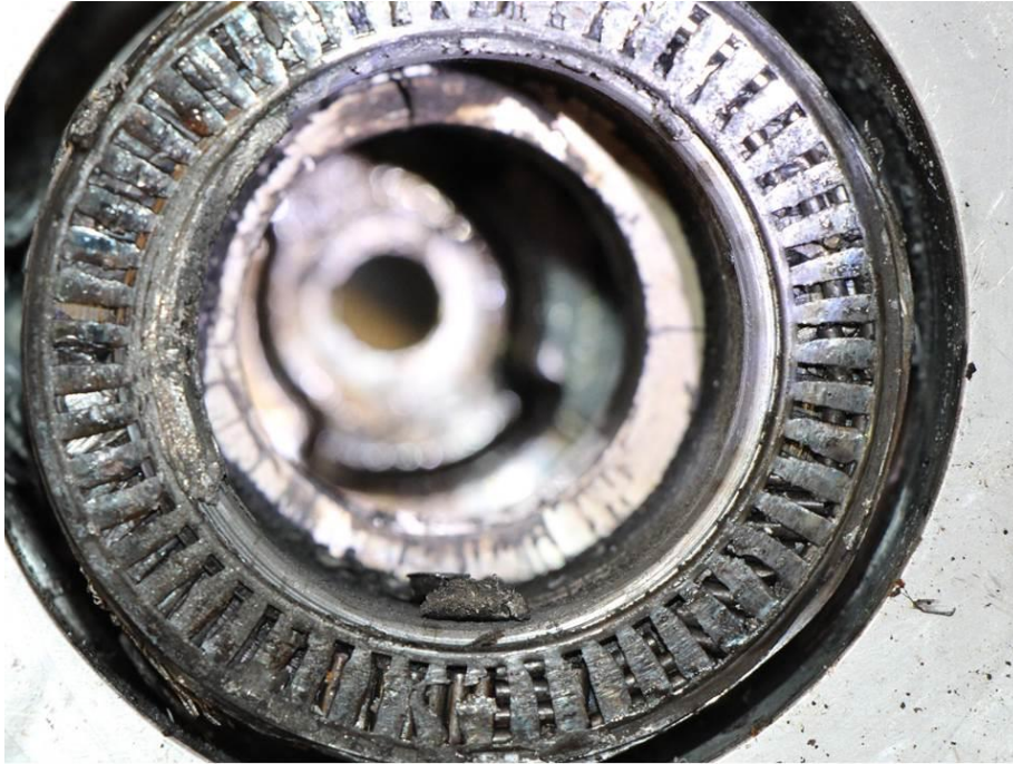
Photo 14 - Damage to the needle thrust bearing.
