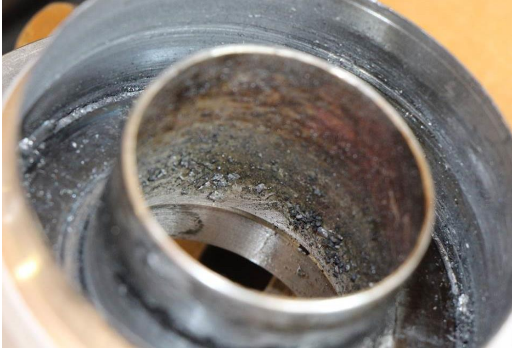
Photo 16 - Galling damage to the three visible walls of the slave piston collar. The galling at the inner core is adjacent to the propeller drive shaft. The galling in the race area is adjacent to the blade pin spool and needle thrust bearing.
