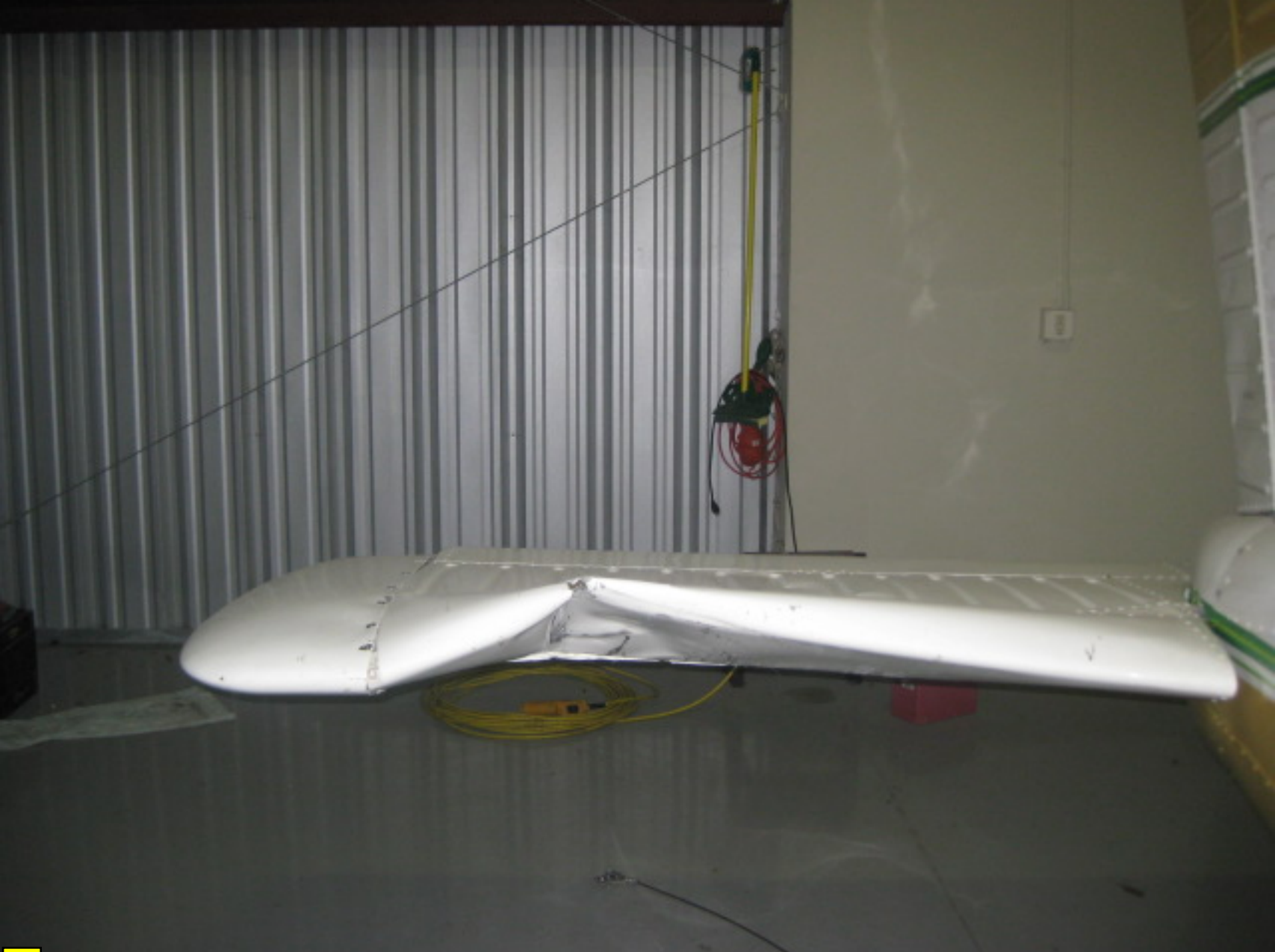
Photo 1 – View of Damage to Horizontal Stabilizer (Photo Courtesy of FAA)
