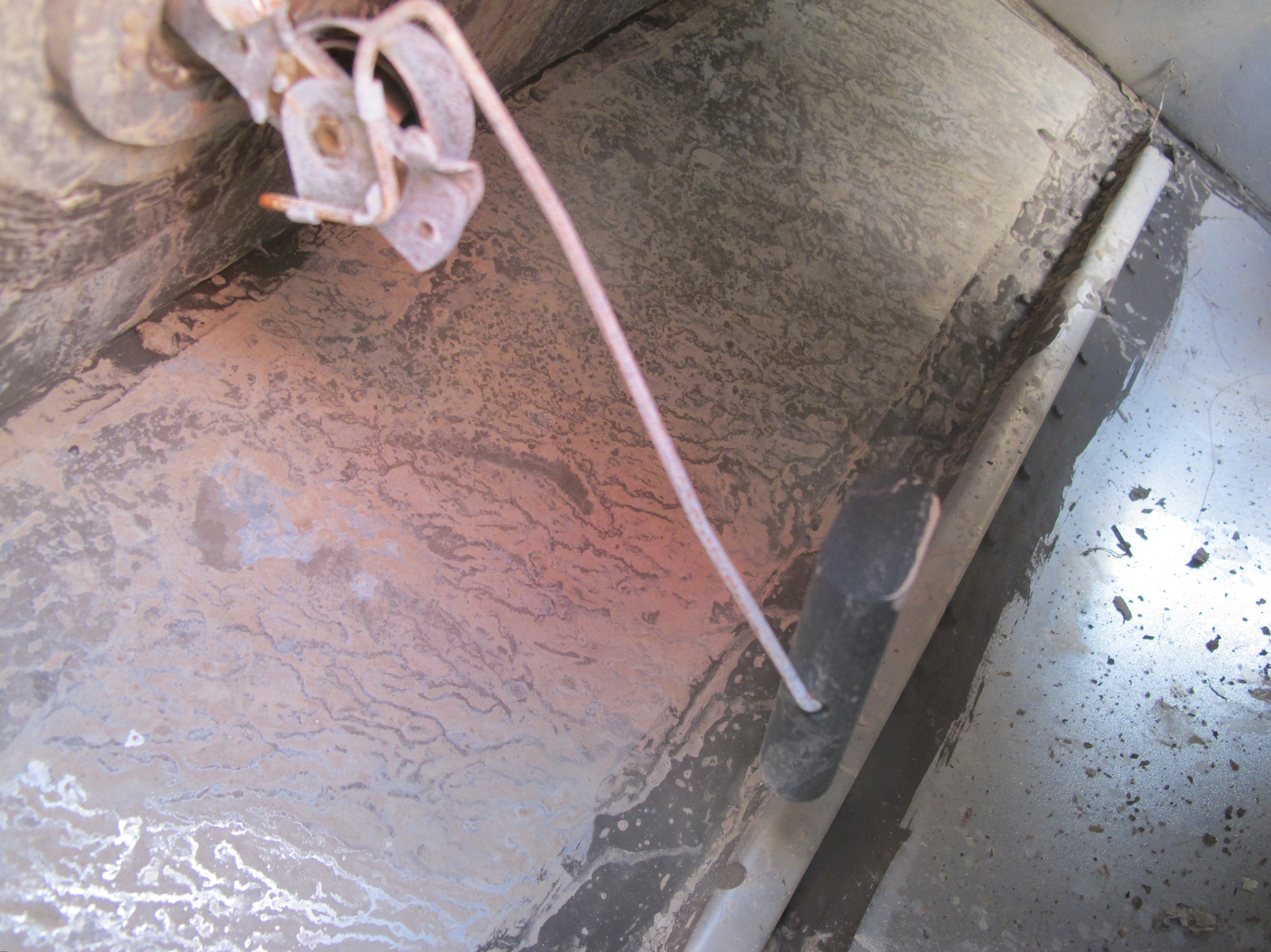
Photo 5 - Left Fuel Quantity Indicating Sensor (Photo Courtesy of Piper)
