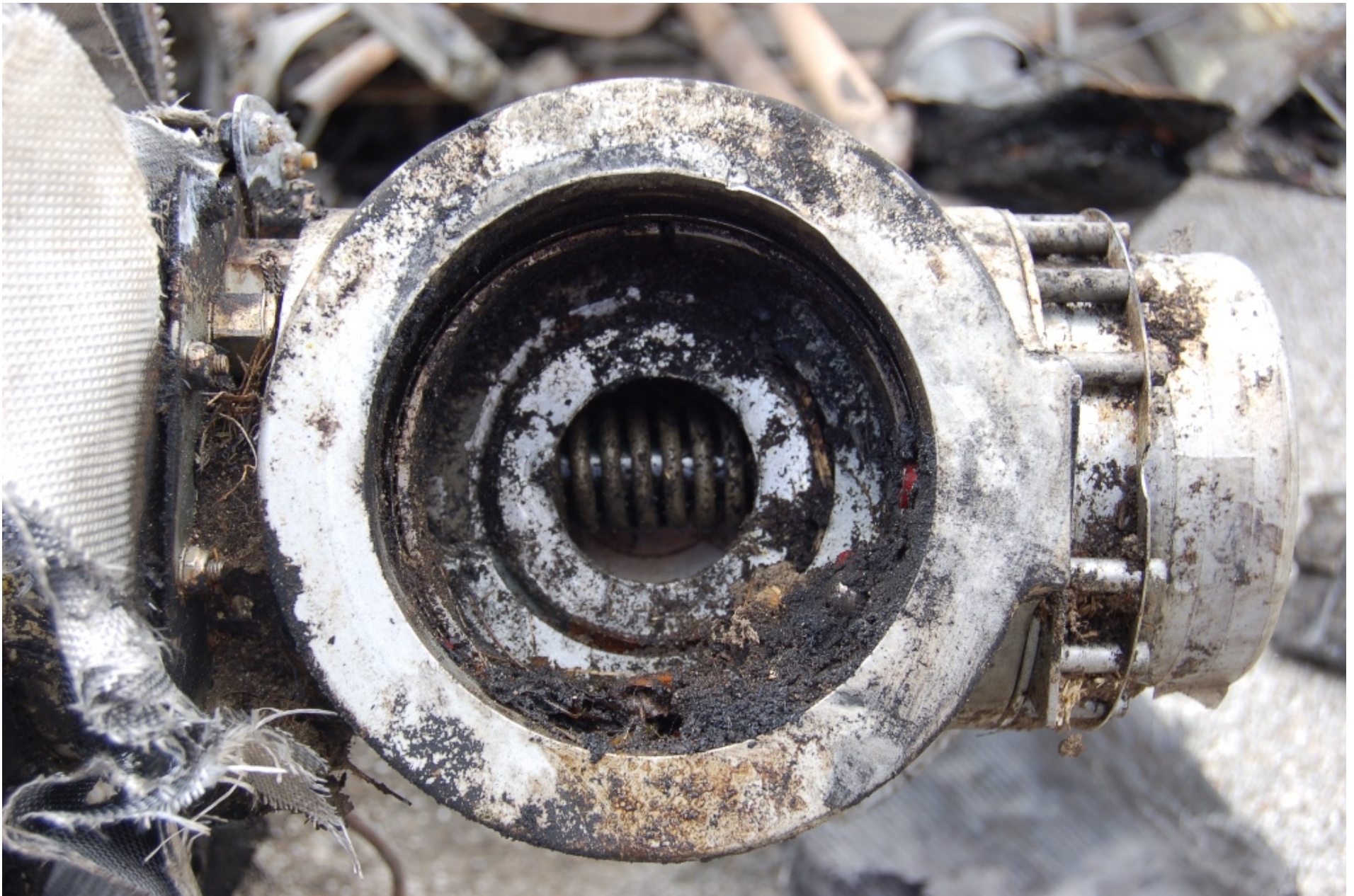
Photo 6 – Close Up of Propeller Hub Showing Fractured Blade Root – Courtesy of FAA
