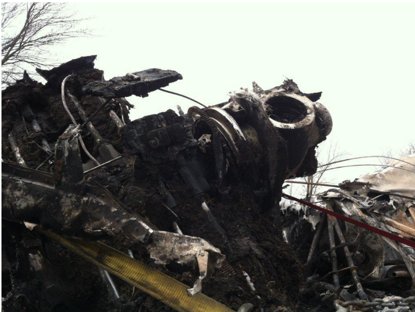
Photo 5 – Propeller Hub with Blade Missing – Courtesy of FAA
