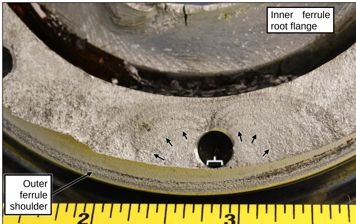
Figure 4. Blade 1 fracture surface (upper image) with a closer view of the fatigue origin area (lower image) after removal from the hub and cleaning with a degreasing solution. In the upper image, unlabeled arrows indicate the extent of crack propagation from the primary origin area as indicated with a bracket in the lower image. Dashed lines indicate the extent of cracking from secondary fatigue cracks. Unlabeled arrows in the lower image indicate the crack propagation direction in the vicinity of the bolt hole.
