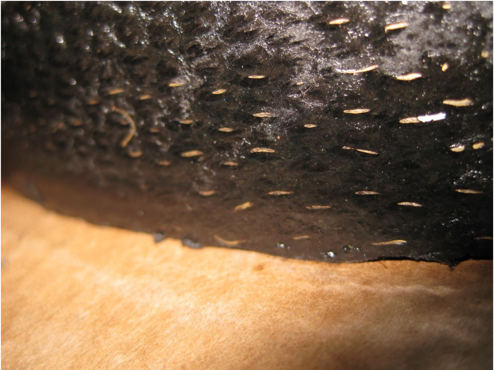
Photo 6 – Close Up Photograph of Clutch Pad – Courtesy of FAA
