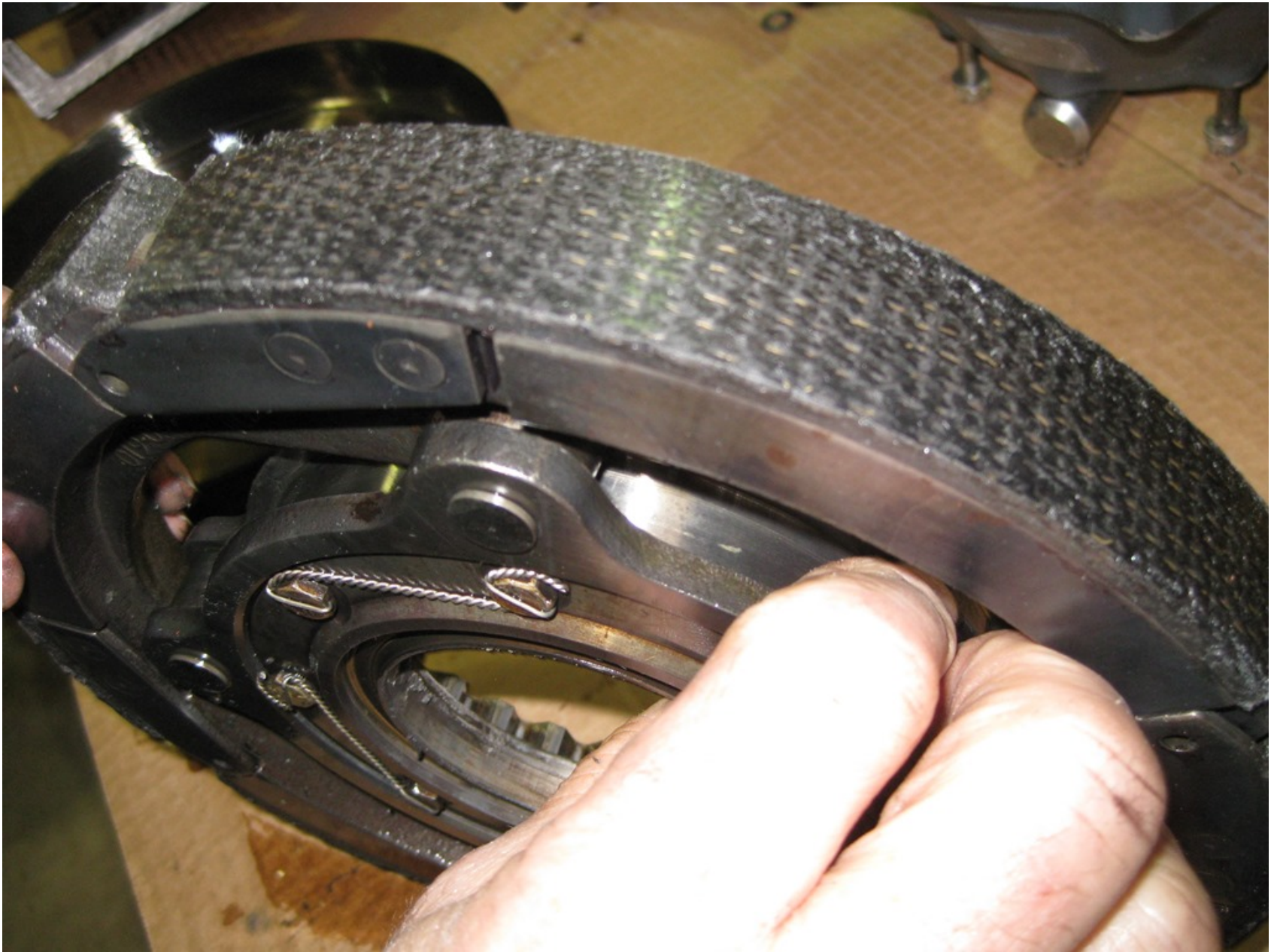
Photo 5 – Glazed Clutch Pads – Courtesy of FAA
