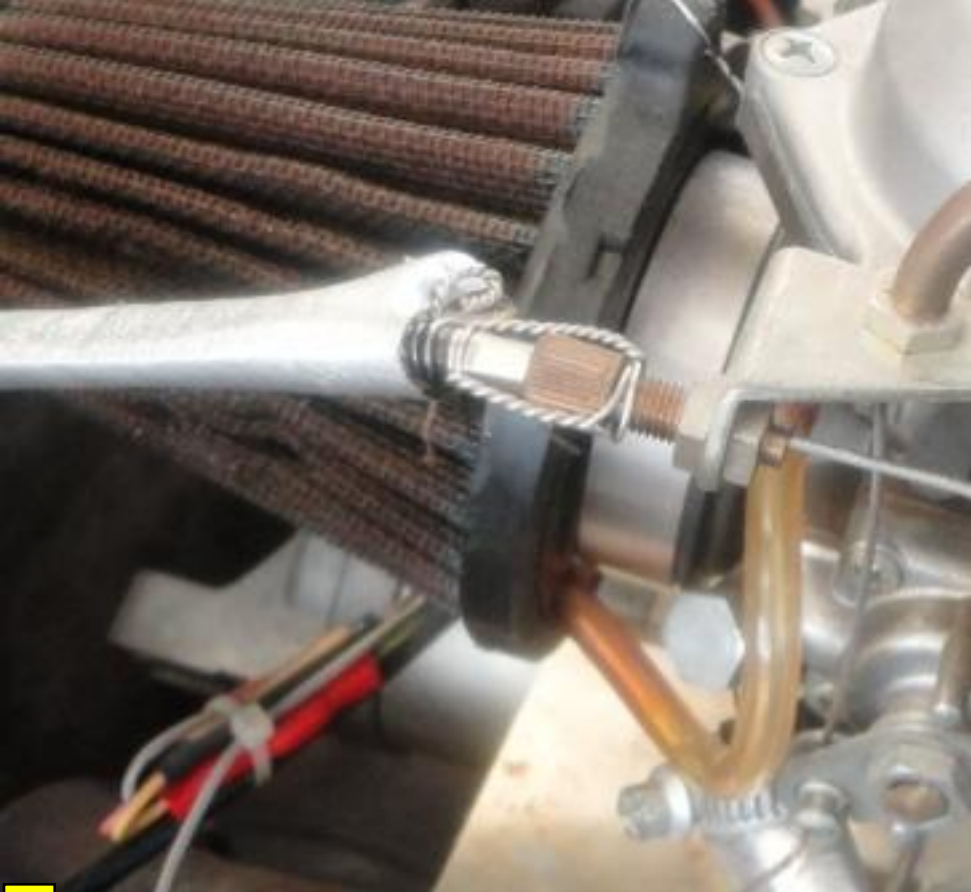
Photo 3 – Vent Line Routing as Found (Courtesy of Rotax)
