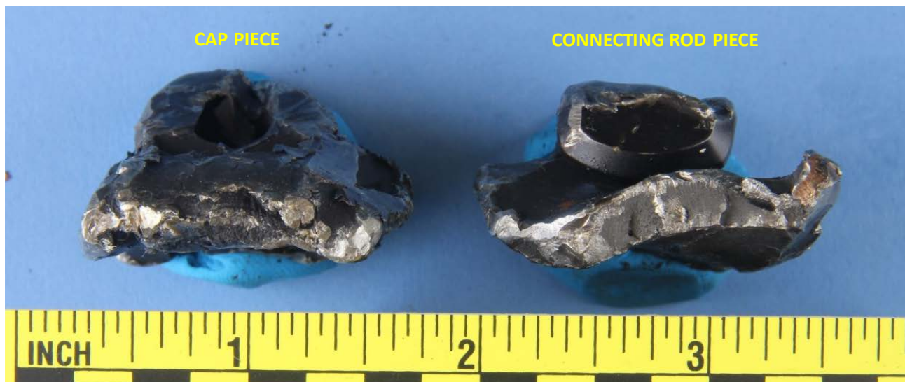
Figure 2: Close-up photos of the fracture surfaces on the connecting rod and cap pieces shown in the top of Figure 1.
