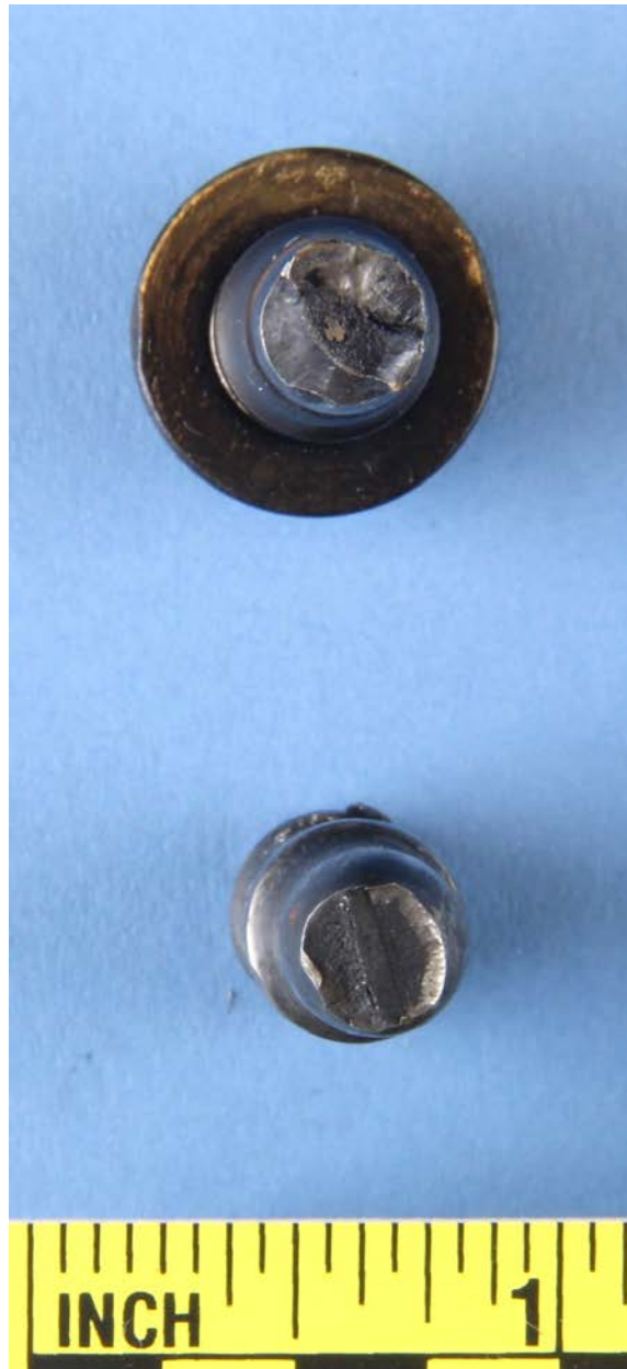
Figure 5: Close-up photo of the fracture surfaces on the bolt pieces with the threaded ends.
