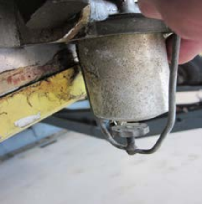
Photo 4: View of gascolator with no safety e (Photo Courtesy of FAA)
