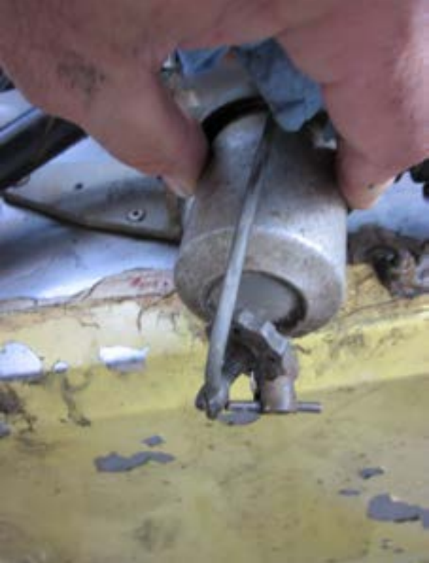
Photo 3- View of gascolator held in place (Photo Courtesy of FAA)
