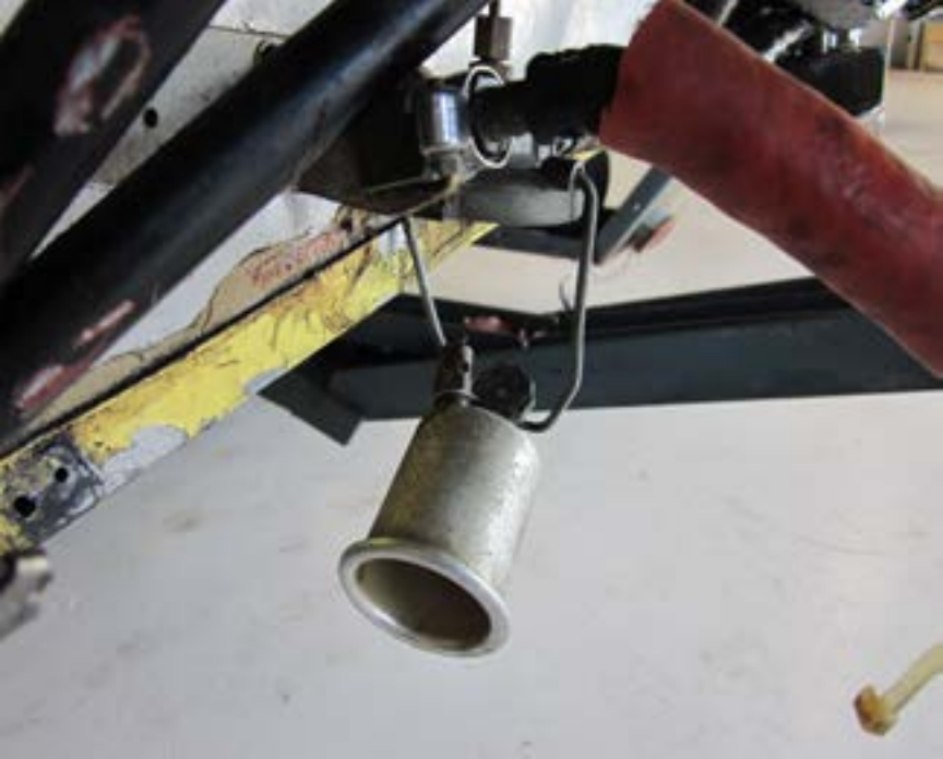
Photo 2 – View of hanging gascolator (Photo Courtesy of A)
